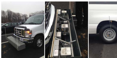
Inertial profilometer vehicle (left), sensor bar with cover open (center), and distance measurement instrument (right).
