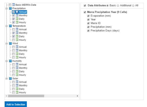
Selected MERRA data can be submitted for data extraction using the existing LTPP InfoPave Data Bucket for the selected MERRA cells.
