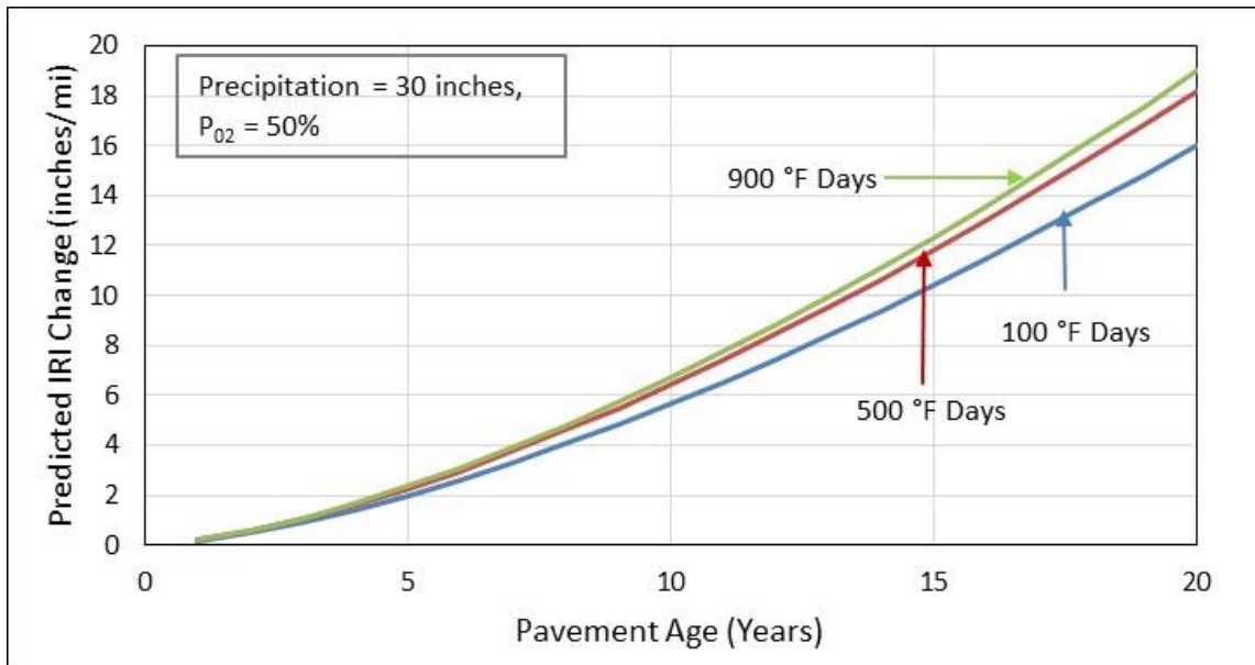
Figure 11. Graph. Change in IRI by fixing average annual precipitation and P_{02} and varying average annual FI.
