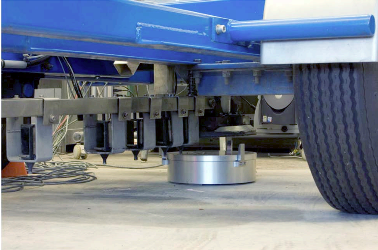
Figure 106. Photo. Reference load cell positioned under the FWD load plate.
