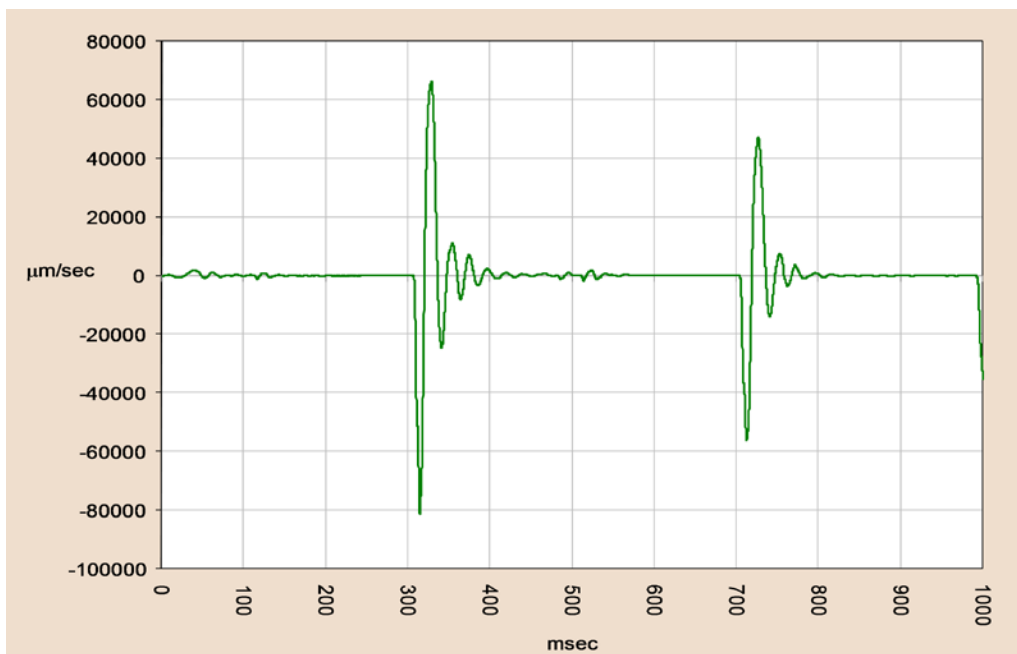
Figure 19. Graph. First integration (velocity) from a Dynatest® FWD impulse.
