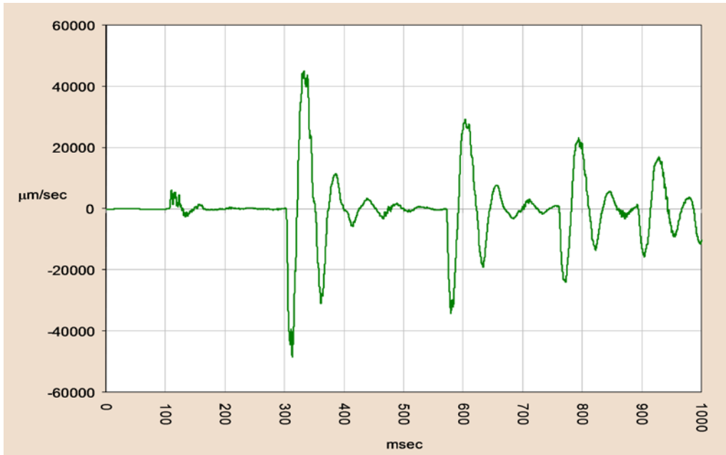
Figure 22. Graph. First integration (velocity) from a JILS FWD impulse.
