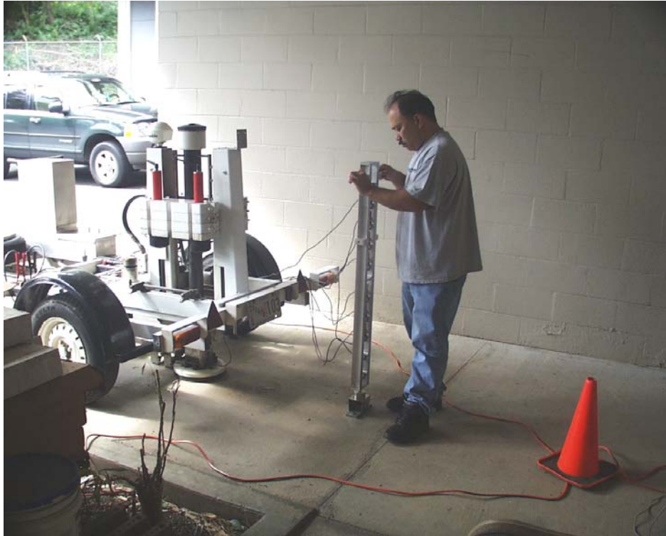
Figure 38. Photo. On-site FWD calibration at Hawaii Department of Transportation Materials Lab.
