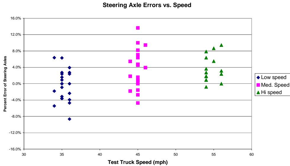
Figure 3-5 Post-Validation Steering Axle Percent Error vs. Speed Group - 120500 – 03 Mar 2005
