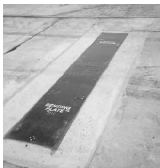
Figure 25 - Bending Plate scales
