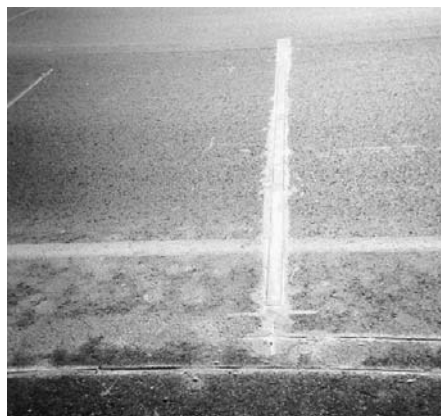
Figure 26 - Piezo Class I sensor
