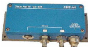
Kistler Type 5038A2Y43 charge amplifier for two channels.
