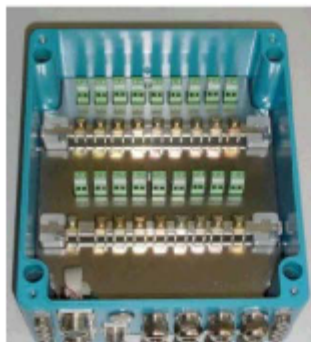
Kistler Charge Amplifier 5153A... for 9 or 18 channels
