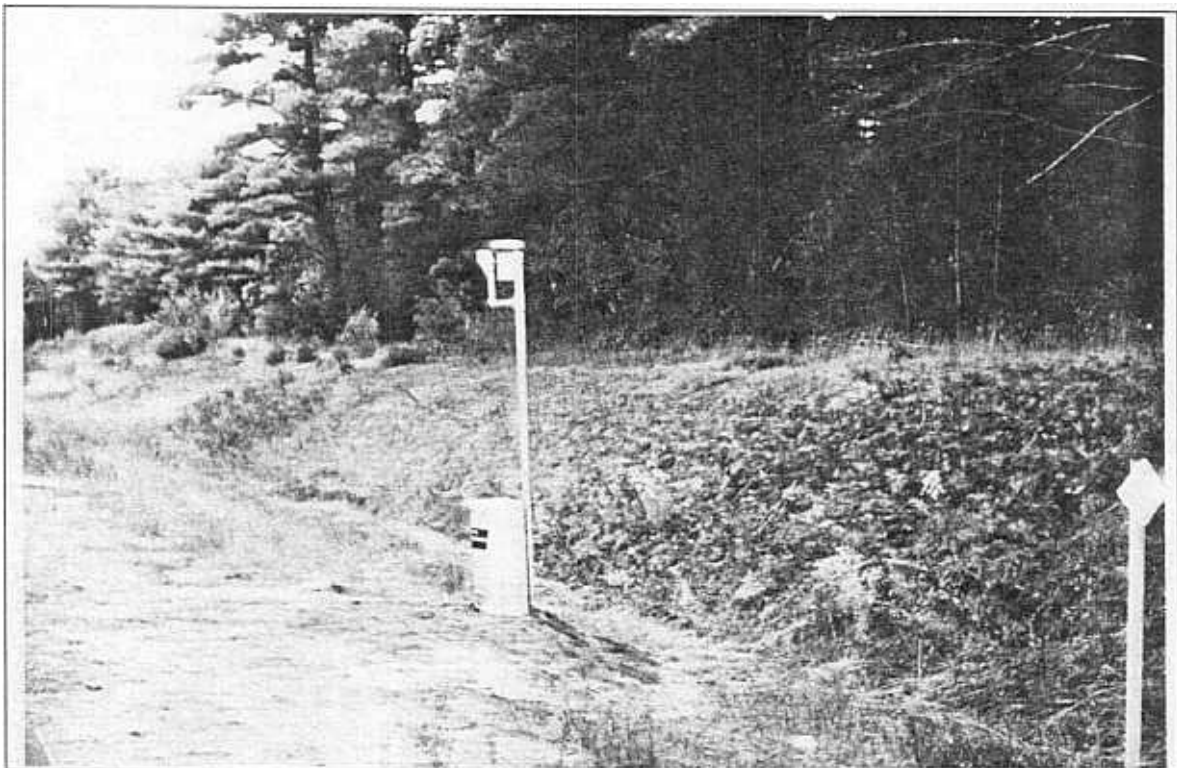
Figure E-3. Equipment Cabinet, Air Temperature Probe, and Rain Gage
