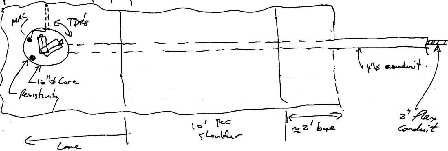
while H-hole in final approach the cables were pulled to the far side of the hole. and the hole for the temperature probe was drilled. Angle for drill was laid out on a piece of plywood to get drill @ proper angle.
