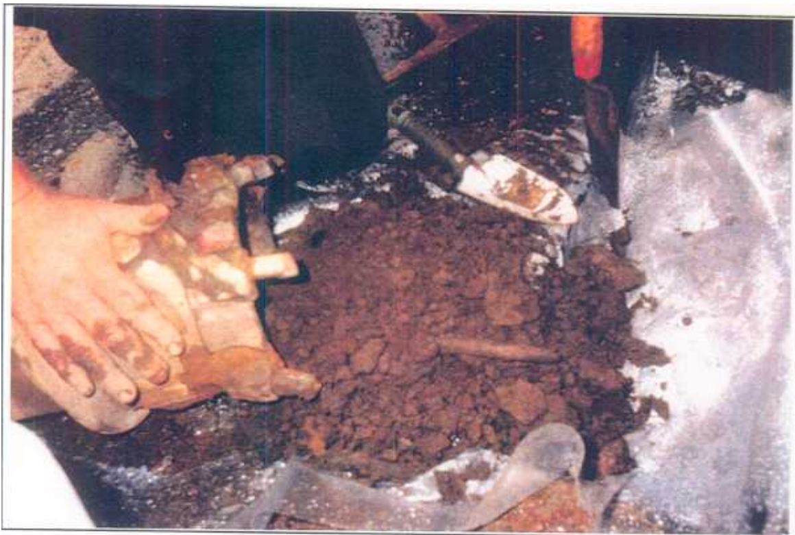
Figure E-4. Material Sampled From Instrumentation Hole For Moisture Determination
