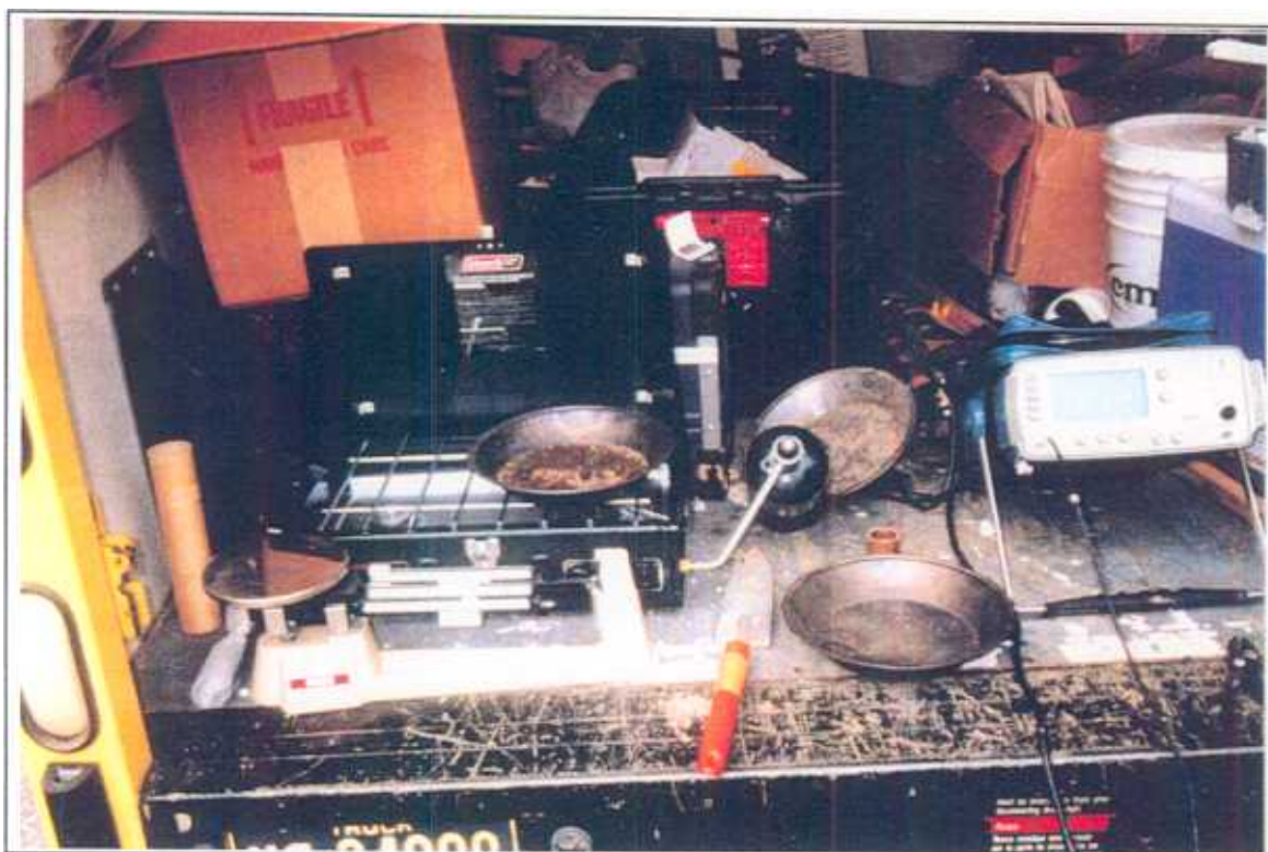
Figure E-5. Material Sampled From Instrumentation Hole For Moisture Determination
