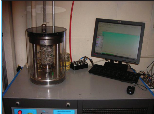
Figure 1. Dynamic Modulus Test Setup in the Asphalt Mixture Performance Tester.
