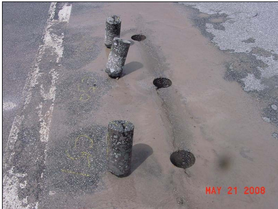
Figure F-12: 100mm Cores at Low Severity Longitudinal Crack in Wheel Path (360802)
