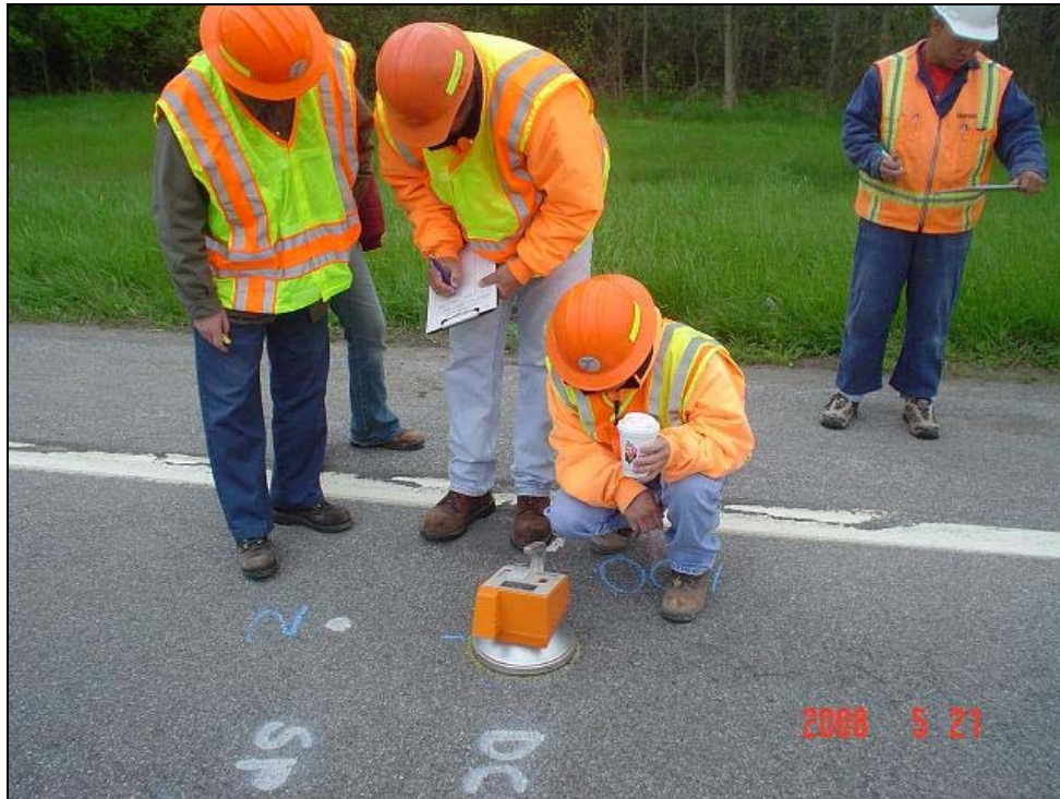
Figure E-13: Pavement Quality Indicator (PQI) Density Data Collection
