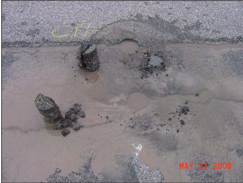
Figure F-5: 100mm Cores at Multiple Inner Wheel Path Longitudinal with Associated Cracking (360801)
