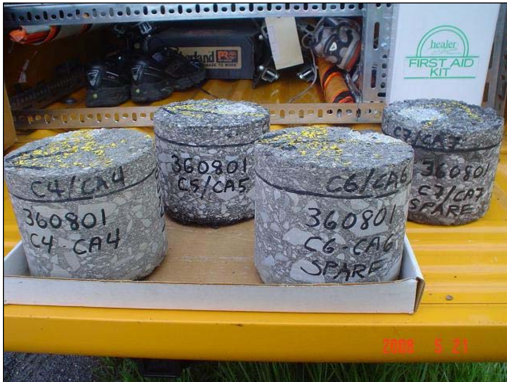
Figure F-13: 150mm Cores at Station 1+00 (360801)
