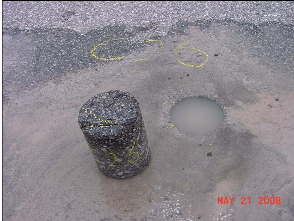
Figure F-7: 100mm Core at Low Severity Longitudinal Crack in Midlane (360801)
