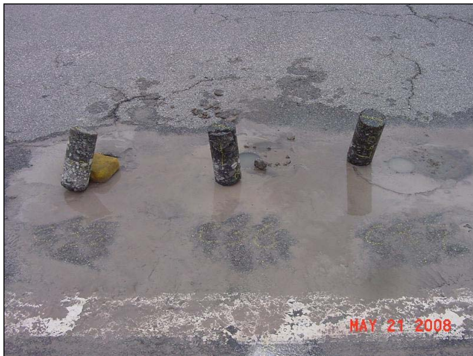
Figure F-10: 100mm Cores at Location of Wheel Path Longitudinal and Associated Cracking (360802)
