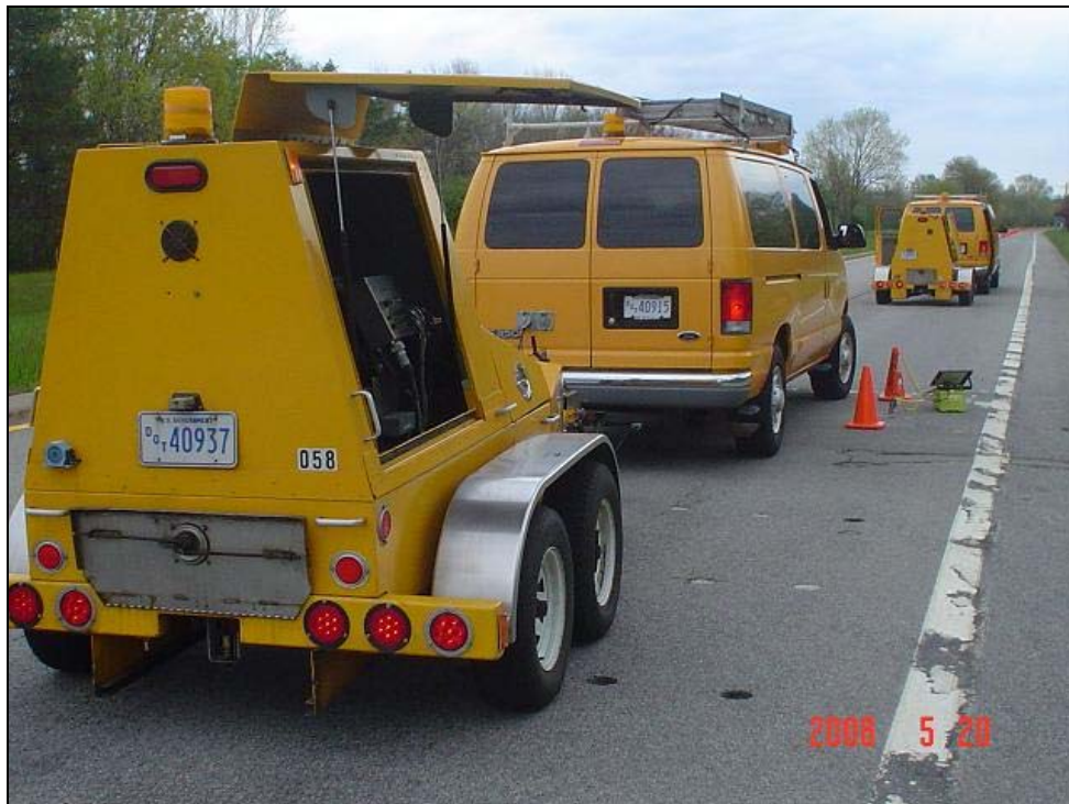
Figure E-14: Falling Weight Deflectometer (FWD) Data Collection
