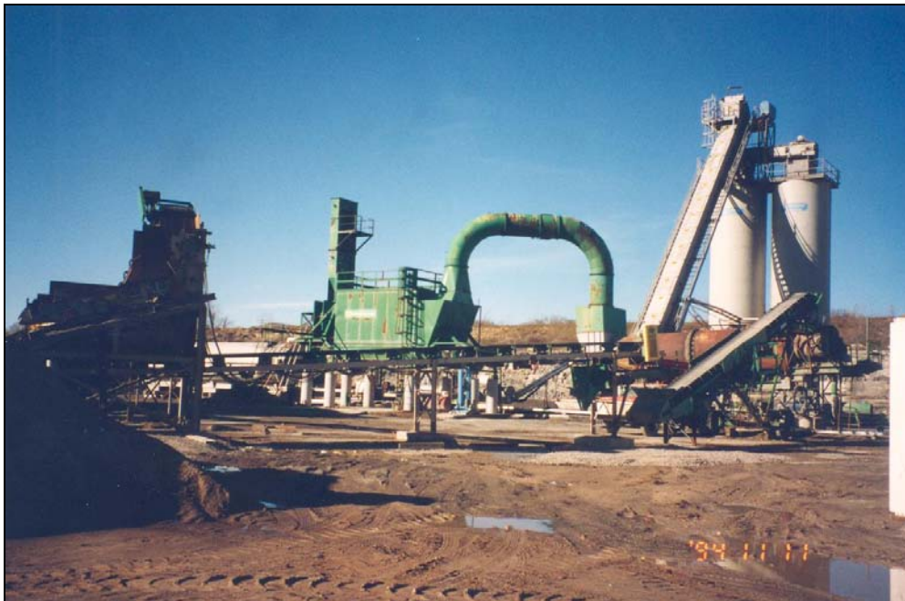
Figure D-8: Asphalt Batch Plant - Genesee LeRoy Stone Corp., Stafford, NY
