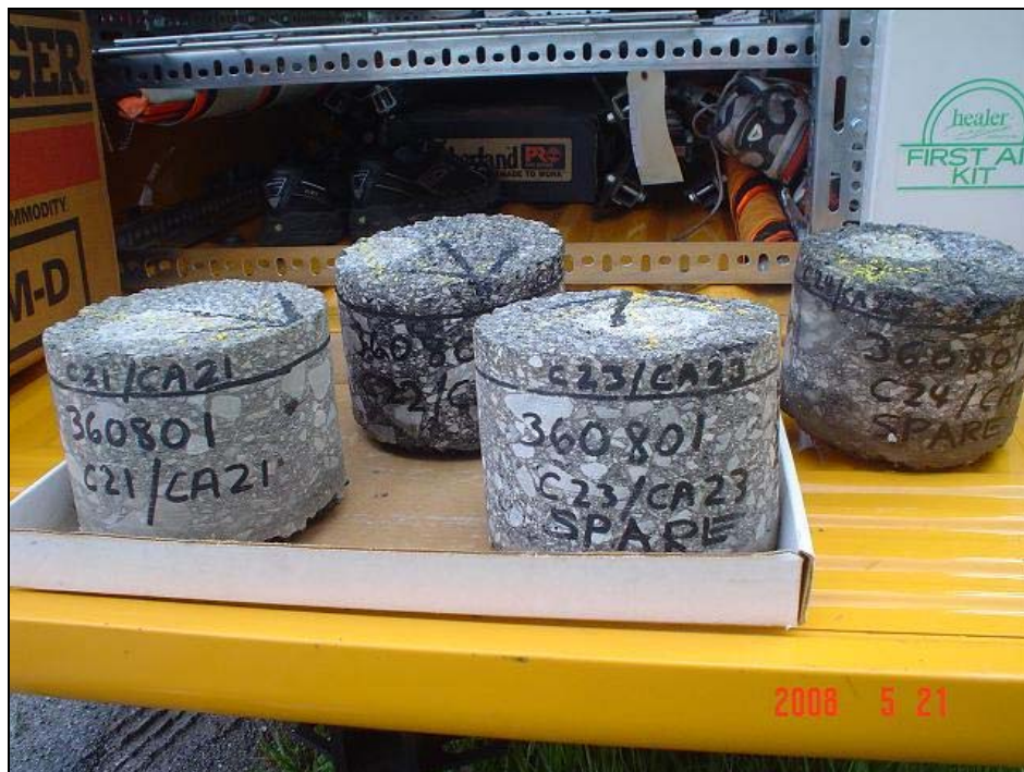
Figure F-14: 150mm Cores at Station 3+50 (360801)
