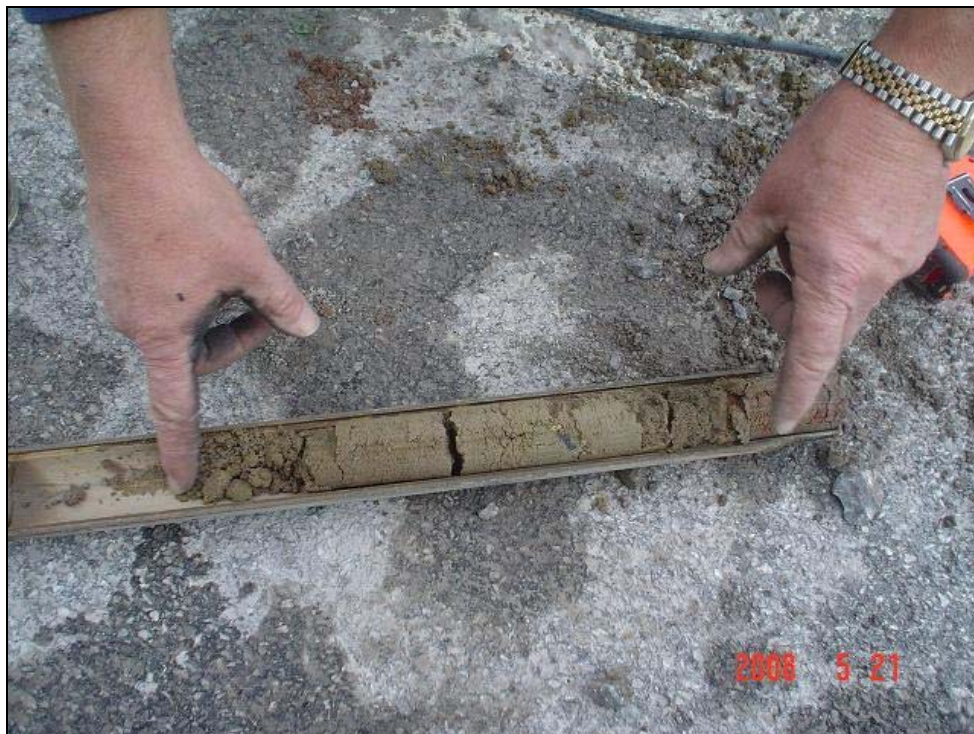
Figure G-2: Split-Spoon Sample Material
