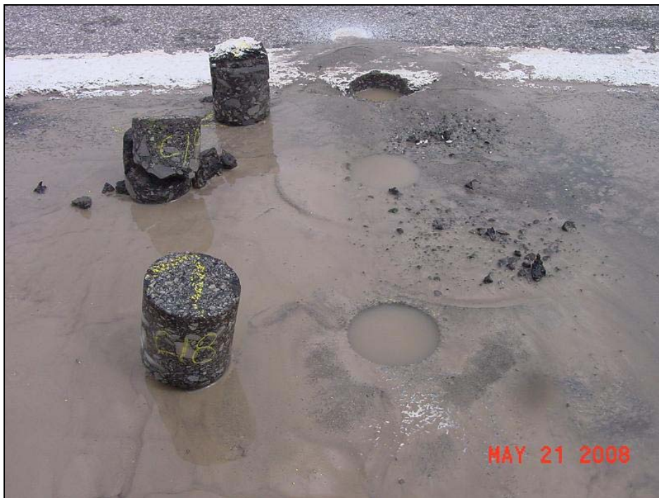
Figure F-6: 100mm Cores at Alligator Cracking from Centerline towards Inner Wheel Path (360801)
