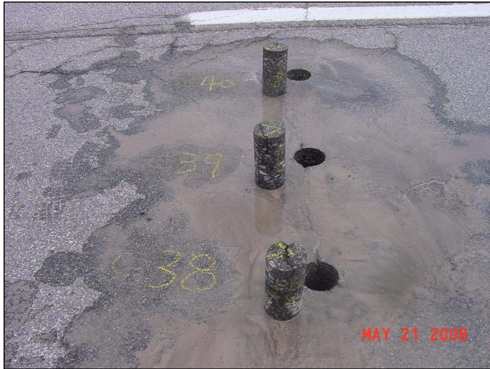
Figure F-11: 100mm Cores at Transverse Crack (360802)
