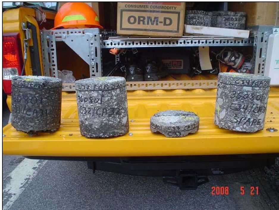
Figure F-15: 150mm Cores at Station 5+00 (360801)
