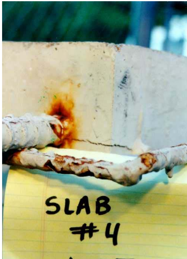
Figure 12. Photo. Rust staining and cracking on the side of slab 4.
