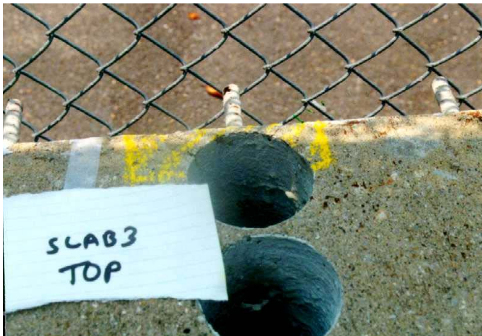
Figure 13. Photo. Delamination (marked in yellow) found on the top surface of slab 3.
