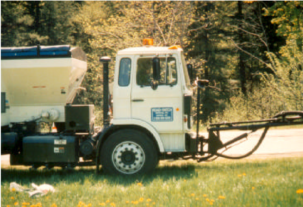
Figure 8. Spray-injection device—self-contained unit.
