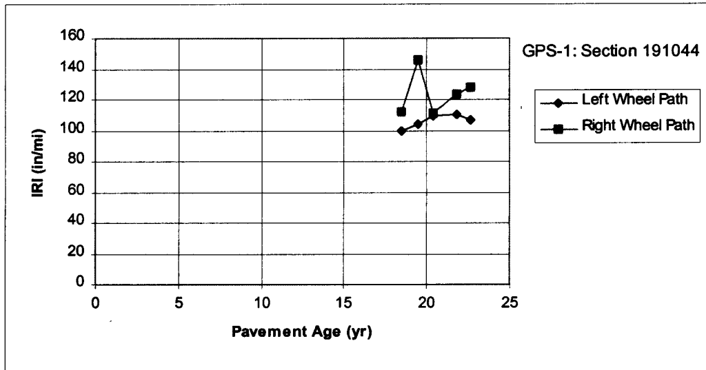
Figure 2.2.12. Section with inconsistent IRI values caused by variations in the profiled path.
