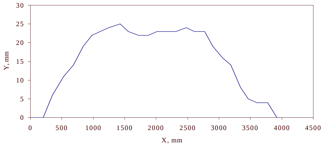
Figure 29. Typical profile providing a negative rut depth from five-point analysis.
