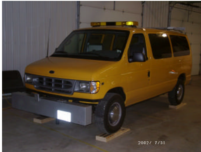
Figure 2.5.4.2. Profiler on top of support blocks.
