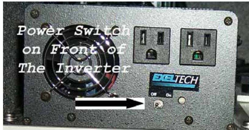
Figure 8. Photo. Inverter switch.
