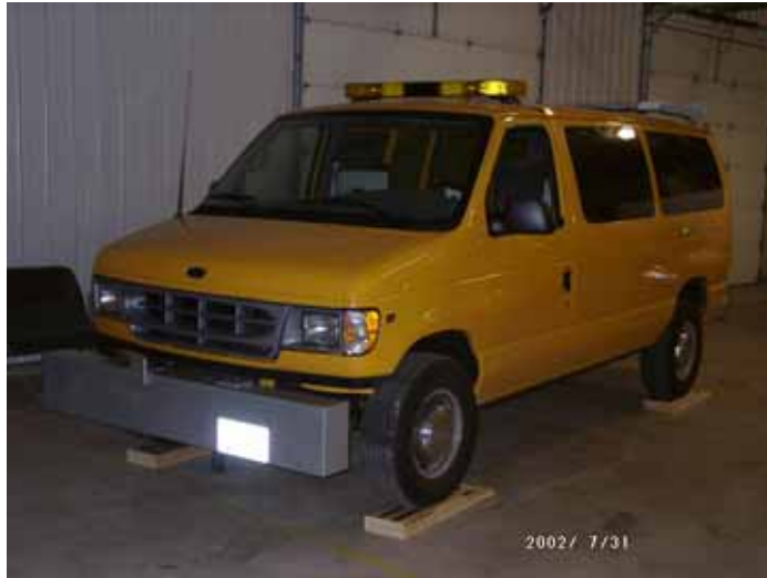
Figure 71. Photo. Profiler on top of support blocks.
