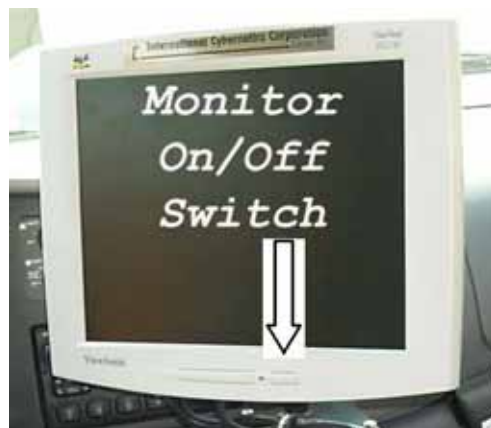
Figure 11. Photo. Monitor on/off switch.
