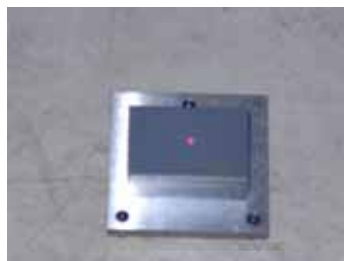
Figure 35. Photo. Block on top of base plate with calibration plate on top of block (1).
