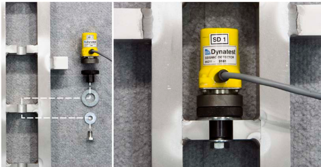
Figure 33. Photo. Attachment of a Dynatest ® geophone in the stand.
