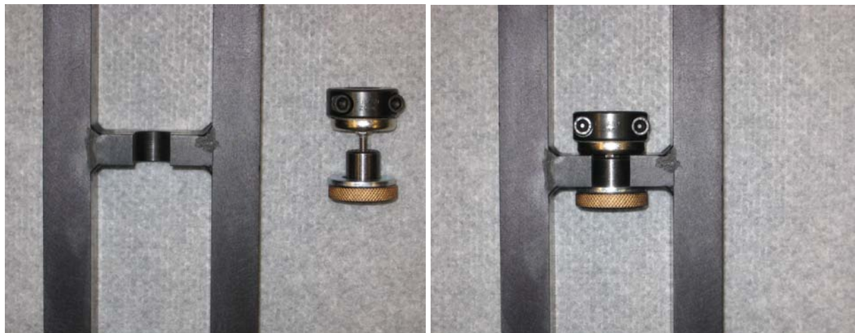
Figure 123. Photo. Attachment of a KUAB geophone adapter.
