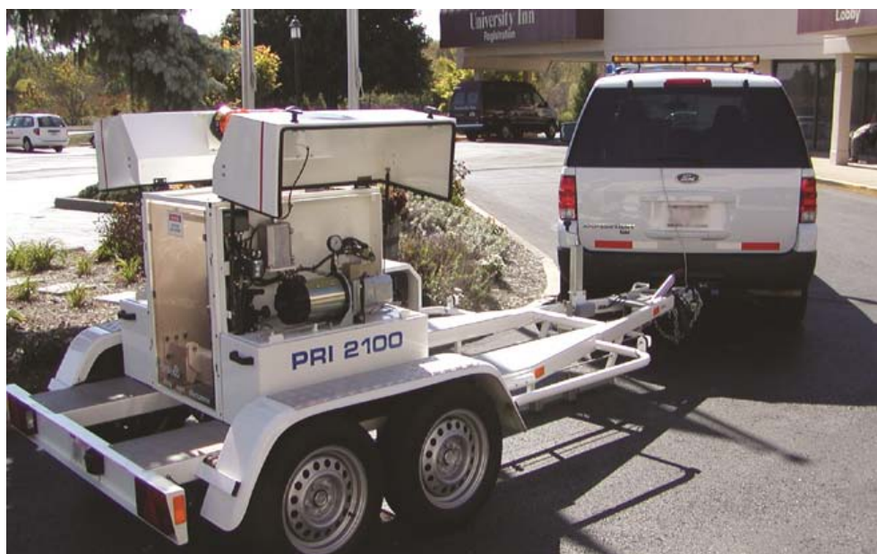
Figure 8. Photo. Carl Bro FWD.
