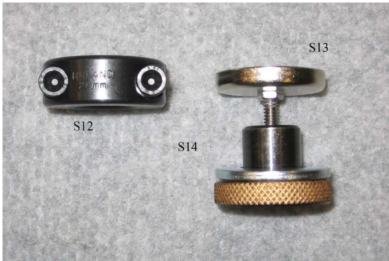
Figure 122. Photo. KUAB geophone adapter equipment.
