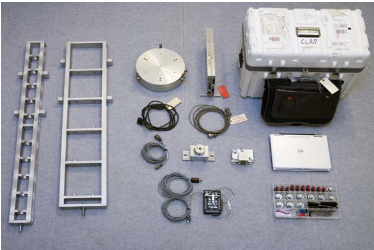
Figure 4. Photo. Calibration system hardware set.
