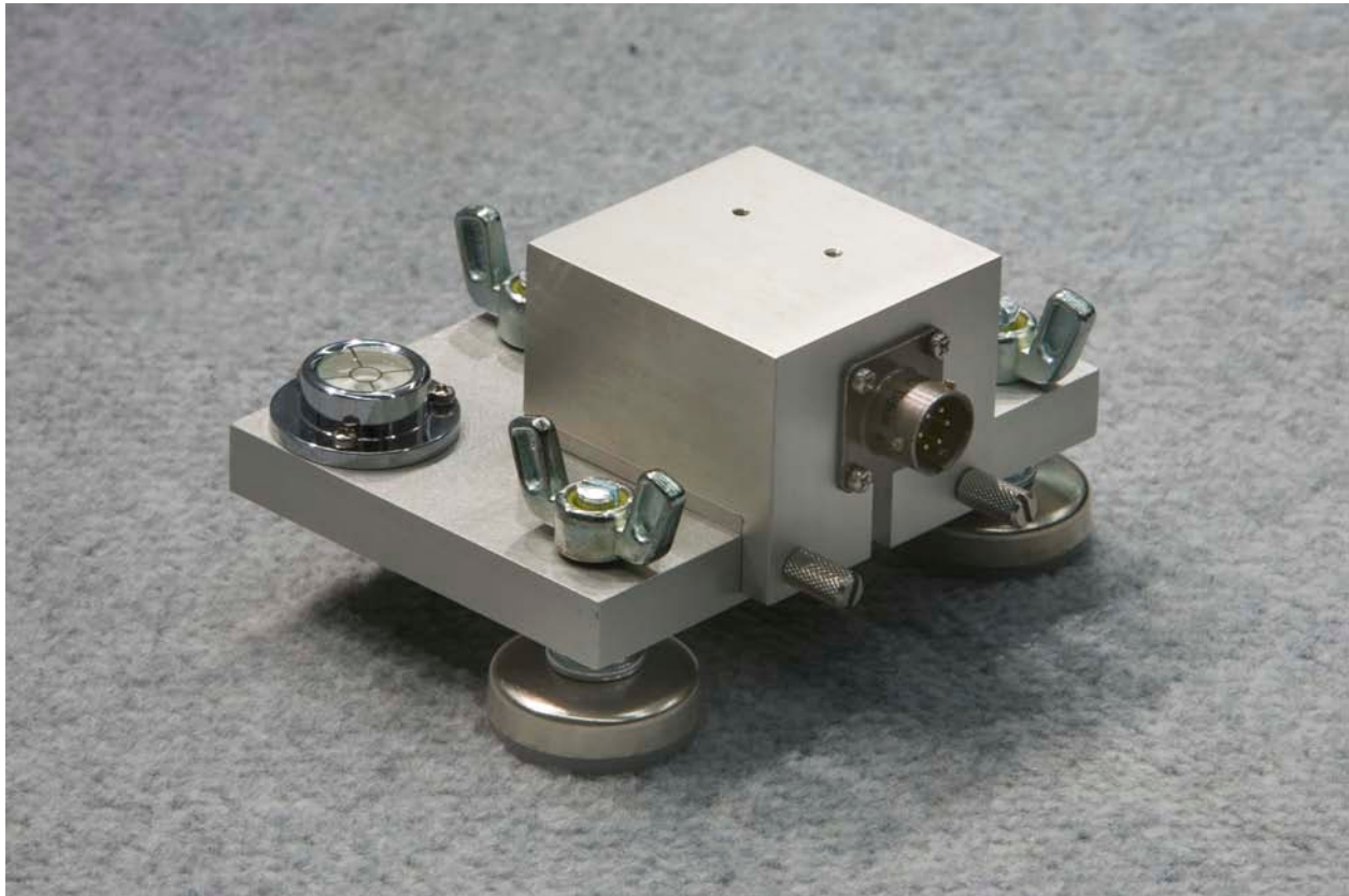
Figure 47. Photo. Accelerometer box.
