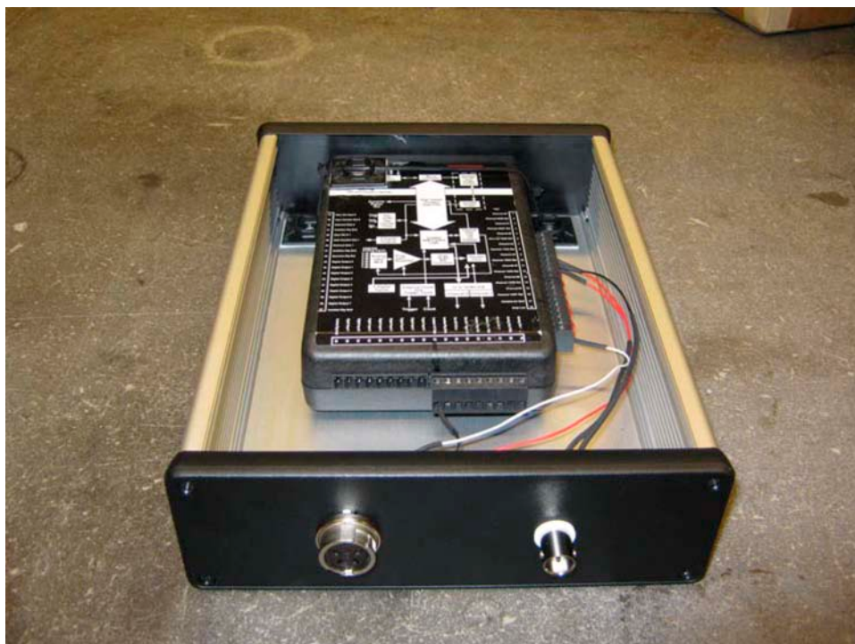
Figure 11. Photo. Box for DAQ wiring protection.
