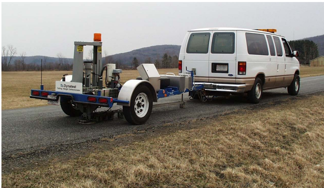
Figure 6. Photo. Dynatest® model 8000 trailer-mounted FWD.
