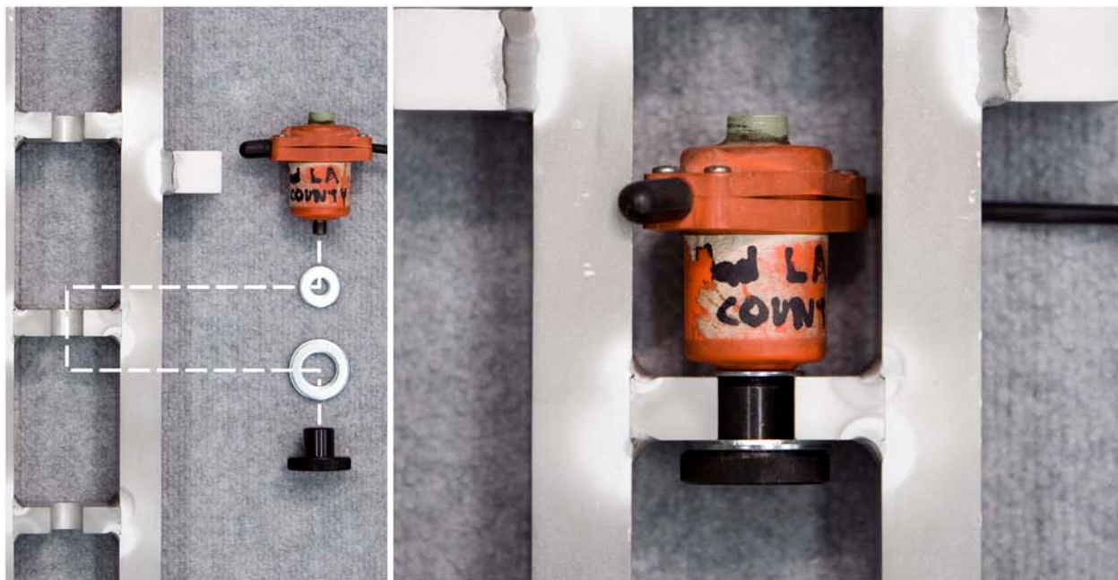
Figure 34. Photo. Attachment of a JILS geophone in the stand.
