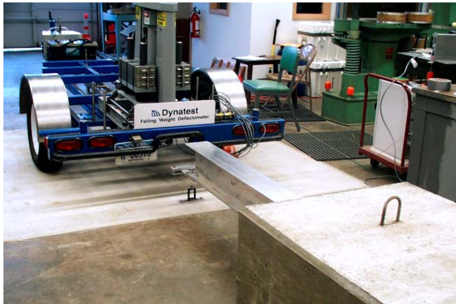
Figure 10. Photo. FWD calibration beam and inertial block.
