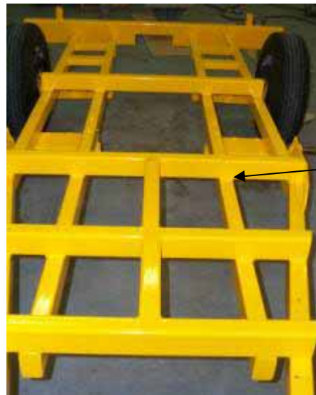
Figure 7. Rear of newly powdered trailer.
