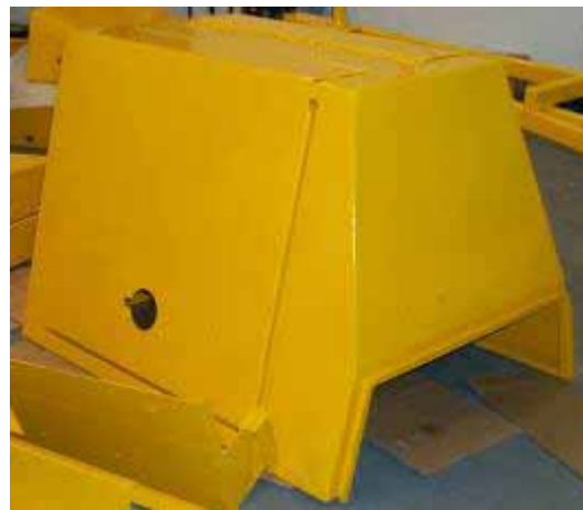
Figure 9. Top trailer cover ("dog house").
