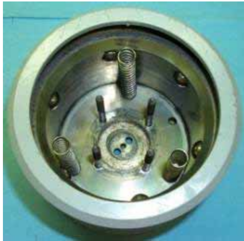
Figure 75. Interior of catch assembly with compression springs.
