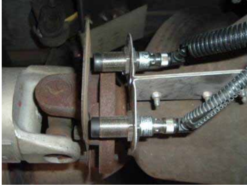
Figure 132. Vehicle-mounted proximity switches.
