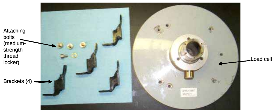
Figure 94. Load plate with mounting brackets.
