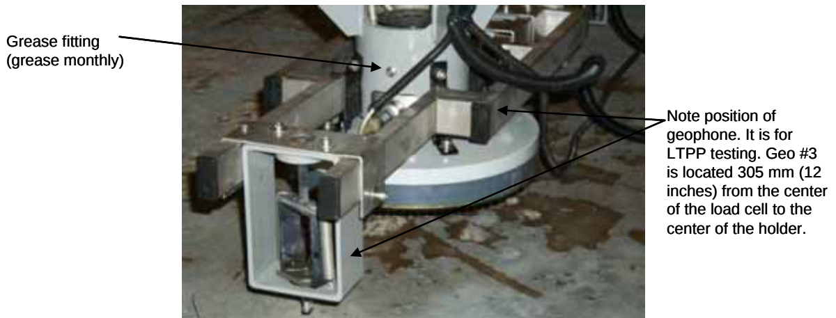
Figure 110. Rear view of raise/lower assembly.
