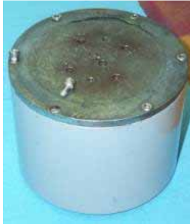
Figure 73. Inner catch top cover installed.
