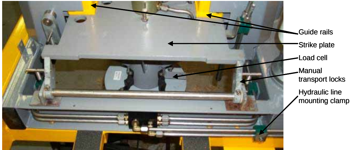
Figure 90. Load cell mounted to the strike plate.
