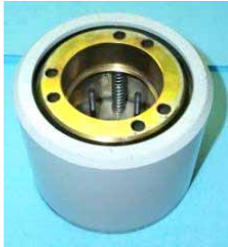
Figure 77. Outer shell with inner ring in position.
