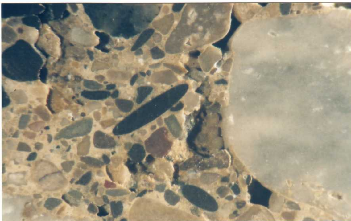
Figure 6.15 - Enlarged Section View of LCB Core Showing Gross Porosity
