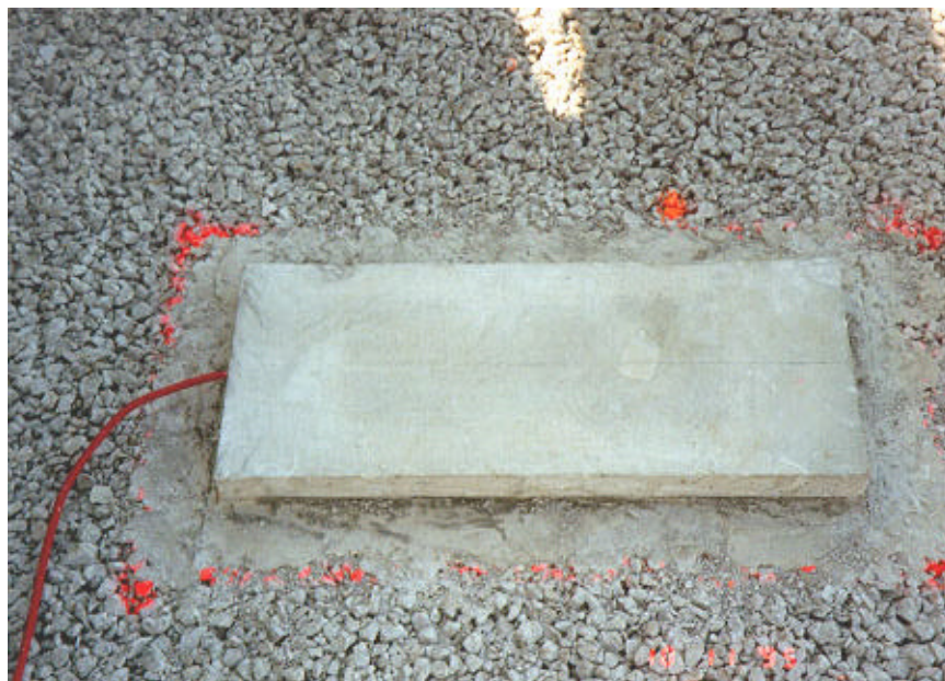
Figure 12.15 Geokon Model 3500 Pressure Cell Setup
