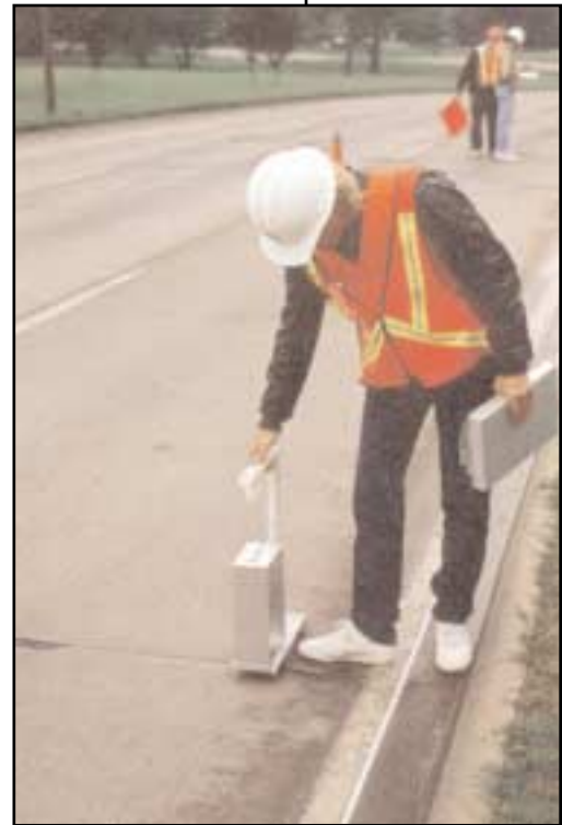
FIGURE B1 The Georgia Faultmeter in Use
