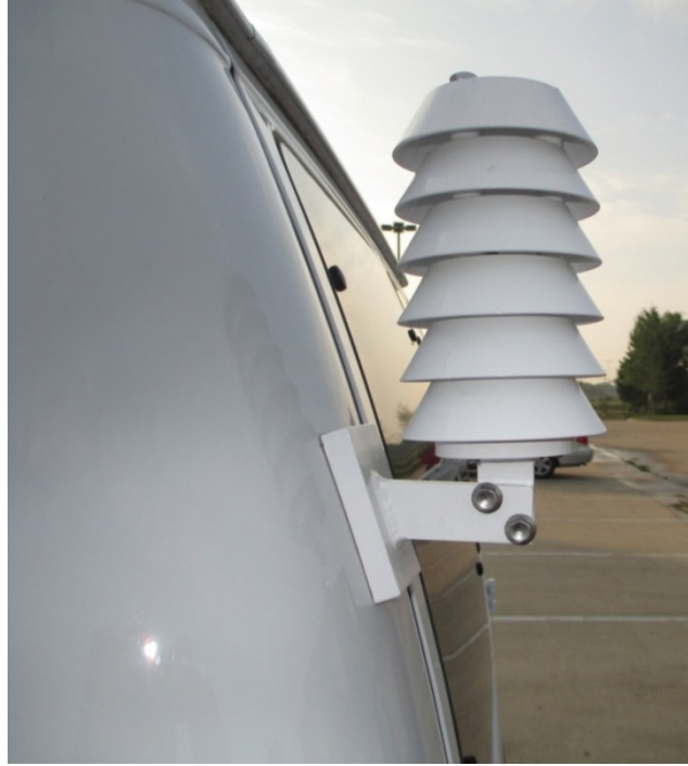
Figure 16. Protective shield housing the ambient temperature sensor.
