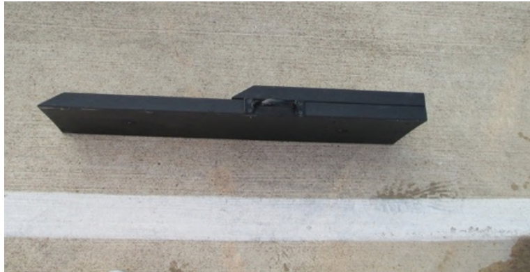
Figure 40. Ramp used to elevate vehicle.
