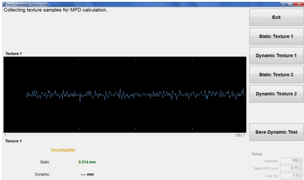
Figure 116. Texture reference test screen after static test.
