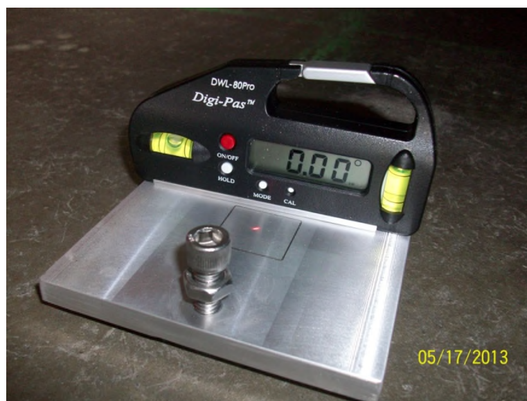
Figure 74. Laser dot centered on base plate.
