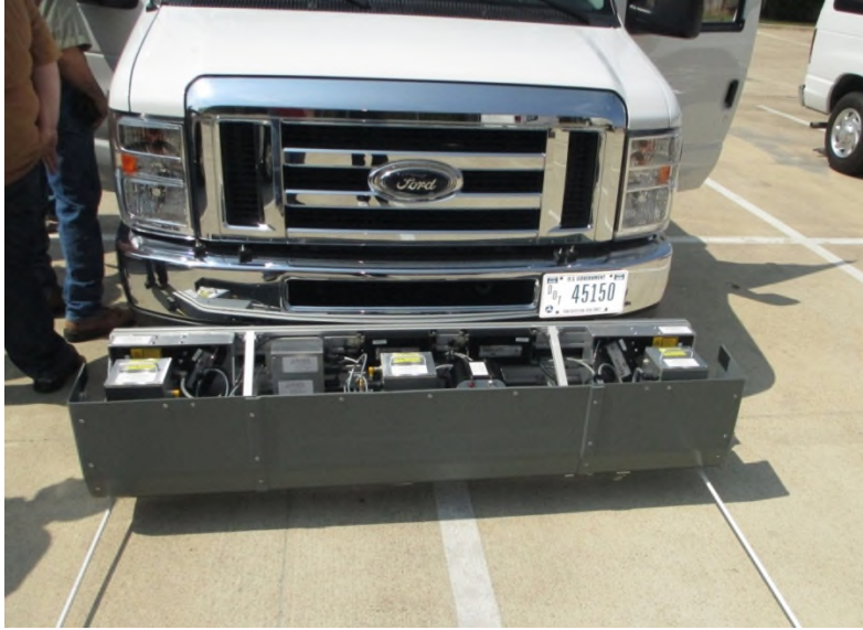
Figure 3. Sensor bar with the cover open.
