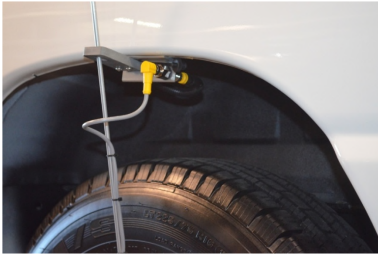
Figure 13. DMI input connection.
