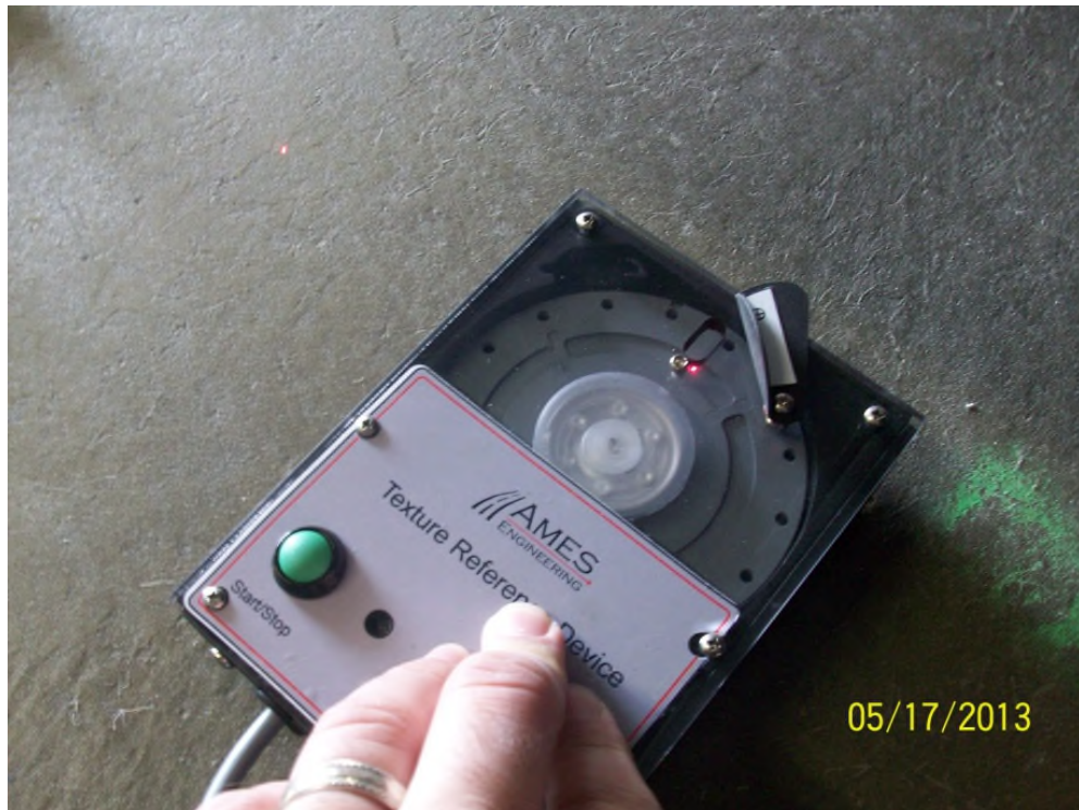
Figure 117. Cover open on texture reference test device.
