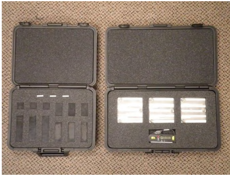
Figure 36. Calibration block kit.
