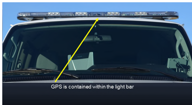
Figure 15. Location of the GPS receiver.
