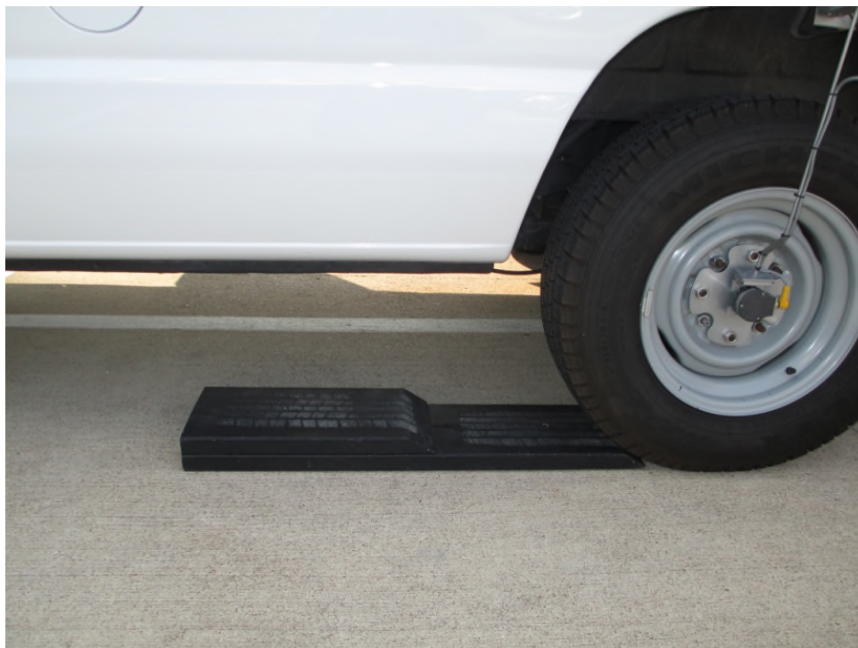
Figure 101. Ramps placed in front of the tire before driving vehicle up the ramp.
