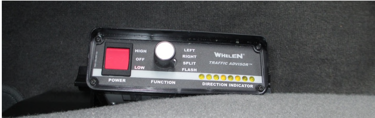
Figure 22. Control switch for directional warning light.
