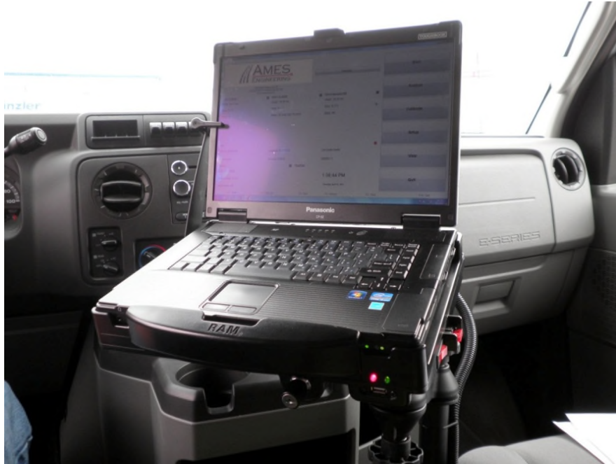
Figure 33. Laptop computer docking station with laptop computer.
