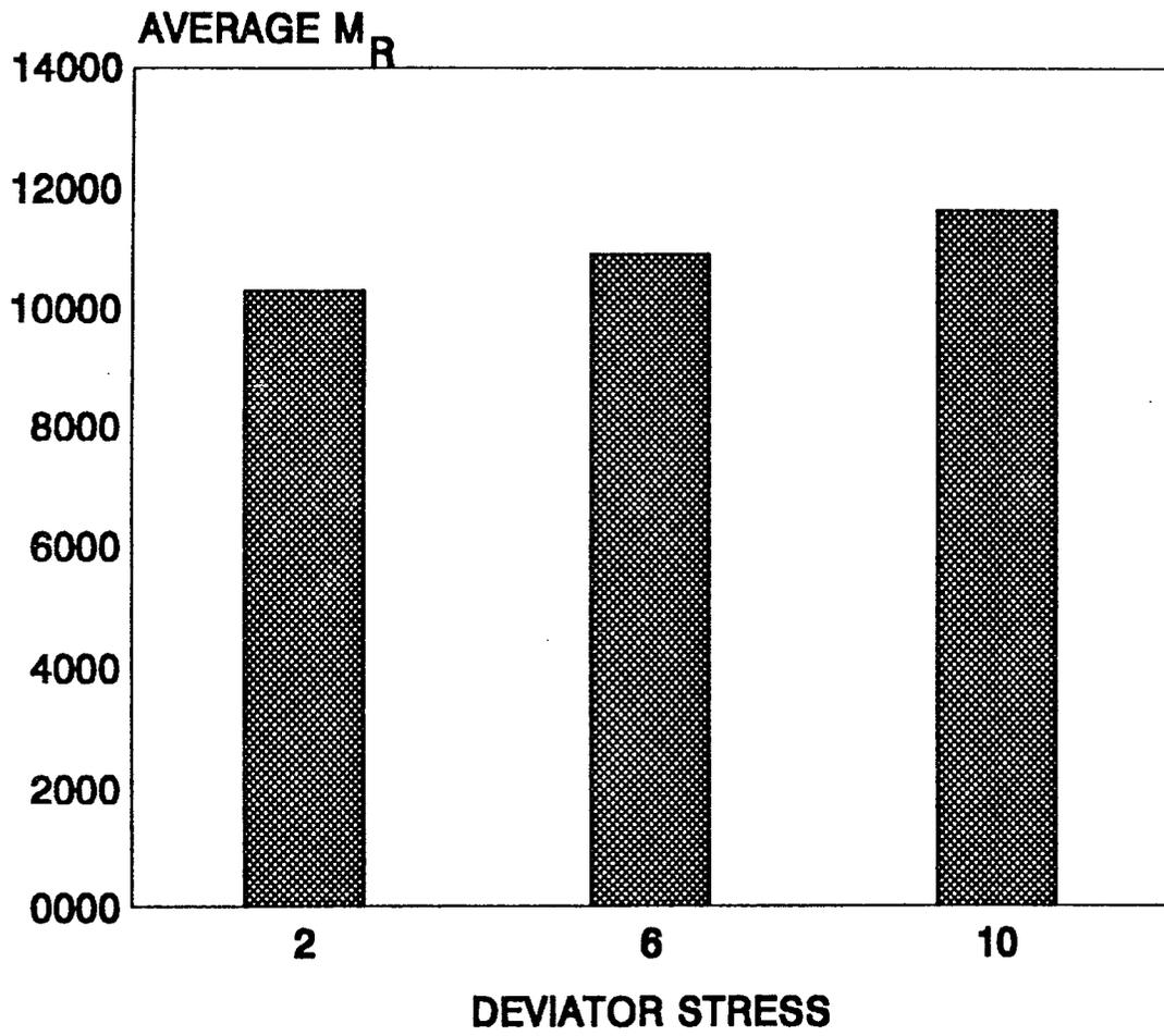
Figure 6. Average M<sub>R</sub> by Deviator Stress for Synthetic Specimen TU-960.
