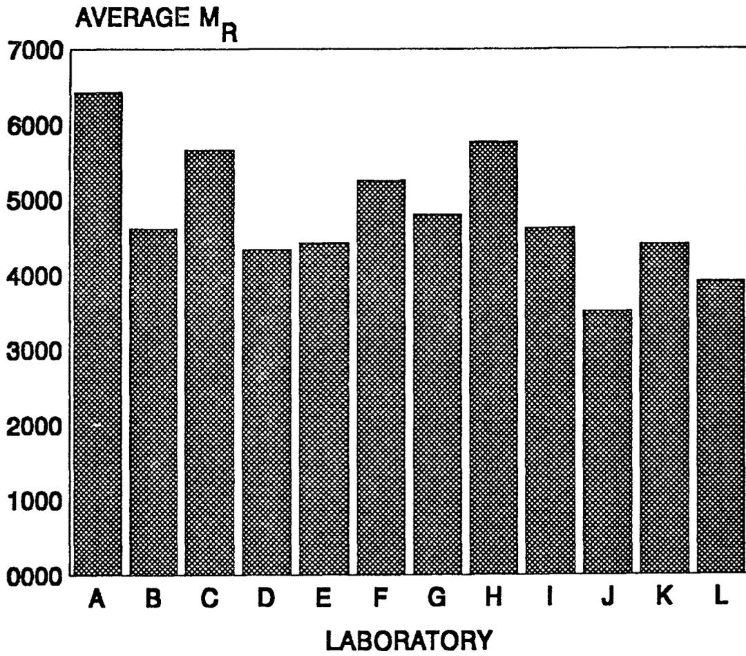
Figure 2. Laboratory Averages for Synthetic Specimen DPTU-1560.
