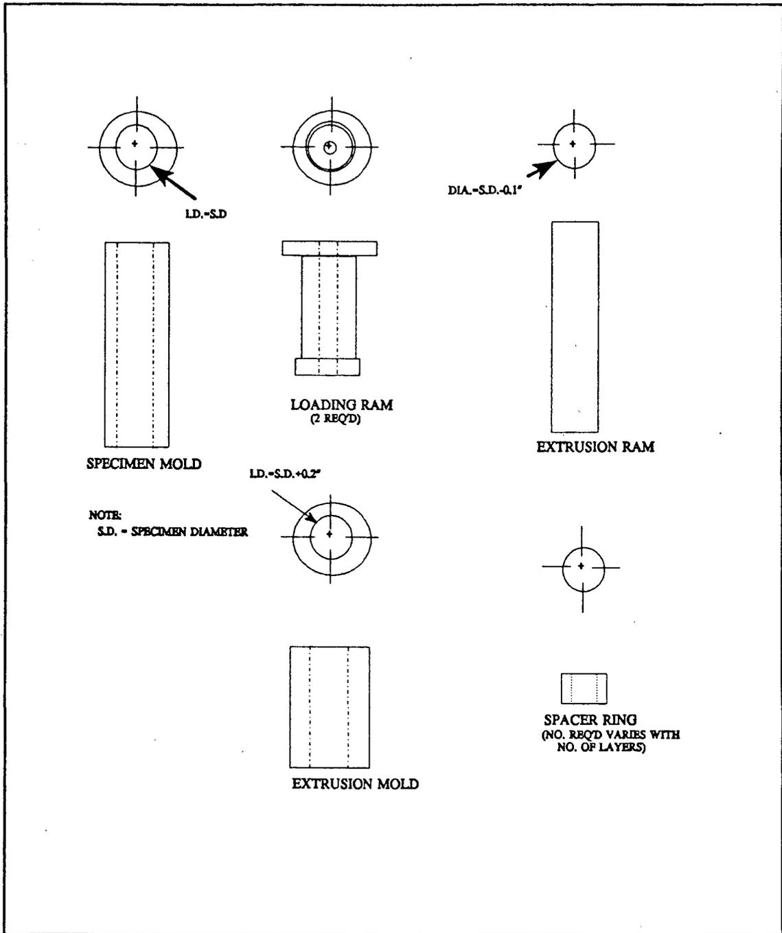
Figure 3. Apparatus for static compaction of Type 2 unbound materials.
