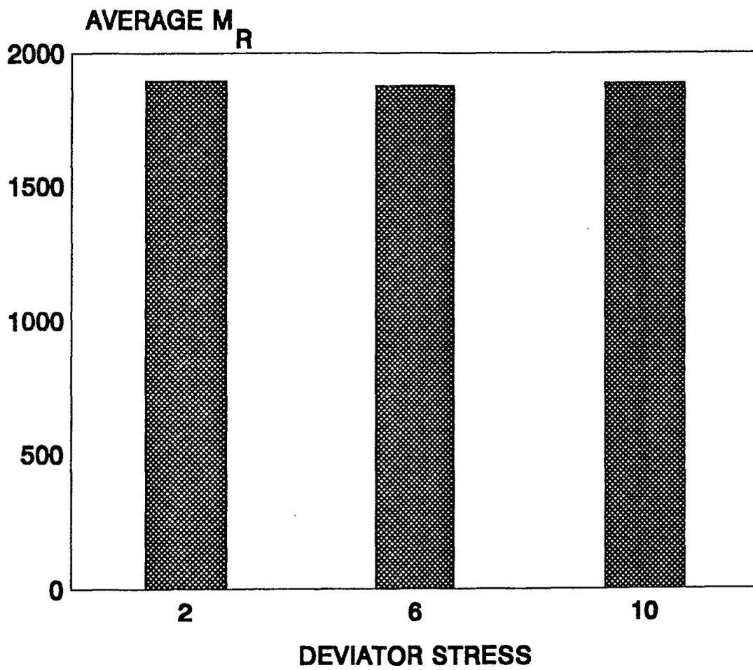
Figure 4. Average M<sub>R</sub> by Deviator Stress for Synthetic Specimen TU-700.
