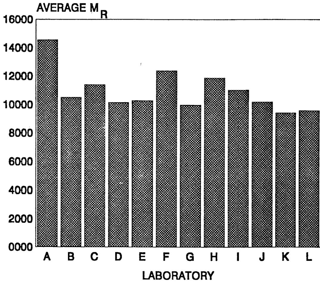
Figure 3. Laboratory Averages for Synthetic Specimen TU-960.
