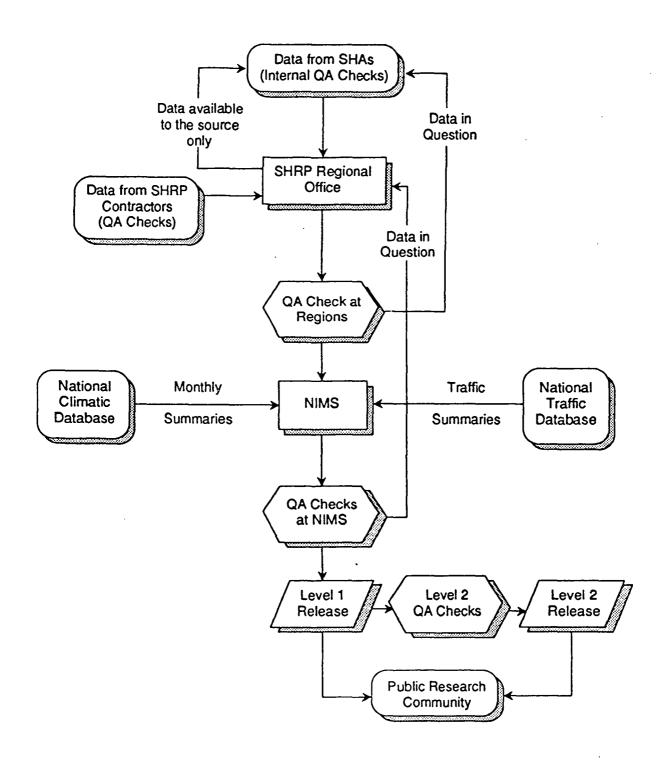
FIGURE 4 Data Flow in the LTPP IMS
