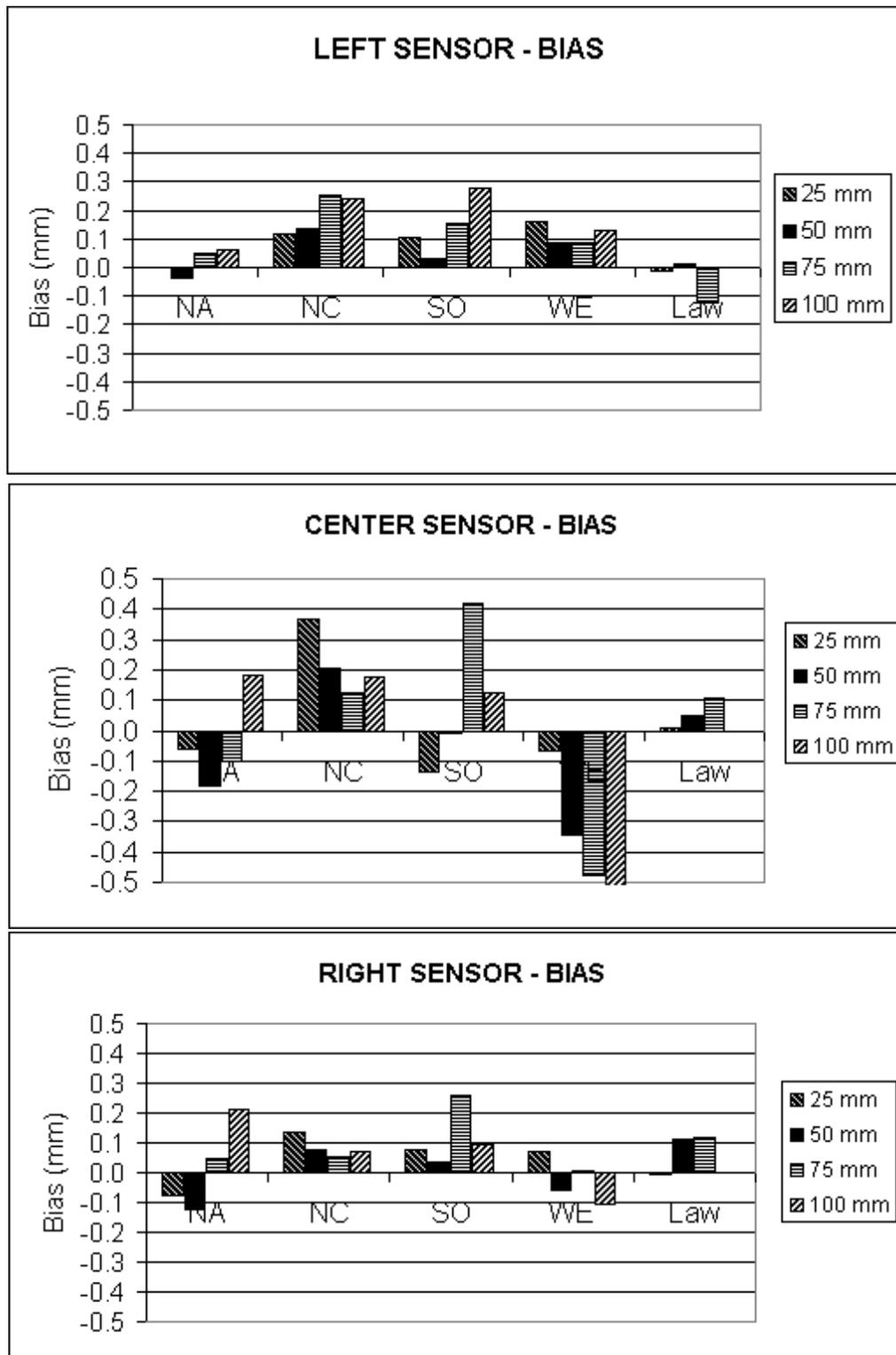
Figure 3.1. Bias values from static height sensor test (NA- North Atlantic, NC – North Central, SO – Southern, WE – Western).
