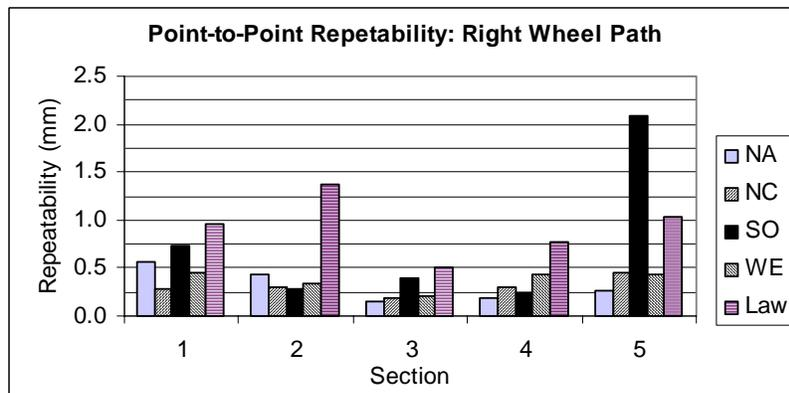
Figure 6.8 Point-to-point repeatability – right wheel path.
