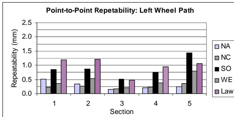
Figure 6.7. Point-to-point repeatability – left wheel path.
