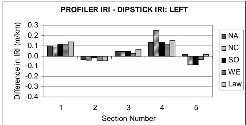
Figure 6.5. Difference between profiler and Dipstick IRI, left wheel path.
