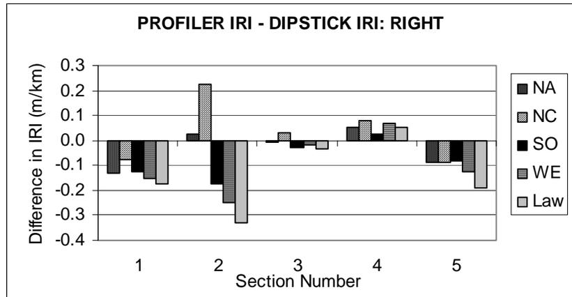
Figure 6.6. Difference between profiler and Dipstick IRI, right wheel path.
