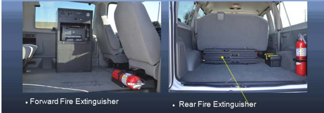
Figure 35. Fire extinguishers in the vehicle.
