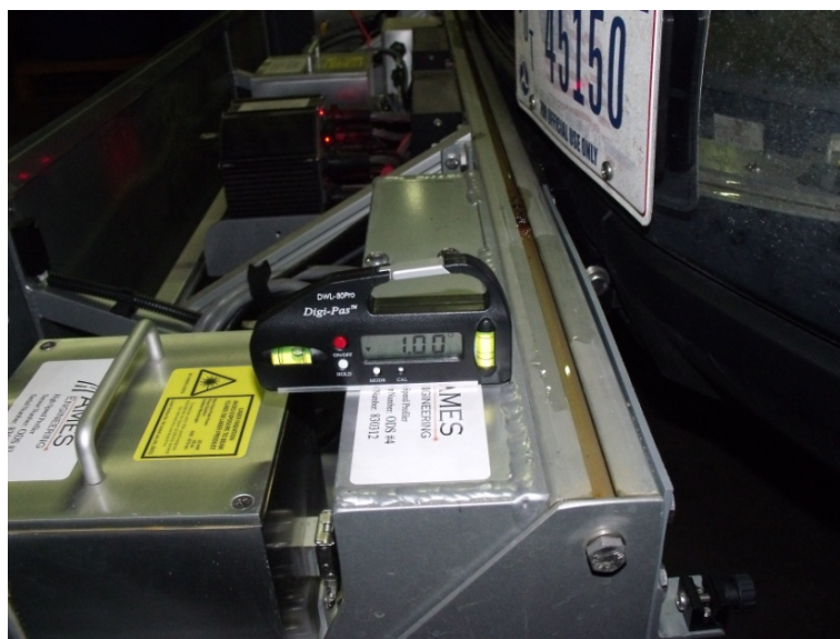
Figure 118. Level placed on top of texture laser perpendicular to sensor bar.
