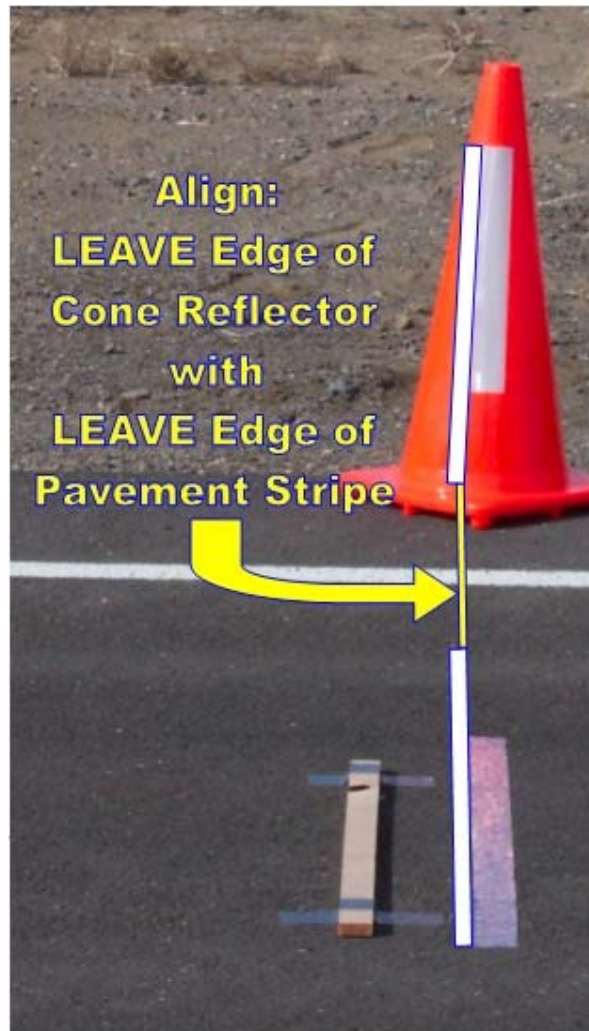
Figure 127. Placement of vertical photocell target in relation to section starting location.
