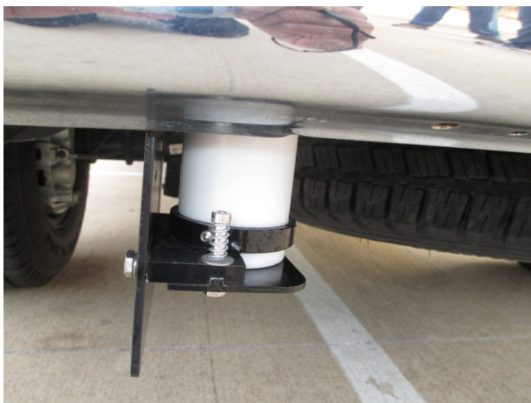
Figure 17. Protective cover covering the pavement surface temperature sensor.
