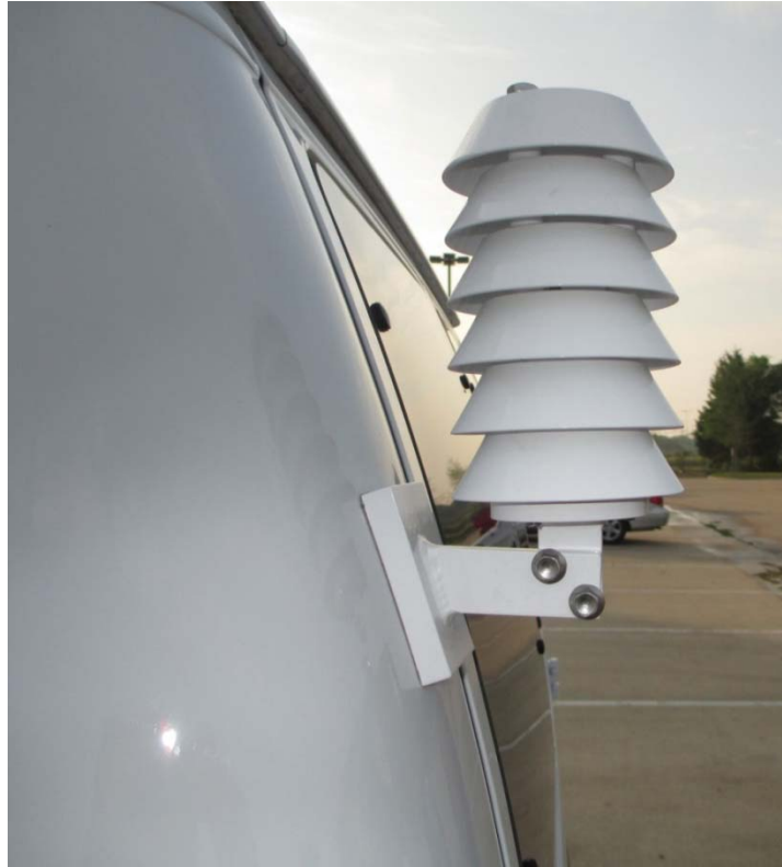
Figure 16. Protective shield housing the ambient temperature sensor.
