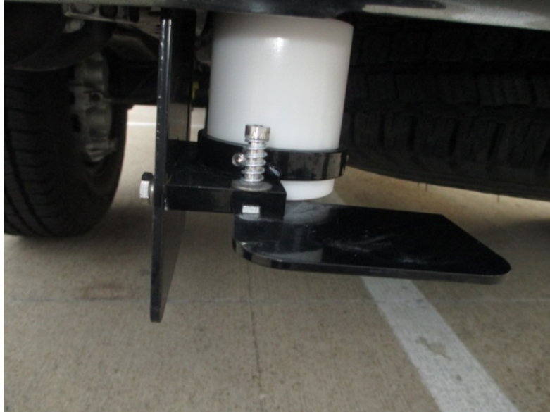
Figure 18. Protective cover open to permit pavement surface temperature measurements.
