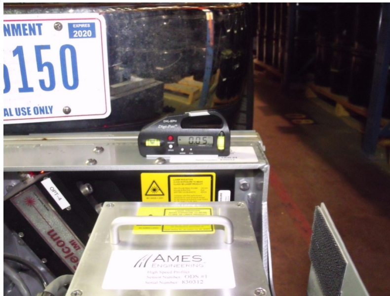
Figure 117. Level placed on top of texture laser parallel to sensor bar.
