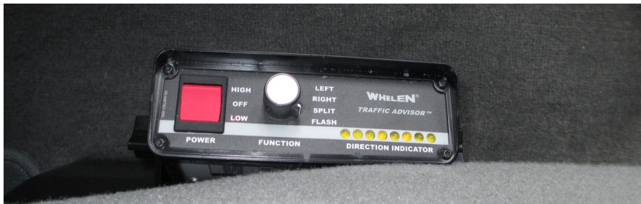
Figure 22. Control switch for directional warning light.
