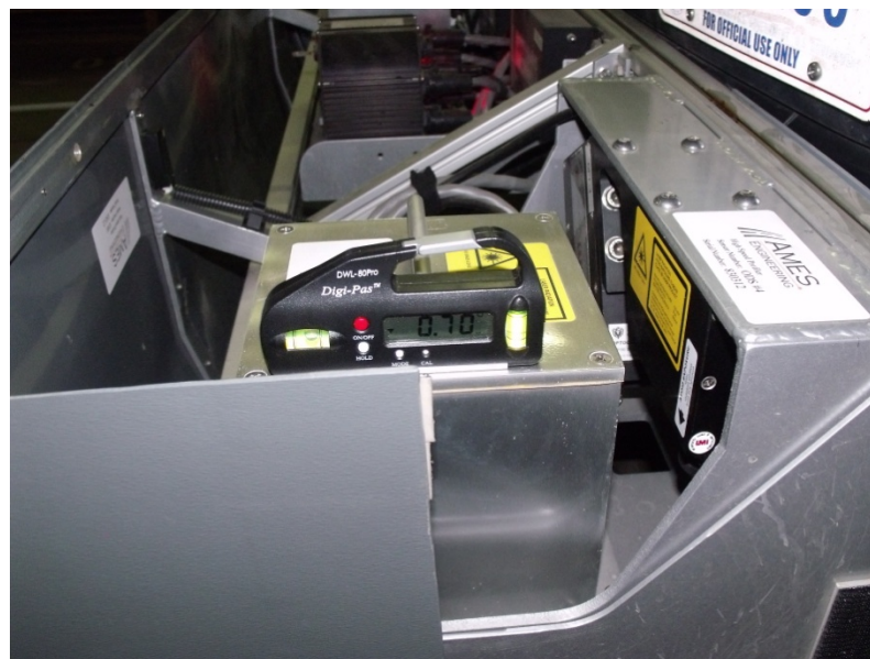
Figure 108. Level placed on top of laser box perpendicular to sensor bar.
