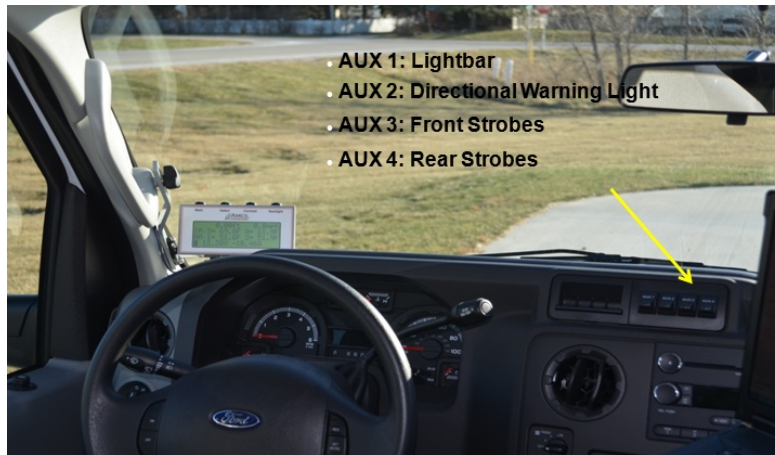
Figure 21. Uplifter switches used to control the safety lighting.
