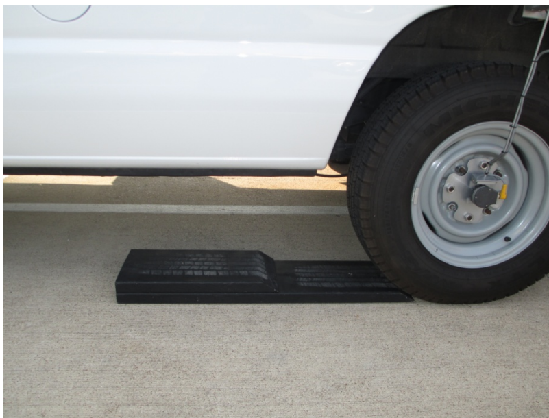
Figure 103. Ramps placed in front of the tire before driving vehicle up the ramp.
