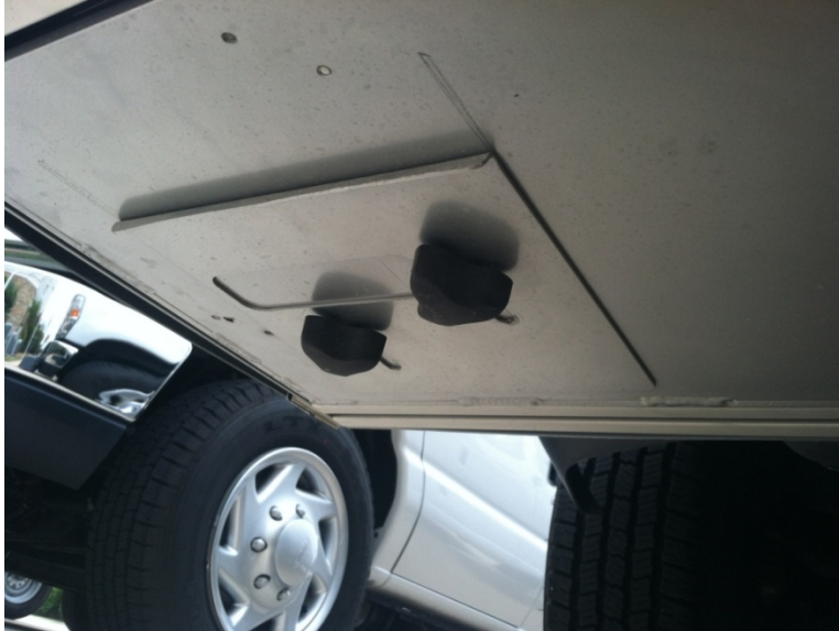
Figure 63. Protective cover that protects the laser sensors.
