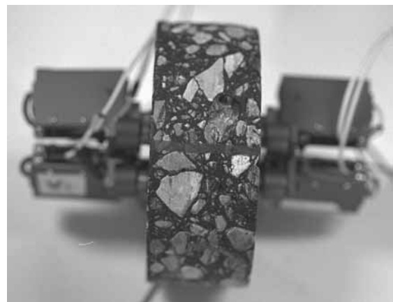
Figure 11. Asphalt specimen with extensometers mounted
