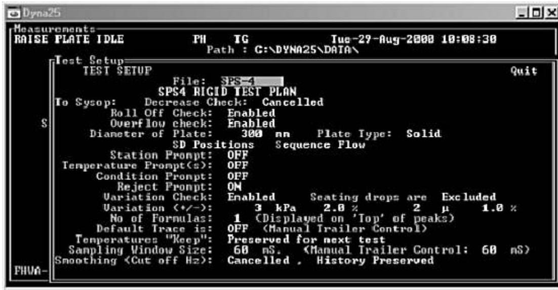
Figure G-1.27 Test Setup - SPS4 Rigid Test Plan
