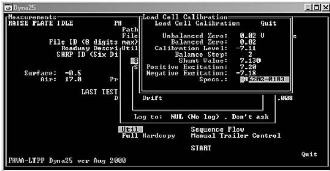
Figure G-1.33 Load Cell Calibration
