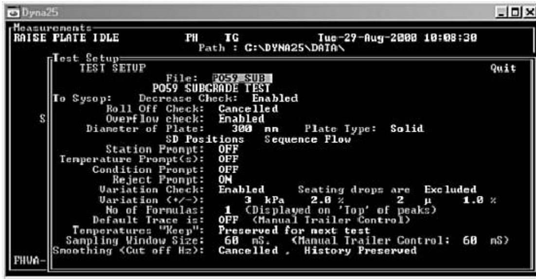
Figure G-1.23 Test Setup - P059 Subgrade Test
