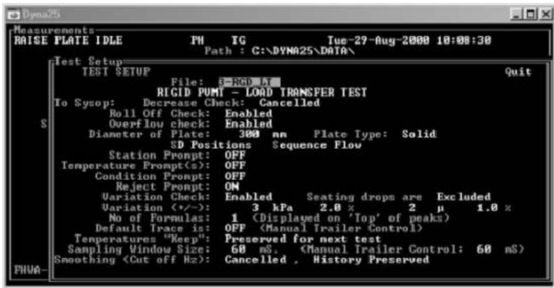
Figure G-1.16 Test Setup - Rigid Pavement - Load Transfer Test
