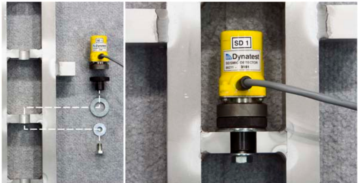
Figure 121. Photo. Attachment of a Dynatest® geophone to the stand.
