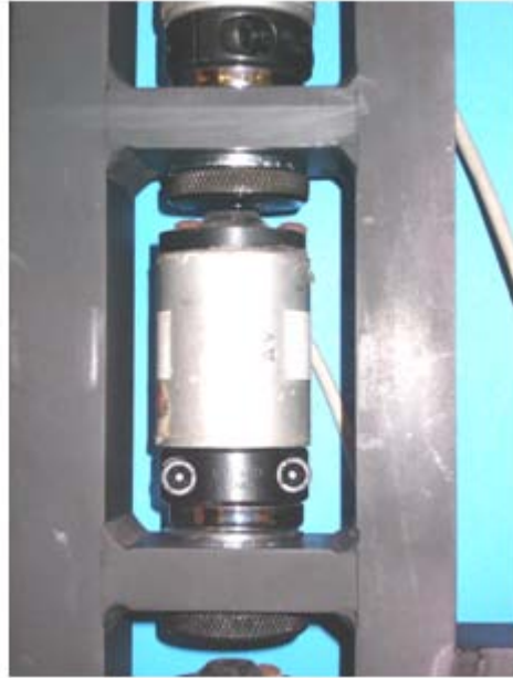
Figure 36. Photo. Attachment of a KUAB geophone in the stand.
