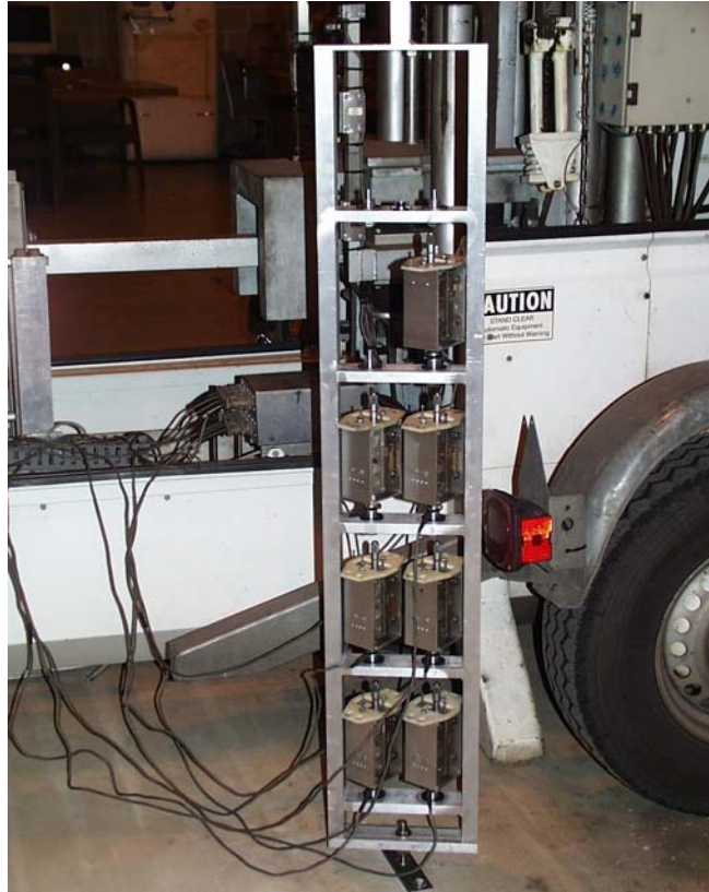
Figure 124. Photo. Seismometer stand with sensors attached.
