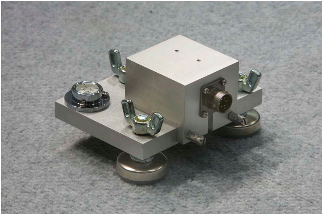
Figure 47. Photo. Accelerometer box.
