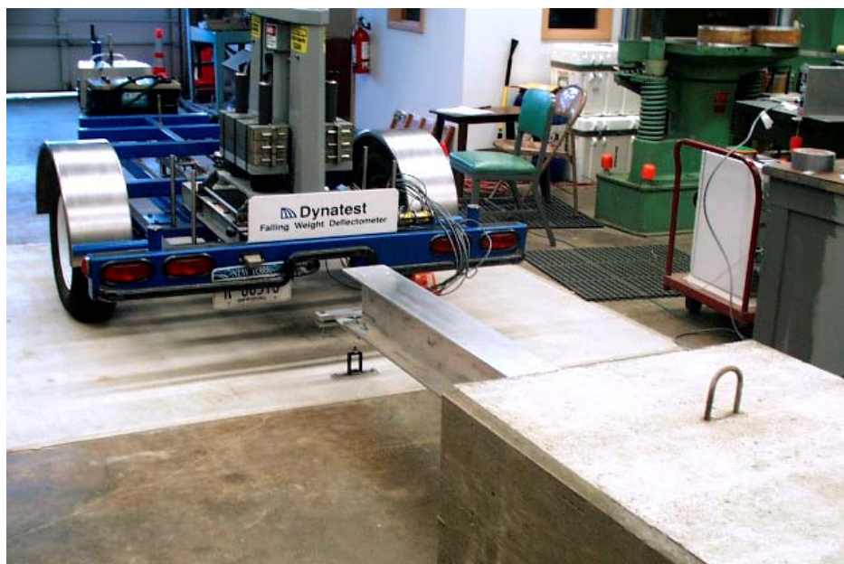
Figure 10. Photo. FWD calibration beam and inertial block.
