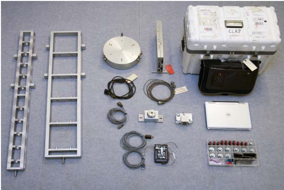
Figure 4. Photo. Calibration system hardware set.
