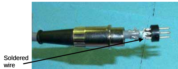
Figure 126. Internal view of the DIN plug.
