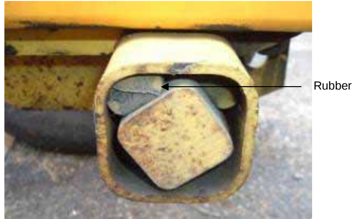
Figure 12. Torsion tube housing.
