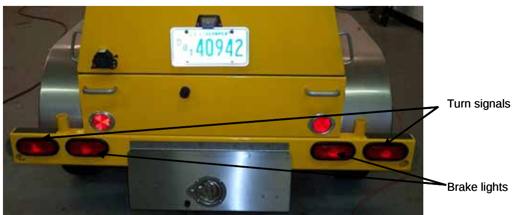
Figure 24. Trailer turn signal and brake lights.
