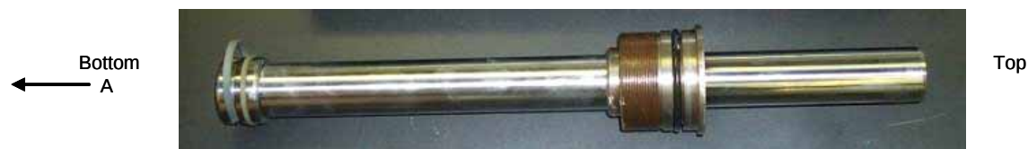
Figure 61. Center cylinder and gland.
