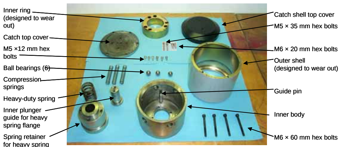
Figure 66. Upper catch shell and interior components.
