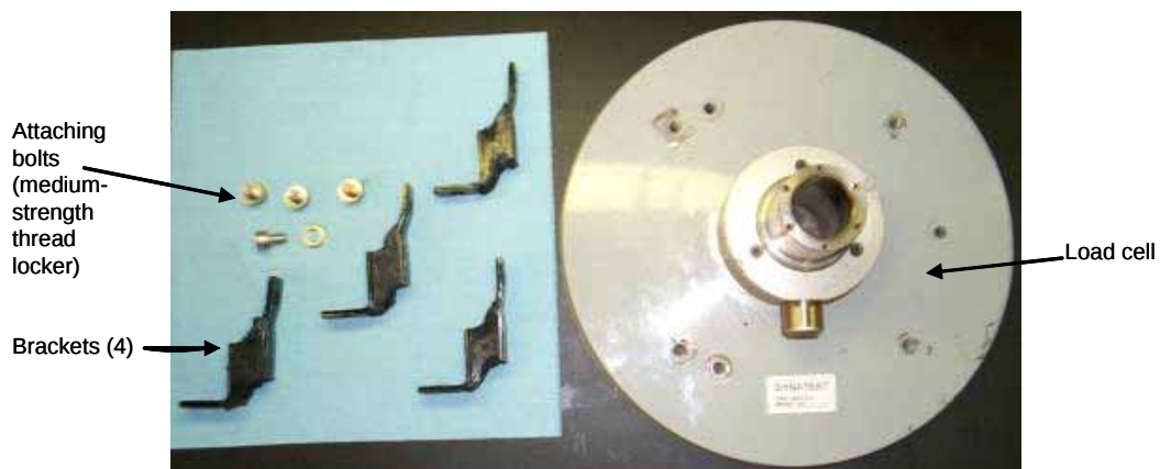
Figure 94. Load plate with mounting brackets.
