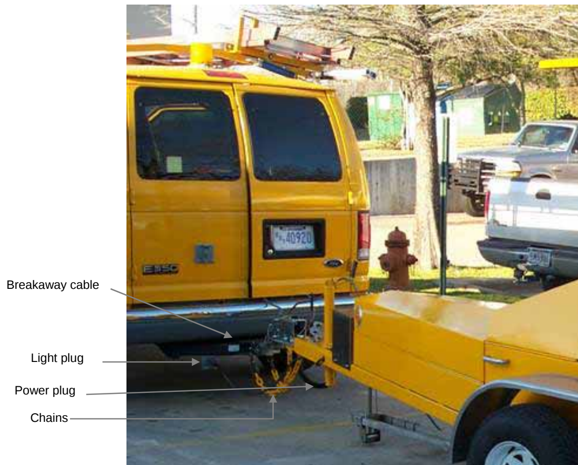
Figure 27. FWD attached to tow vehicle.
