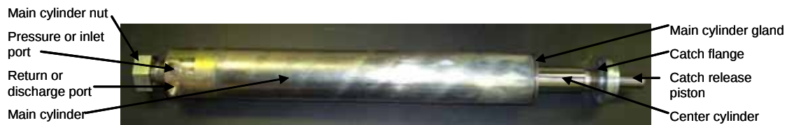
Figure 63. Assembled main cylinder.
