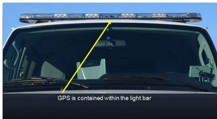
Figure 15. Location of the GPS receiver.
