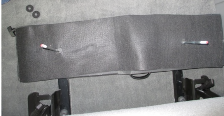
Figure 41. Mechanism for securing the ramps.
