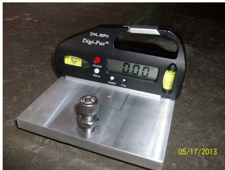
Figure 86. Laser dot centered on base plate.
