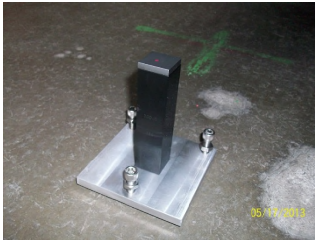
Figure 129. Calibration target on top of a 100 mm block.
