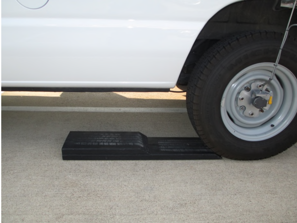
Figure 119. Ramps placed in front of the tire before driving vehicle up the ramp.
