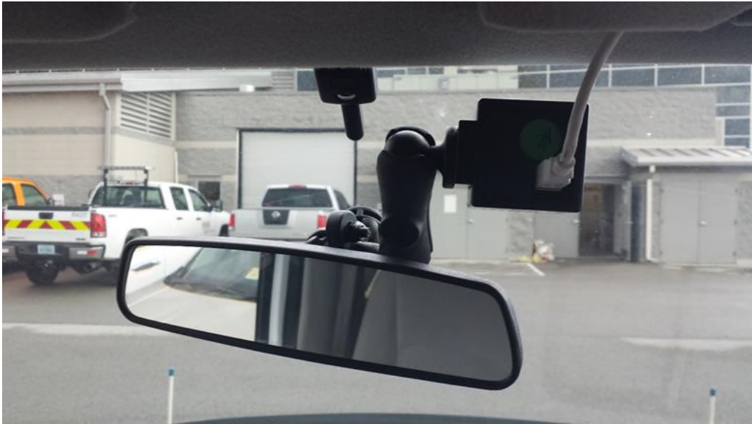
Figure 43. View from inside the vehicle of the right-of-way camera.
