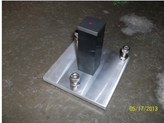
Figure 128. Calibration target on top of a 75 mm block.
