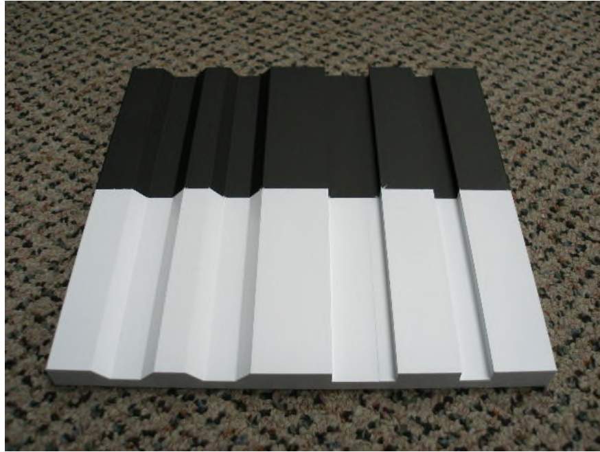
Figure 51. Side view of the TPMS calibration block.
