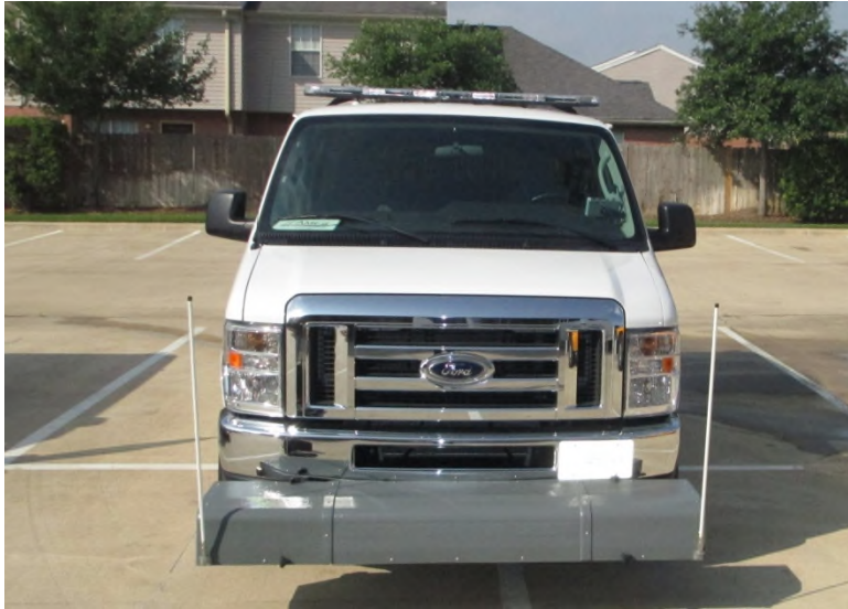
Figure 19. Light bar on front of the vehicle.
