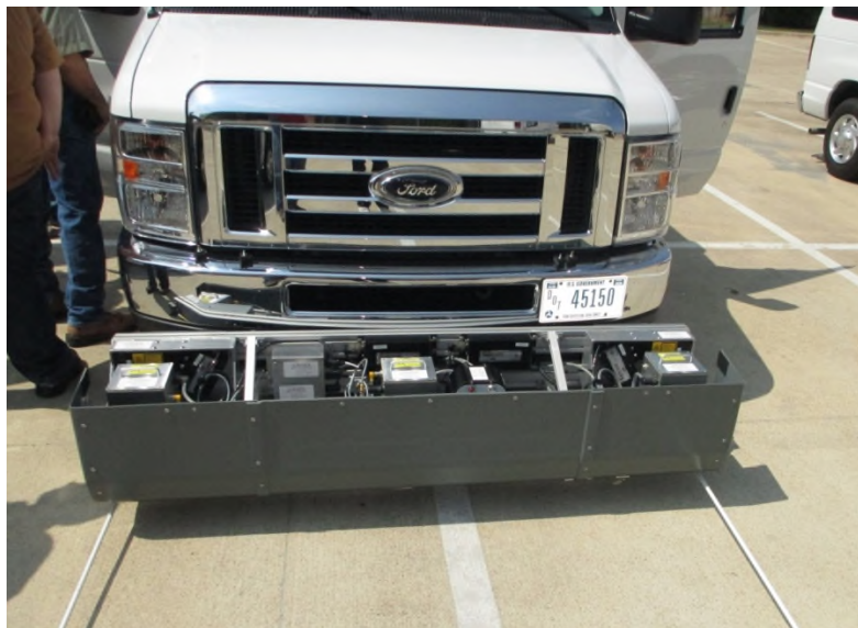
Figure 3. Sensor bar with the cover open.
