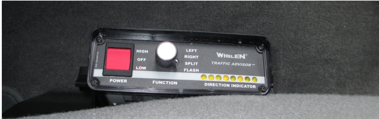
Figure 22. Control switch for directional warning light.
