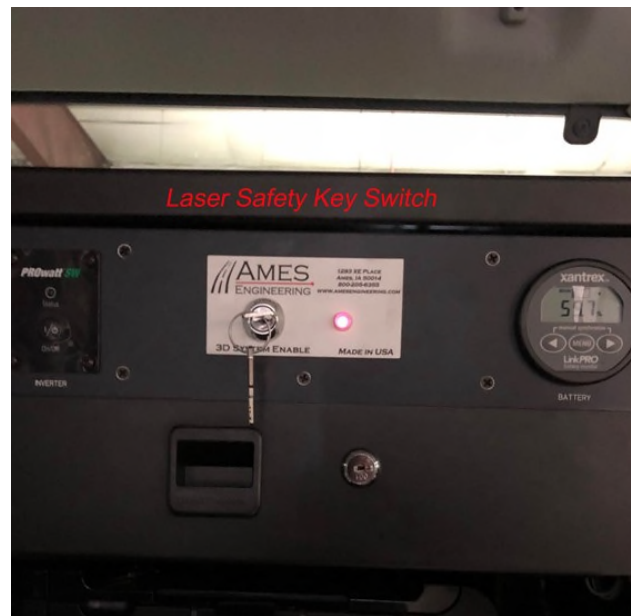
Figure 50. Laser safety key switch.
