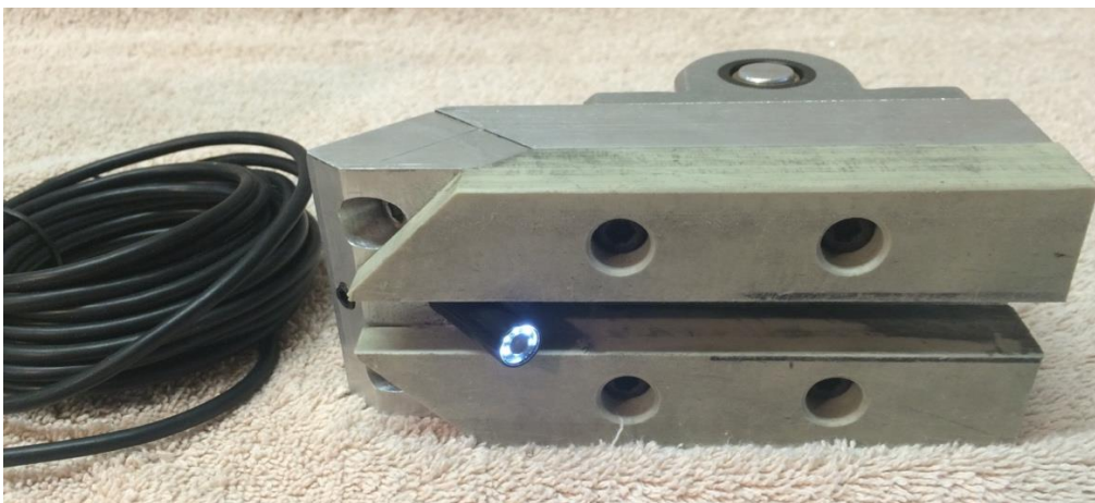
Figure 26. Photo. Lighted “endoscope” extending through the “carriage” slot.
