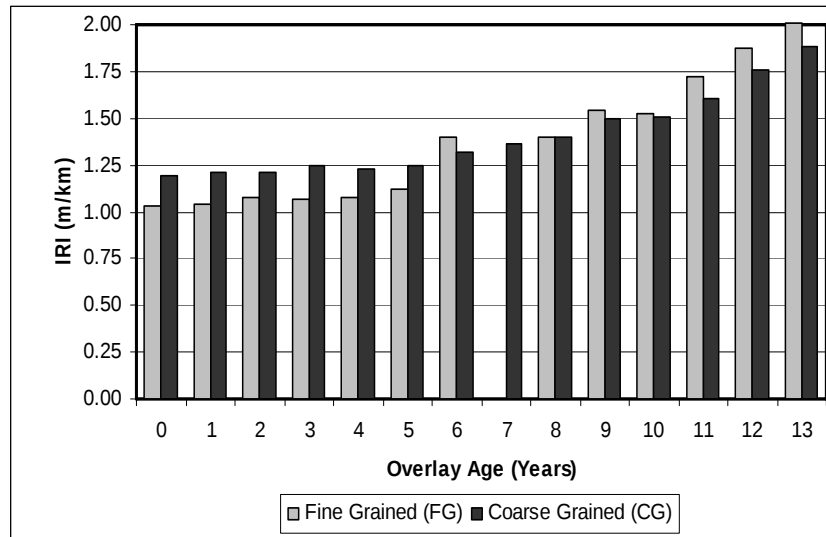
Figure 6. Effect of subgrade type on roughness progression in medium overlays with wet-freeze climatic zones.
