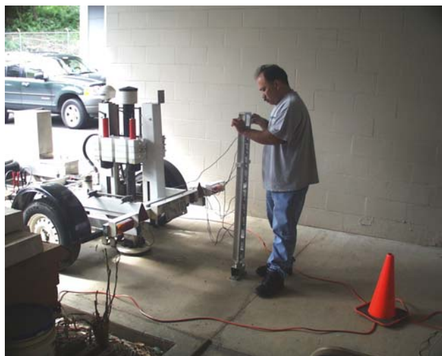
Figure 3. On-Site FWD Calibration in Hawaii
