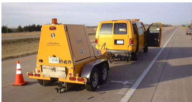
Figure 2. LTPP FWD in Operation.
