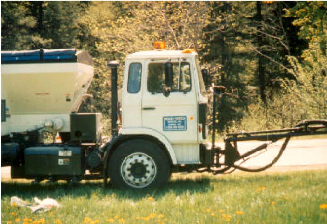
Figure 8. Spray-injection device—self-contained unit.
