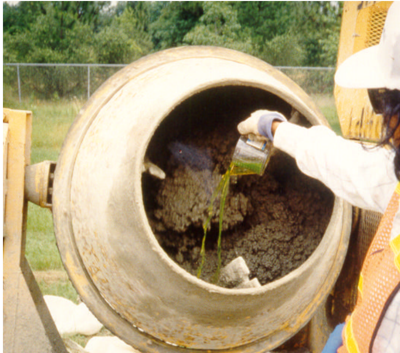
Figure 20. Adding carefully measured components to a drum mixer.
