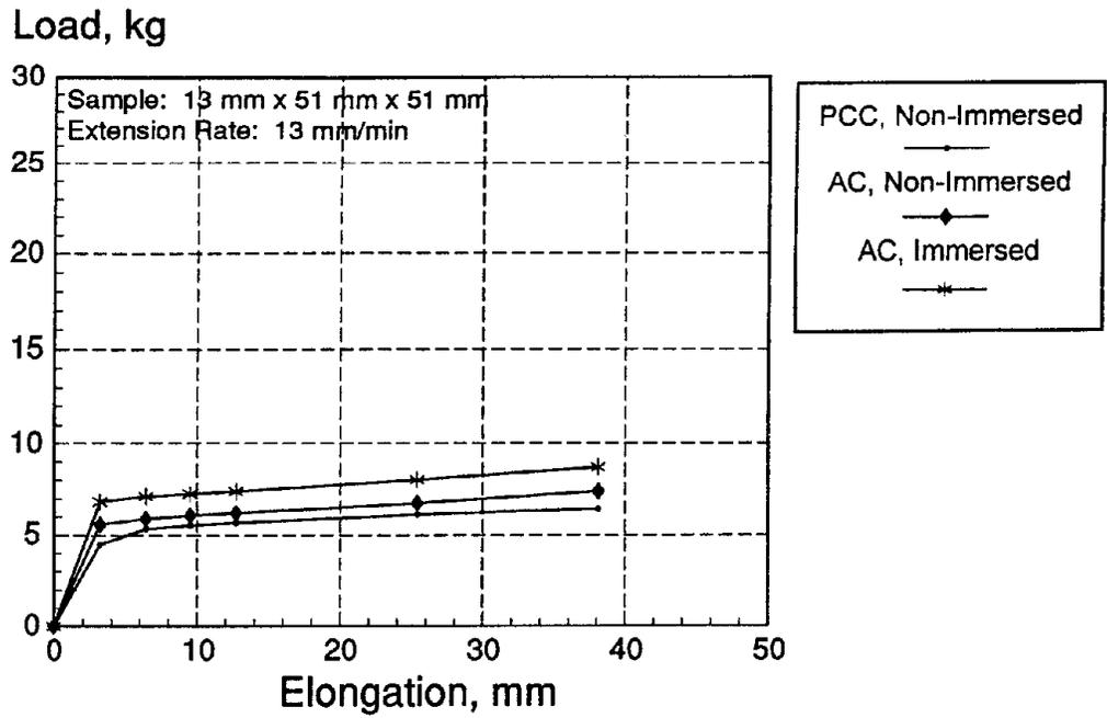
Figure C-7. ASTM D 3583 load-deformation curves for RS 515.
