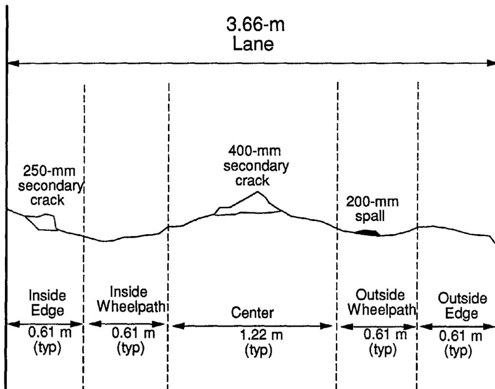
Figure 9. Initial inspection sketch of transverse crack.
