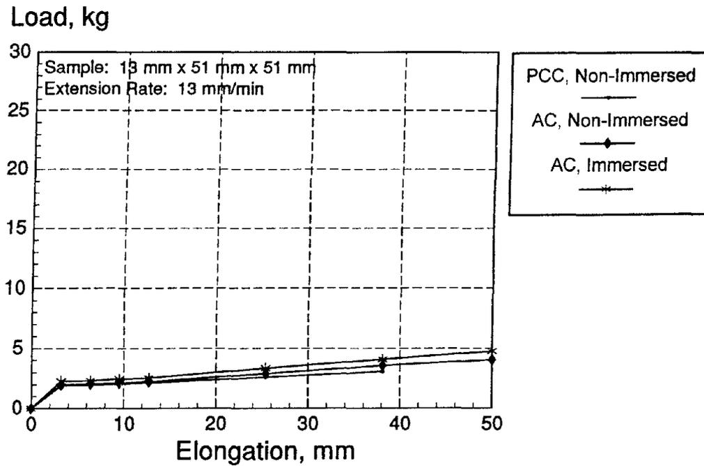
Figure C-9. ASTM D 3583 load-deformation curves for XLM.
