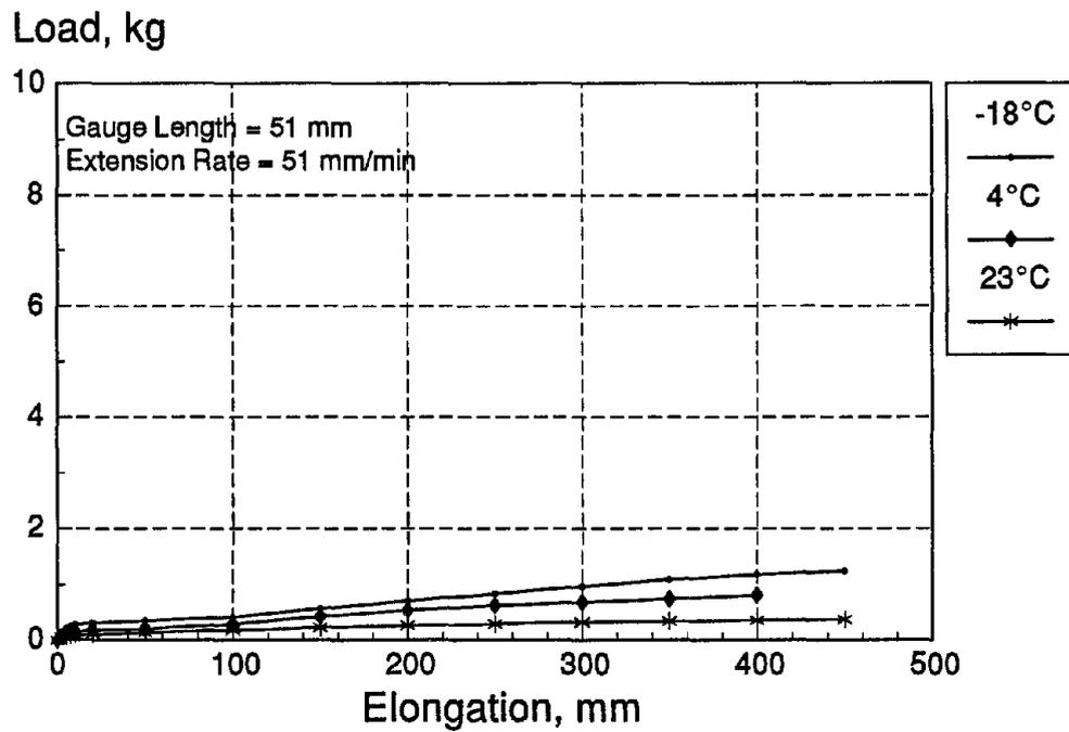
Figure C-4. ASTM D 412 load-deformation curves for XLM.
