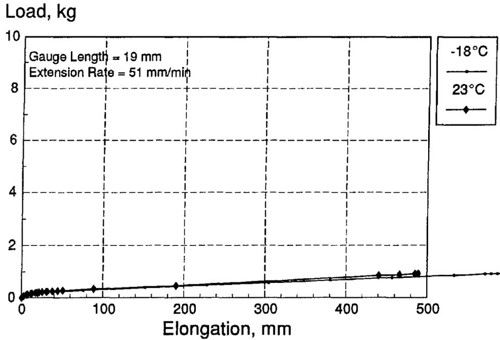
Figure C-5. ASTM D 412 load-deformation curves for 890-SL
