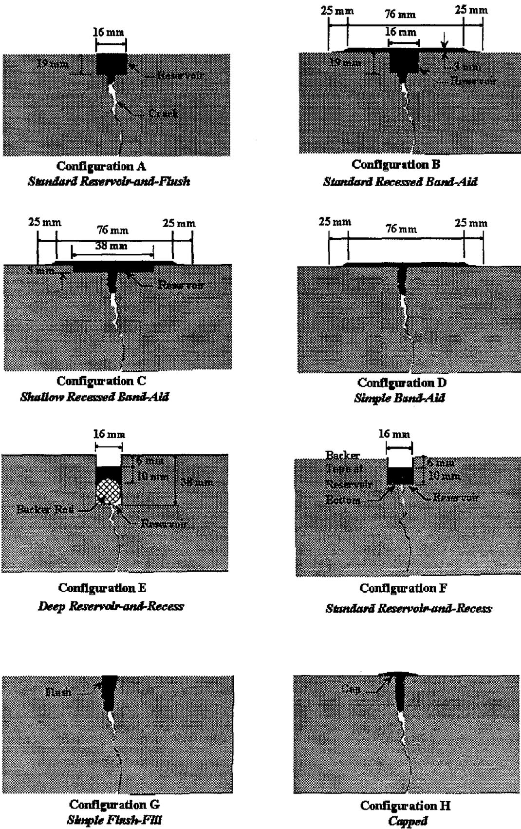
Figure 2. Material placement configurations for AC crack treatments.
