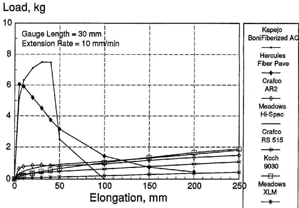
Figure 20. Force-ductility load-elongation curves for various primary materials.
