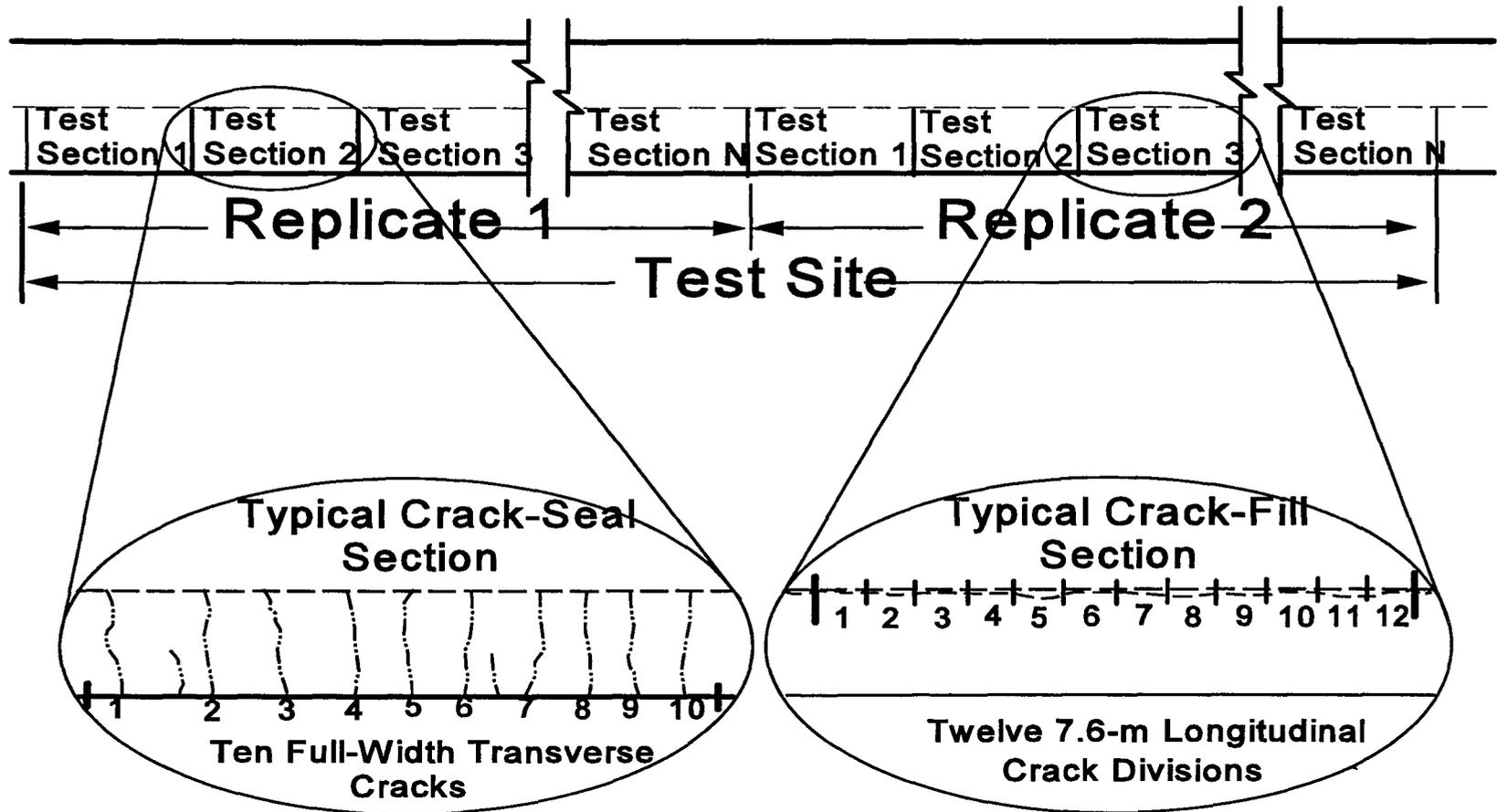
Figure 8. Conceptual layout of test sections at each test site.
