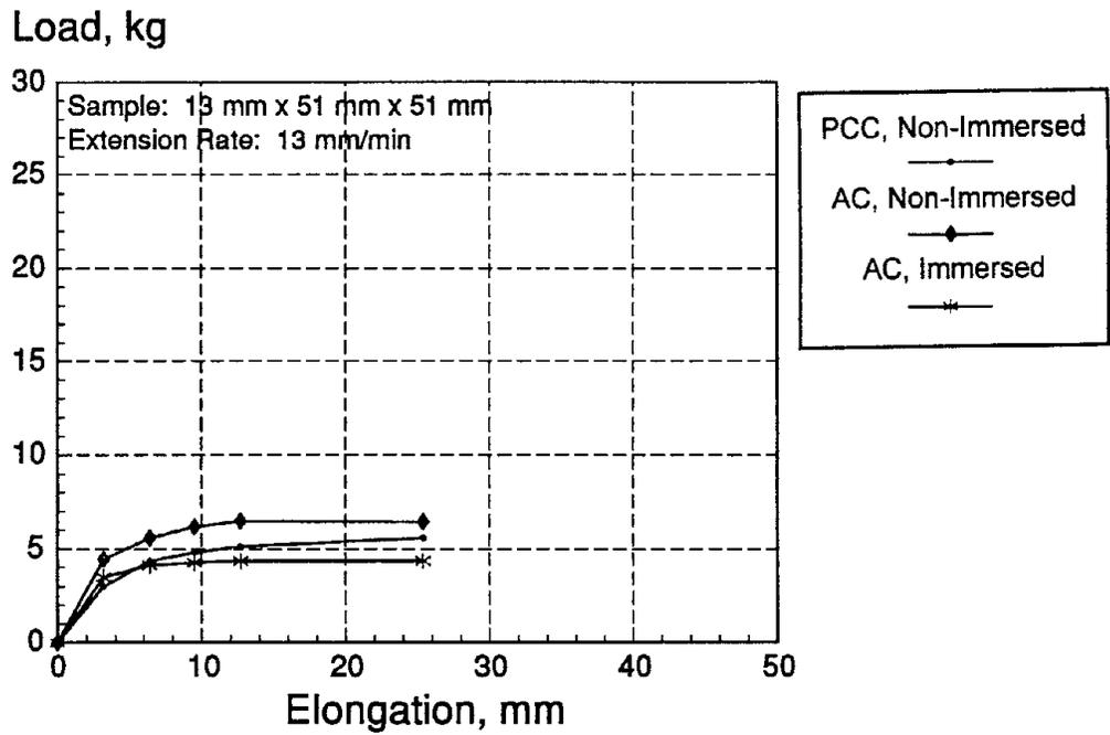
Figure C-8. ASTM D 3583 load-deformation curves for 9030.
