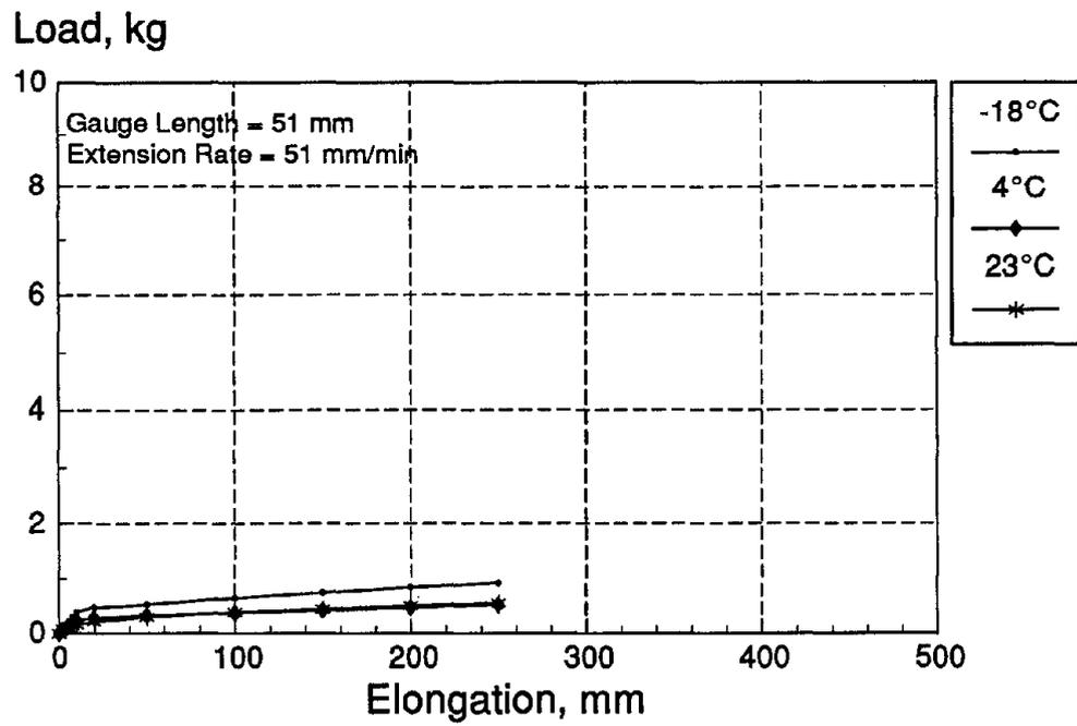
Figure C-3. ASTM D 412 load-deformation curves for 9030.
