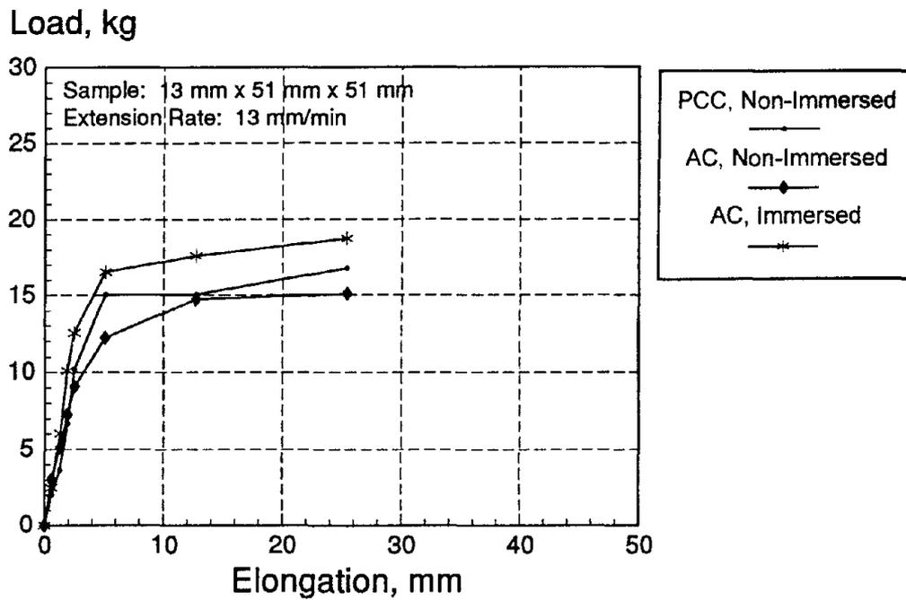
Figure C-10. ASTM D 3583 load-deformation curves for 890-SL.
