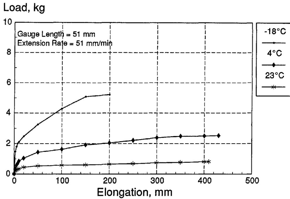
Figure C-1. ASTM D 412 load-deformation curves for Hi-Spec.
