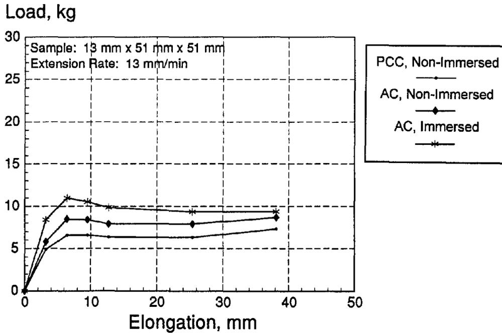
Figure C-6. ASTM D 3583 load-deformation curves for Hi-Spec.
