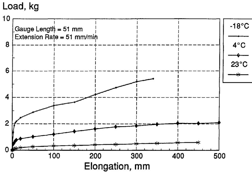
Figure C-2. ASTM D 412 load-deformation curves for RS 515.
