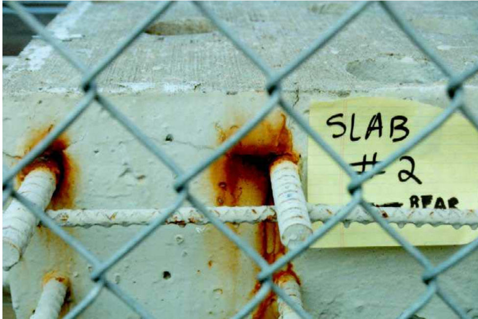
Figure 6. Photo. Cracks and corrosion products on the rear side of slab 2 in August 1998.
