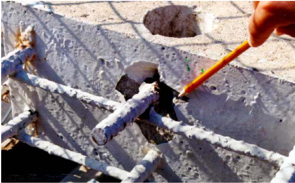
Figure 11. Photo. Corrosion and spalling on one rebar at the concrete-air interface on the side of slab 3 in September 1997.
