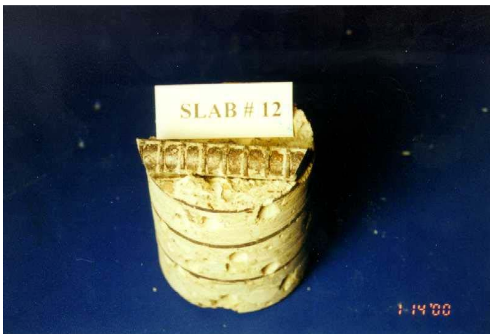
Figure 20. Photo. Autopsy of core extracted from slab 12 in December 1999.
