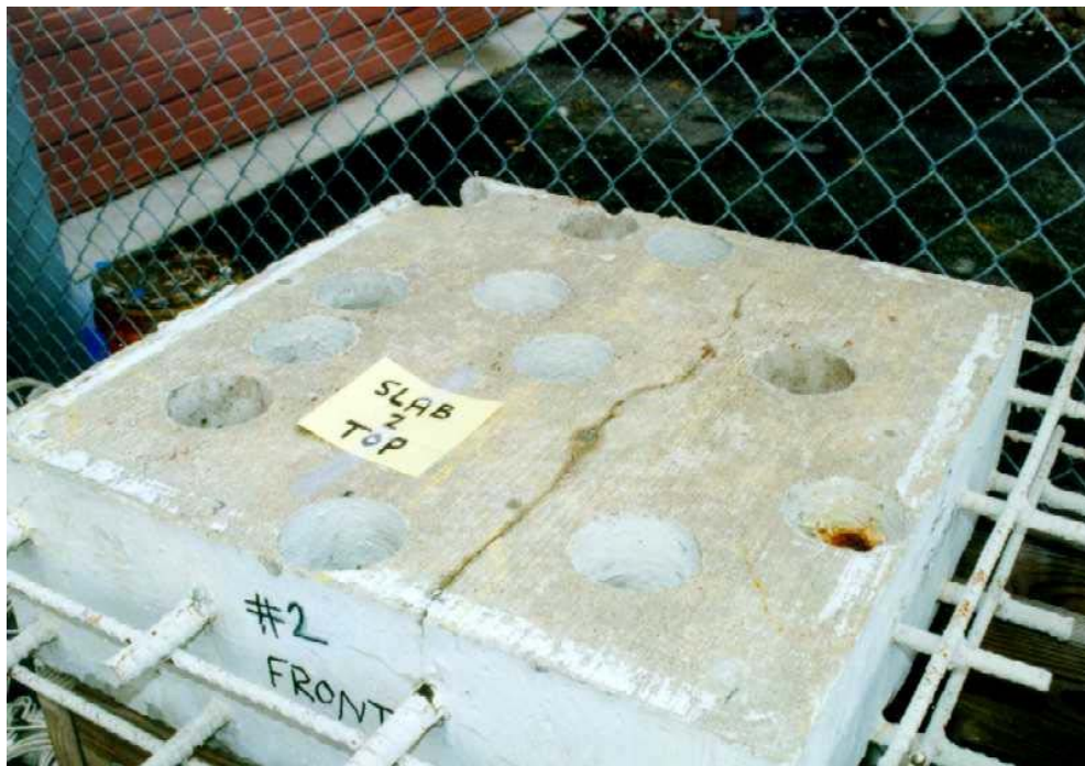
Figure 8. Photo. Corrosion on the ends of rebars exposed in core holes of slab 2.
