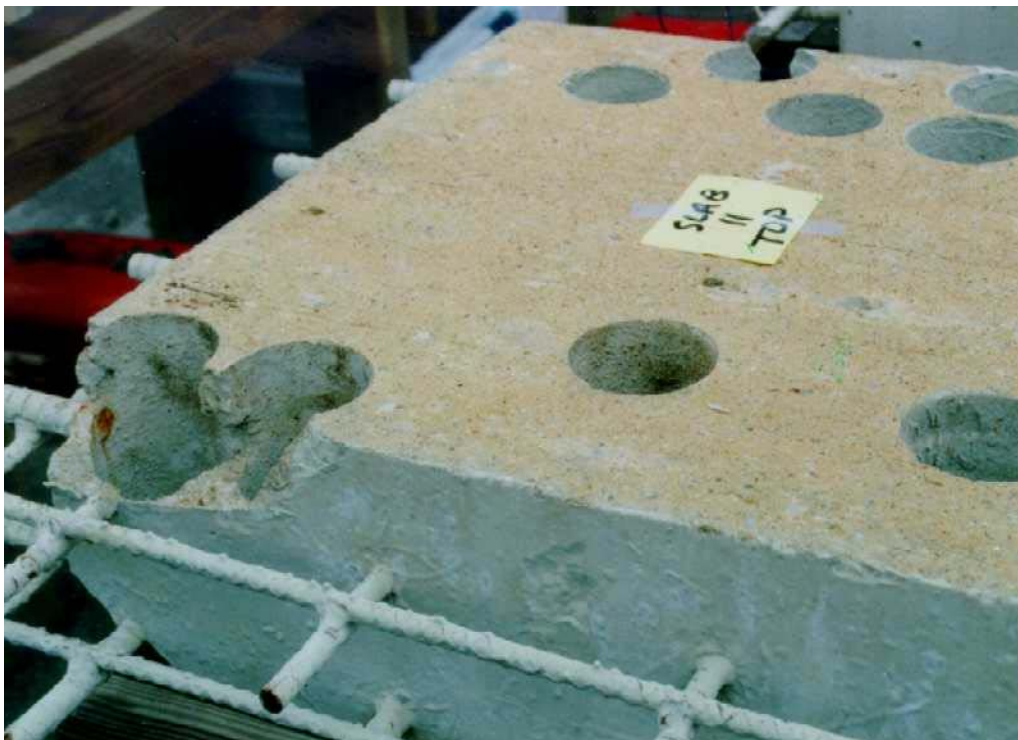
Figure 19. Photo. Noncorrosion-related concrete failure adjacent to core holes on one corner of slab 11 in spring 1997.
