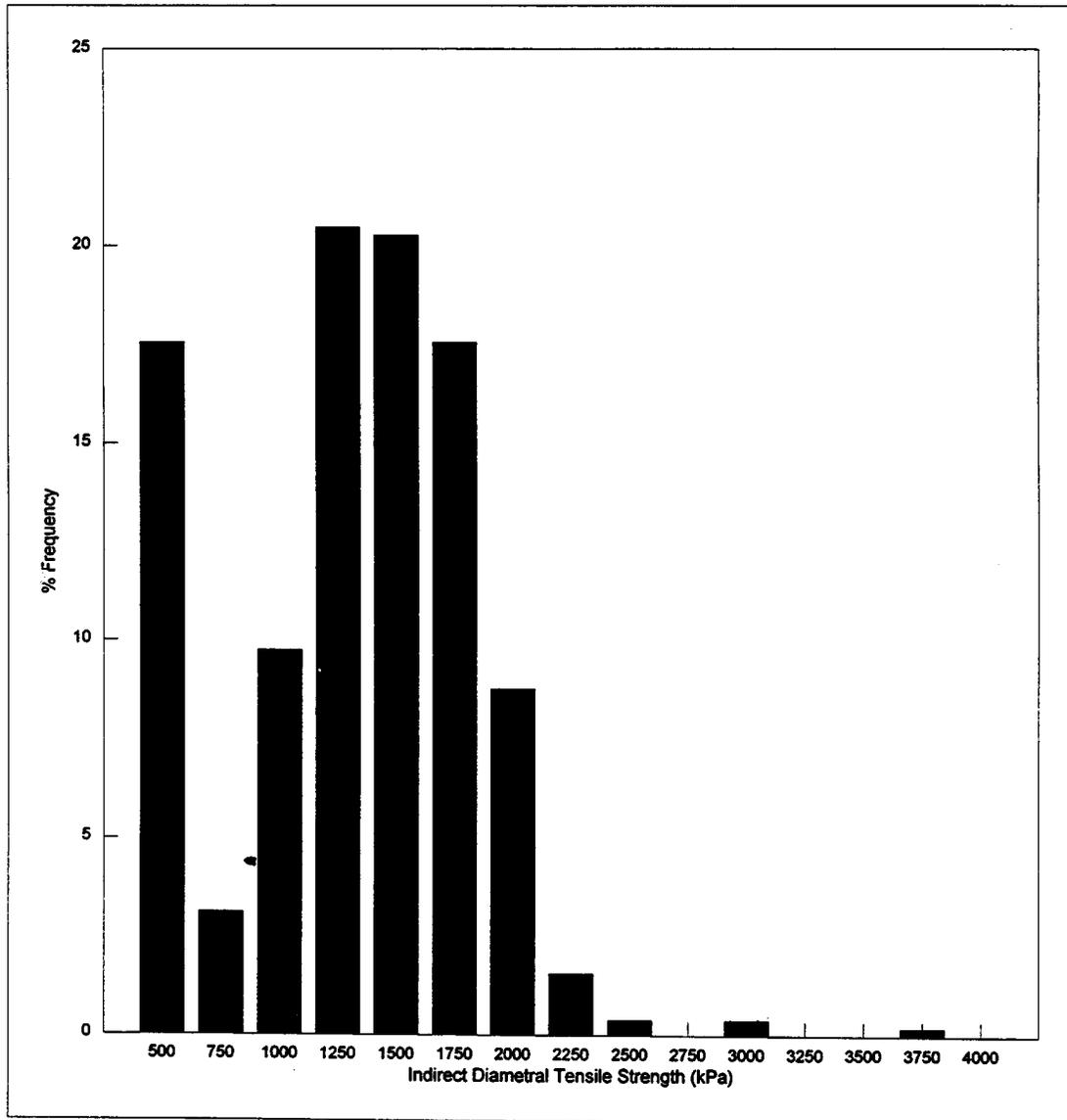
**Figure 4. Histogram of the indirect tensile strengths measured at 25 °C (77 °F) for dense-graded asphalt concrete mixtures recovered from the GPS sites.**
