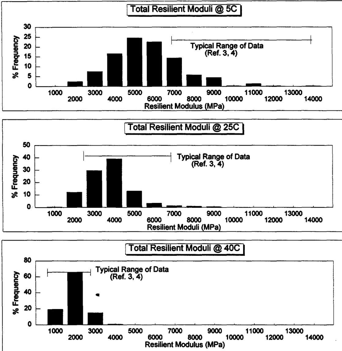
**Figure 6. Histogram of the total resilient modulus of asphalt concrete materials measured at the three test temperatures.**
