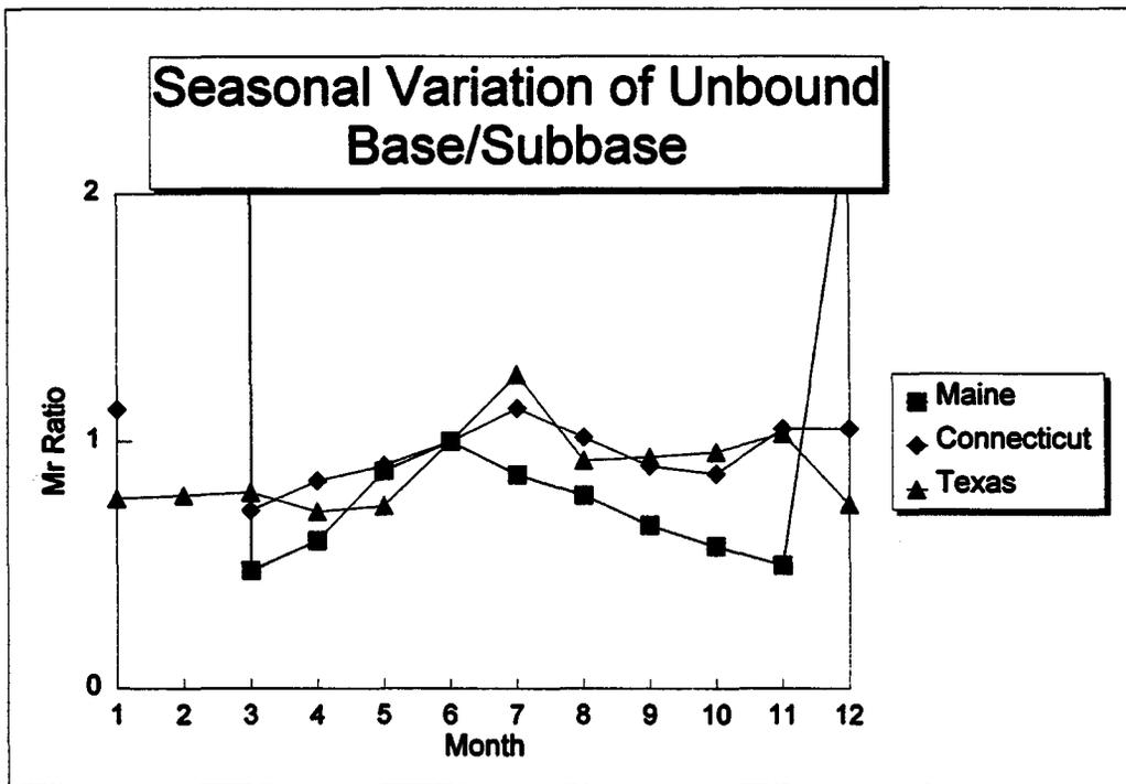
**Figure 56. Seasonal variation of the normalized backcalculated layer moduli for unbound granular base/subbase materials at three of the seasonal sites.**
