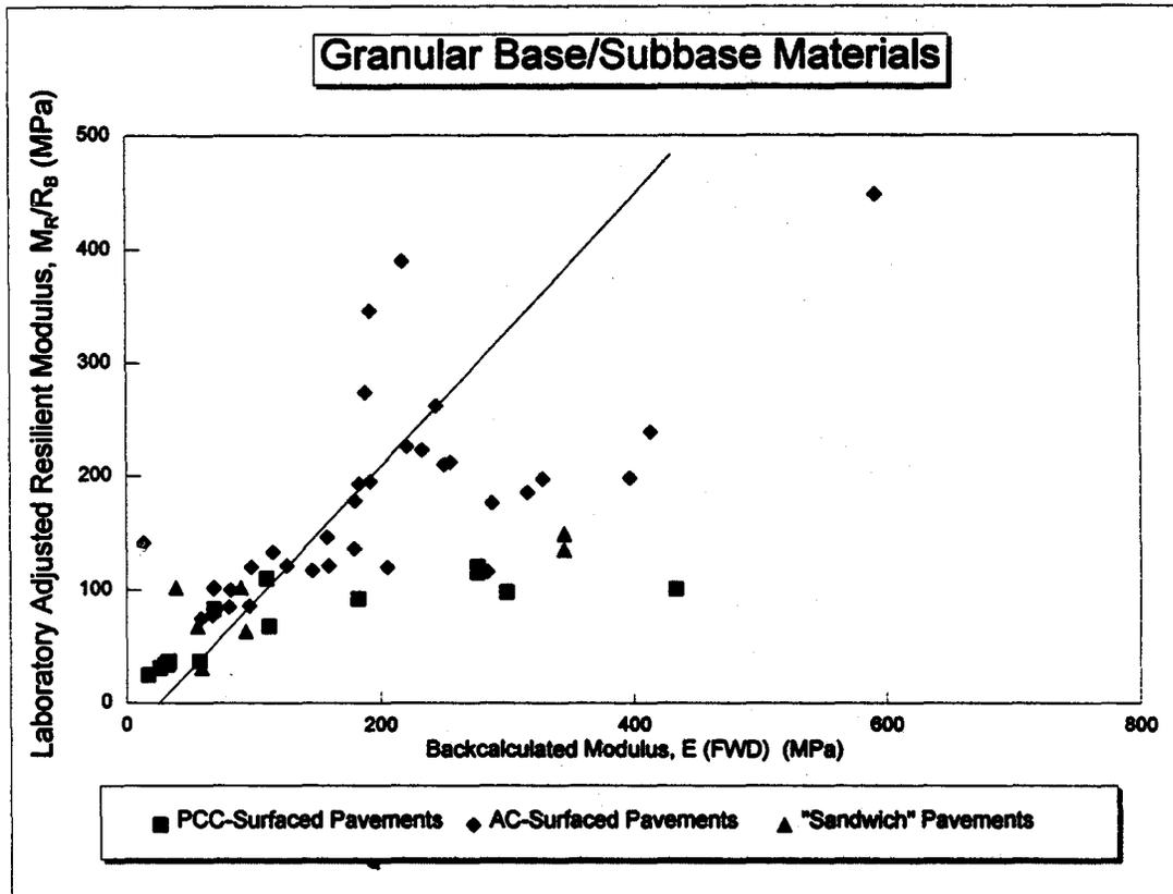
**Figure 30. Graphical comparison of backcalculated and laboratory measured moduli for the base and subbase layers.**
