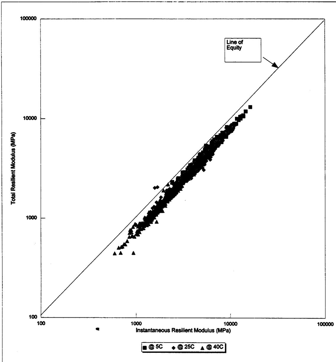
**Figure 3. Comparison of total and instantaneous resilient modulus for dense-graded asphalt concrete materials recovered and tested from the GPS sites.**
