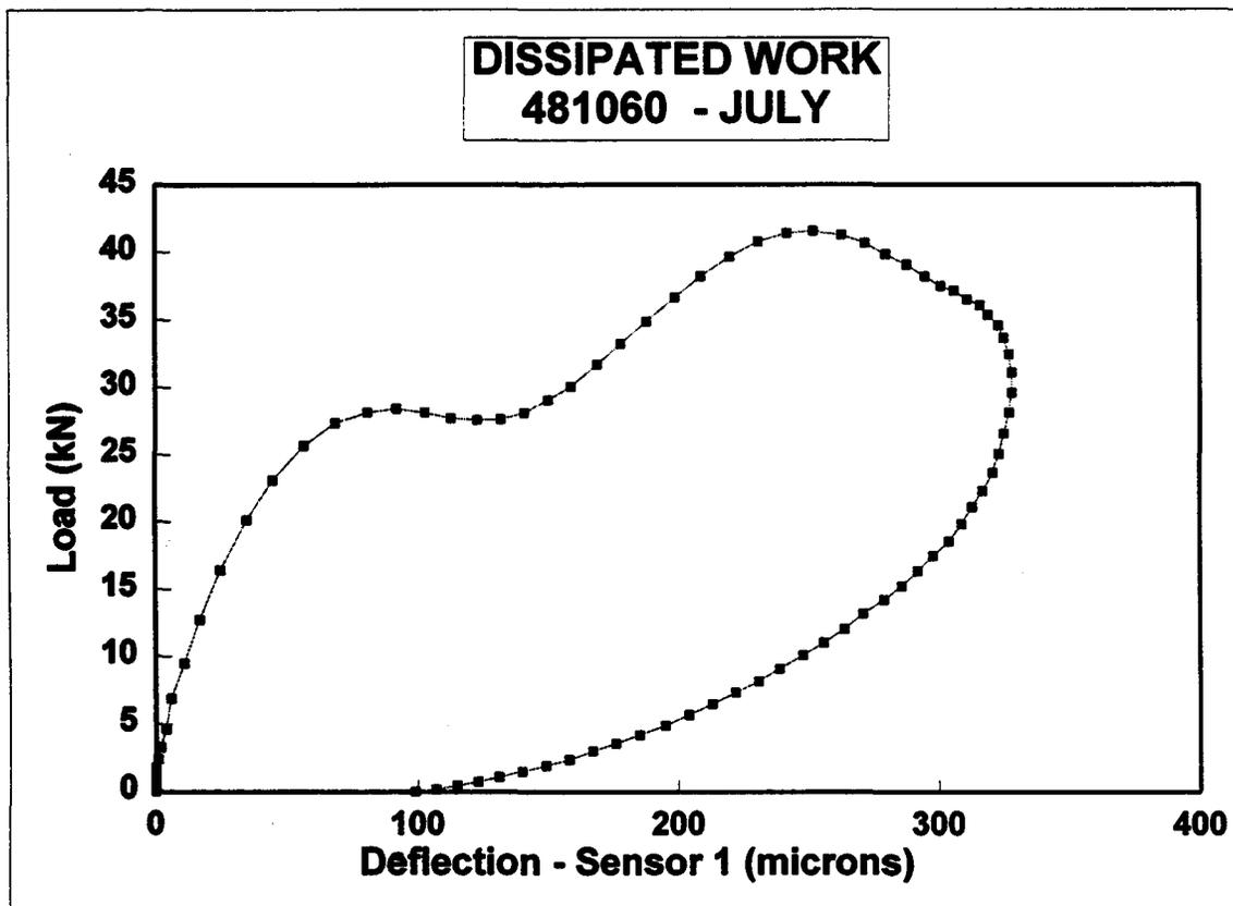
**Figure 71. Hysteresis loop as measured by the FWD at GPS site 481060 (asphalt concrete-surfaced pavement) in July.**
