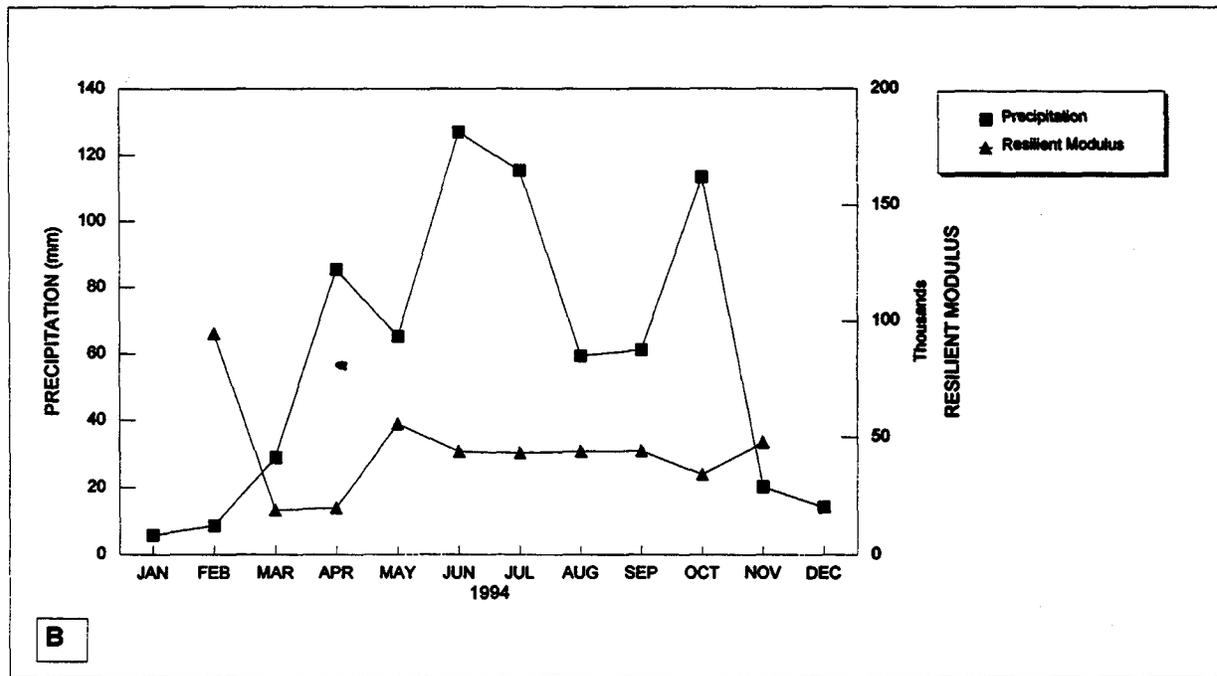
**Figure 41. Minnesota seasonal site measurements in the granular base, including backcalculated resilient modulus from 1994.**
