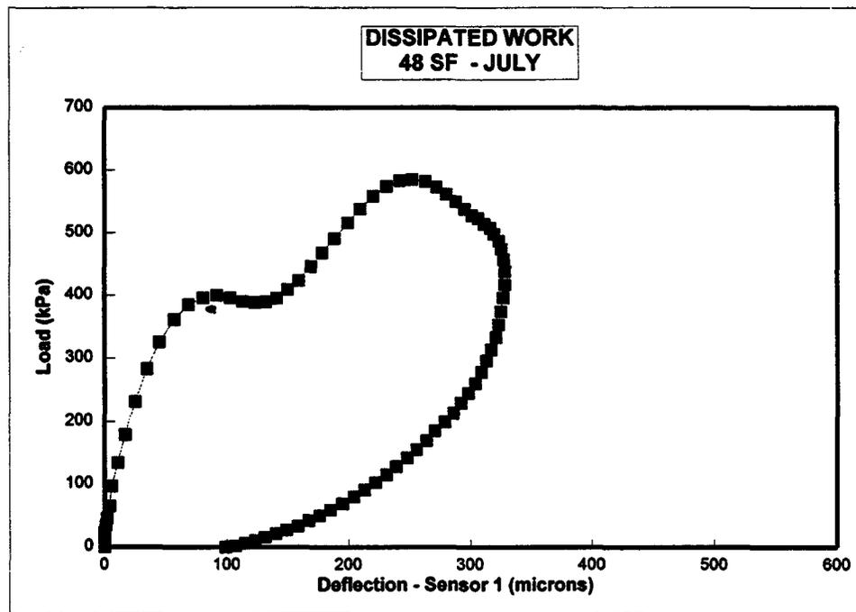
**Figure 34. Typical deflection-time history data collected during FWD testing and the associated dissipated work for a GPS site that has viscoelastic and plastic behavior.**
