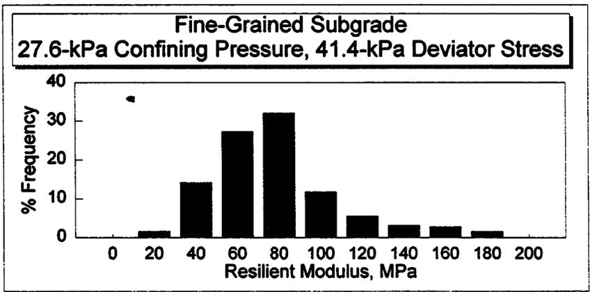
**Figure 13. Histogram of resilient modulus at specific stress states for unbound coarse- and fine-grained soils.**
