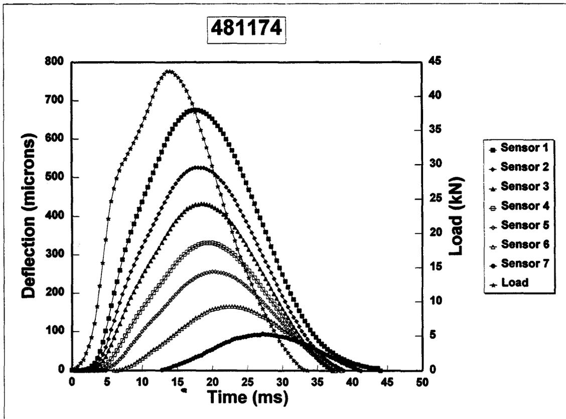
**Figure 61. FWD load pulse type "A" and the deflections measured by each sensor at GPS site 481174.**
