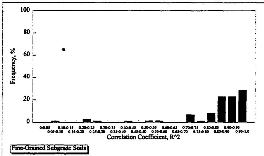
**Figure 14. Histogram of the R<sup>2</sup> term using equation 5 to fit the laboratory repeated-load resilient modulus test data for unbound materials and soils.**
