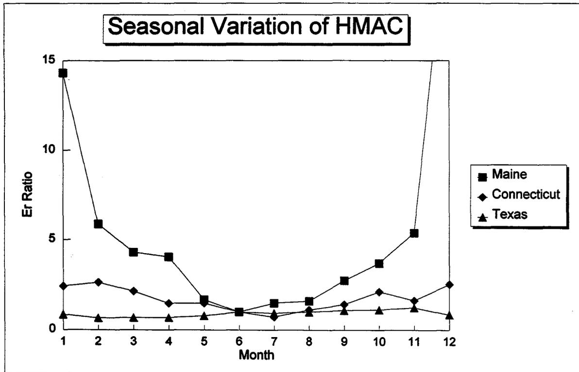
**Figure 55. Seasonal variation of the normalized backcalculated layer moduli for asphalt concrete mixtures at three of the seasonal sites.**
