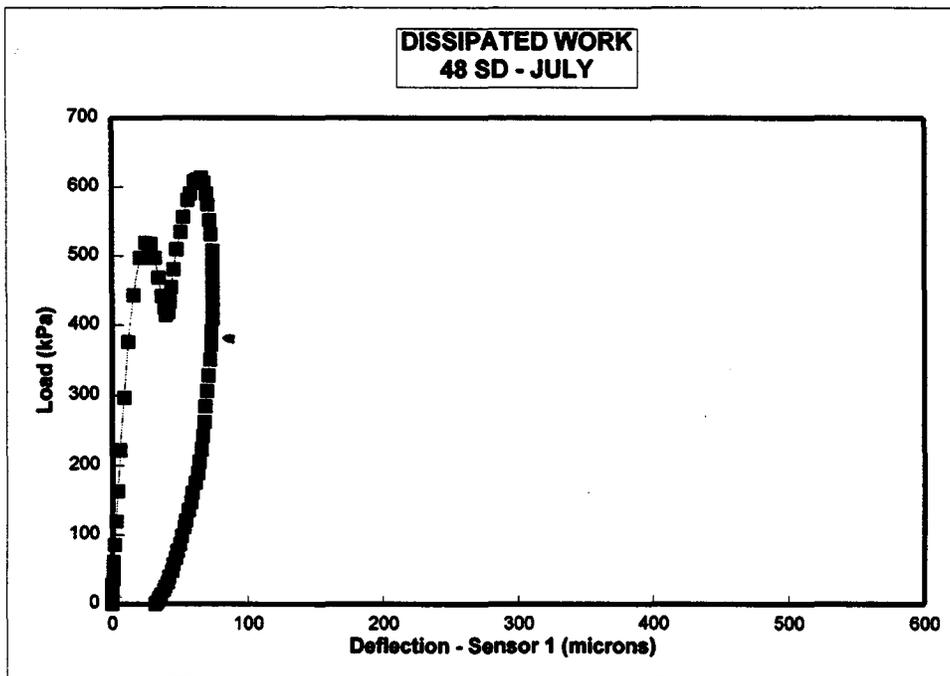
**Figure 33. Typical deflection-time history data collected during FWD testing and the associated dissipated work for a GPS site that has viscoelastic behavior.**
