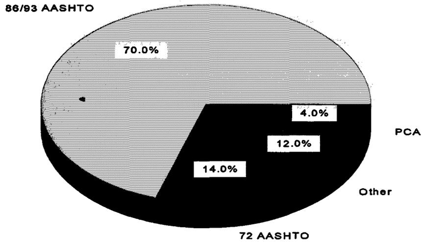
**Figure 1. Design procedures used on a routine basis by State Highway Agencies across the United States (2).**
