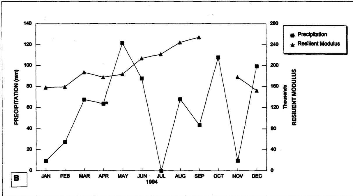
**Figure 44. Texas seasonal site measurements in the granular base, including backcalculated resilient modulus from 1994.**
