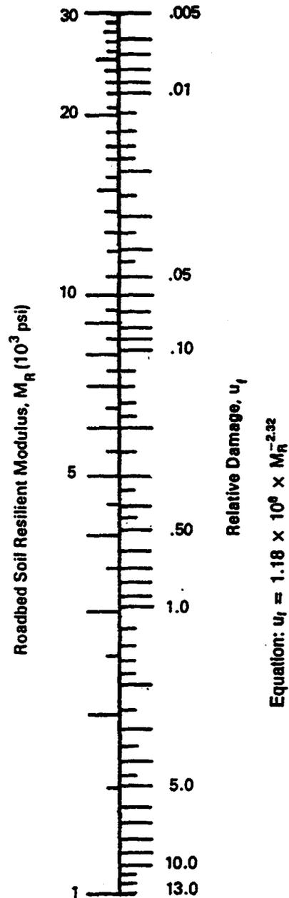
Figure 45. Chart for estimating effective roadbed soil resilient modulus for flexible pavements designed using the serviceability criteria (1).
