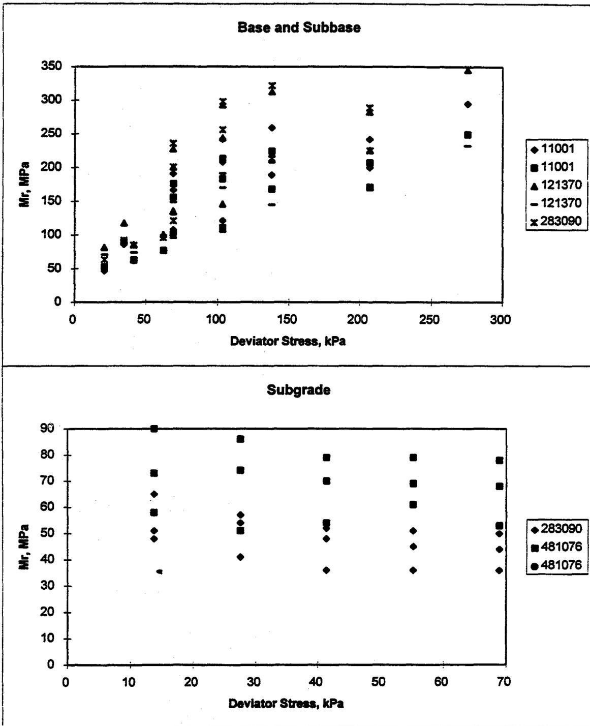
**Figure 12. Results from repeated-load triaxial resilient modulus tests performed on unbound base materials and subgrade soils.**
