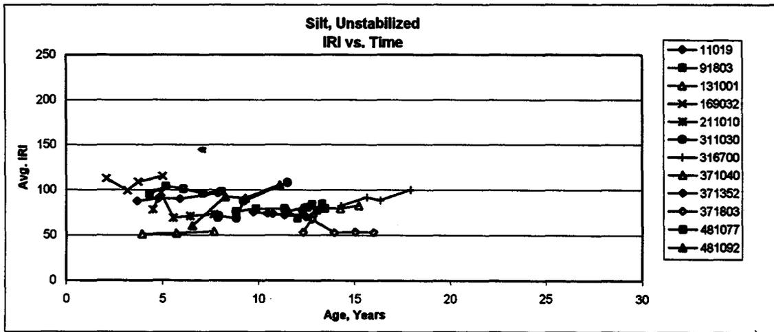
**Figure 47. Example of IRI versus time for GPS sites with silt subgrades.**
