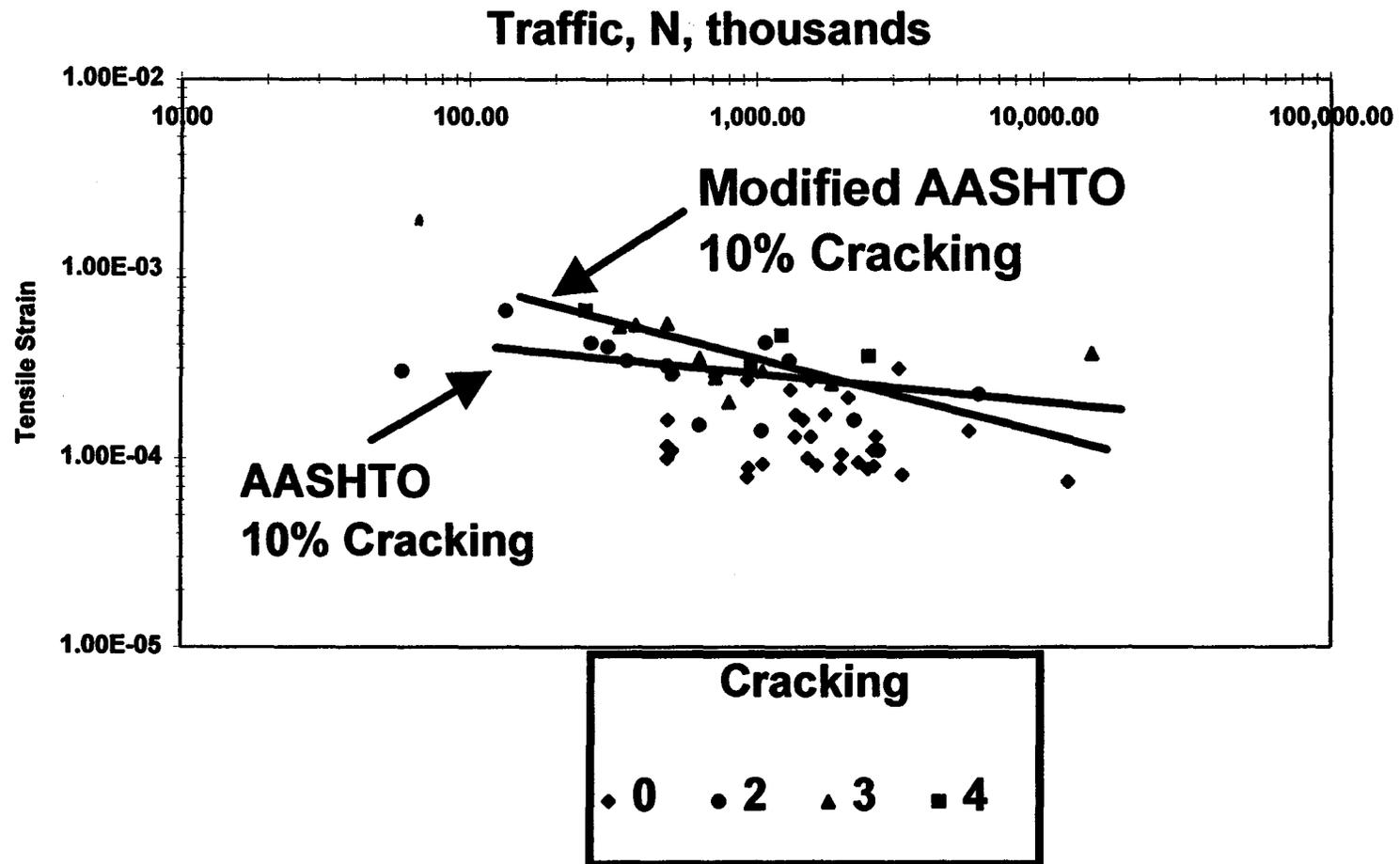
**Figure 58. Relationship between asphalt concrete tensile strains calculated with elastic layer theory of the total number of 80-kN (18-kip) ESAL's.**
