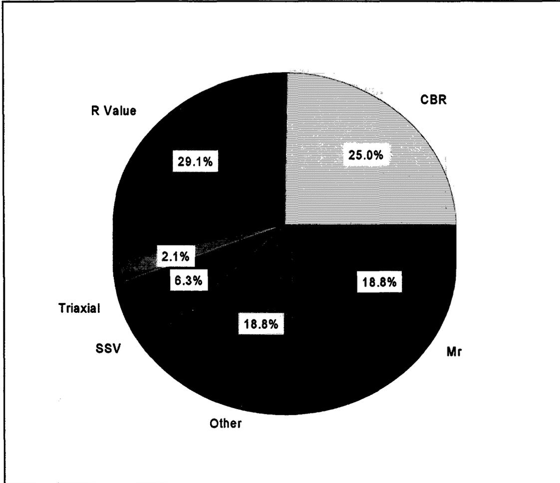
**Figure 2. Subgrade parameters used for flexible pavement designs across the United States (2).**
