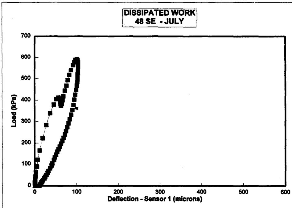
**Figure 32. Typical deflection-time history data collected during FWD testing and the associated dissipated work for a GPS site that has elastic behavior.**
