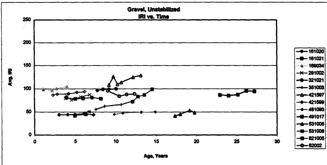
**Figure 49. Example of IRI versus time for GPS sites with gravel subgrades.**
