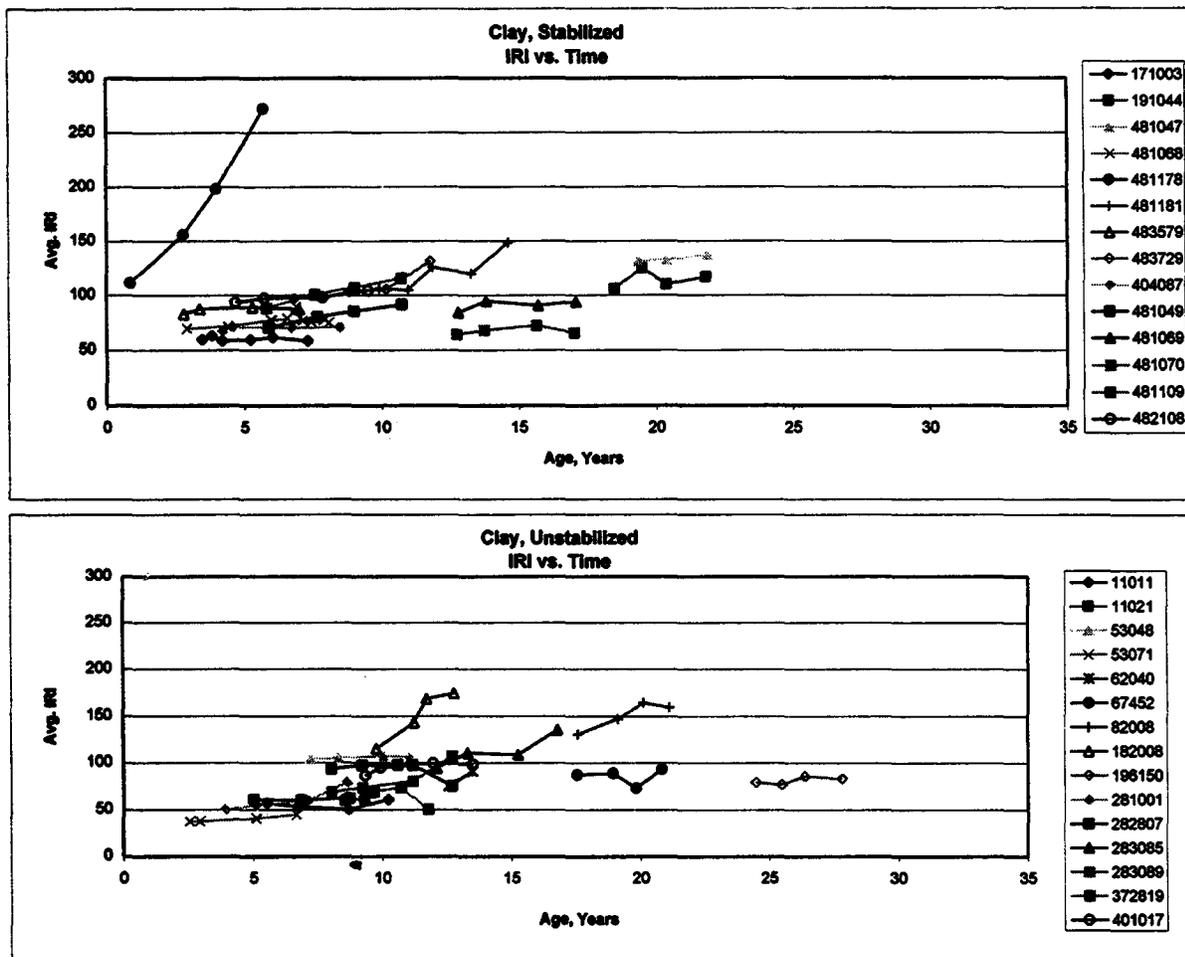
**Figure 46. Example of IRI versus time for GPS sites with clay subgrades.**
