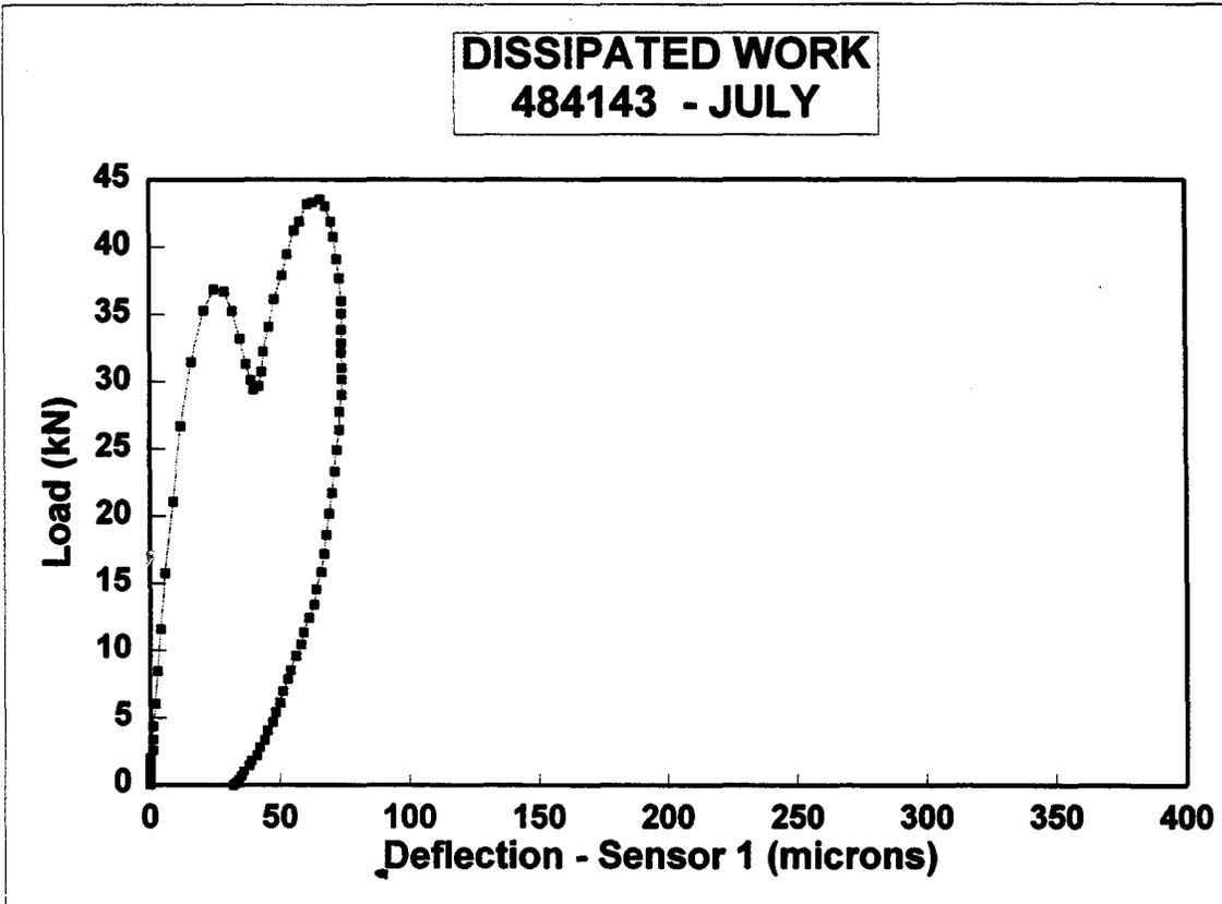
**Figure 70. Hysteresis loop as measured by the FWD at GPS site 484143 (PCC-surfaced pavement) in July.**
