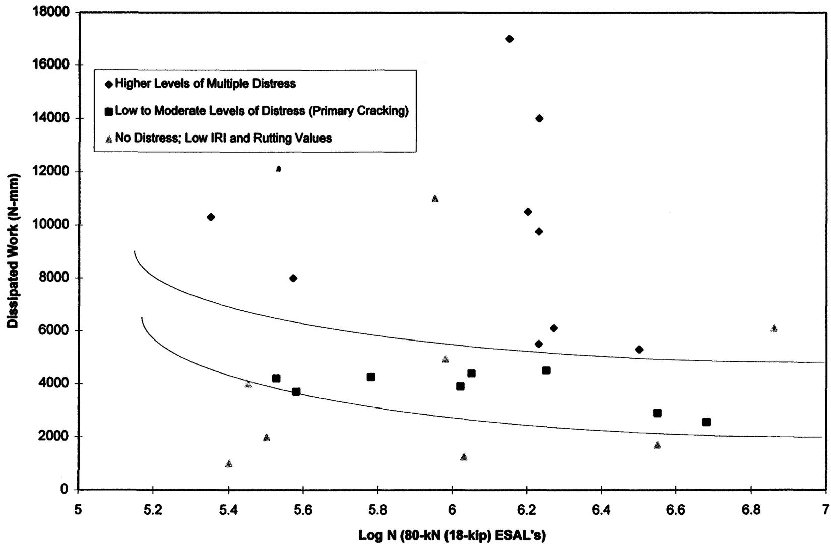
**Figure 73. Comparison of dissipated work to pavement condition for different traffic levels for selected GPS sites in the southern region.**
