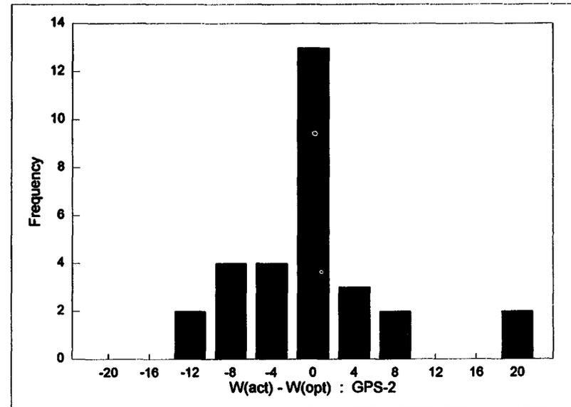
**Figure 38. Comparison of difference between optimum and actual moisture contents for subgrade soils in GPS-1 and GPS-2 sections with positive drainage systems.**
