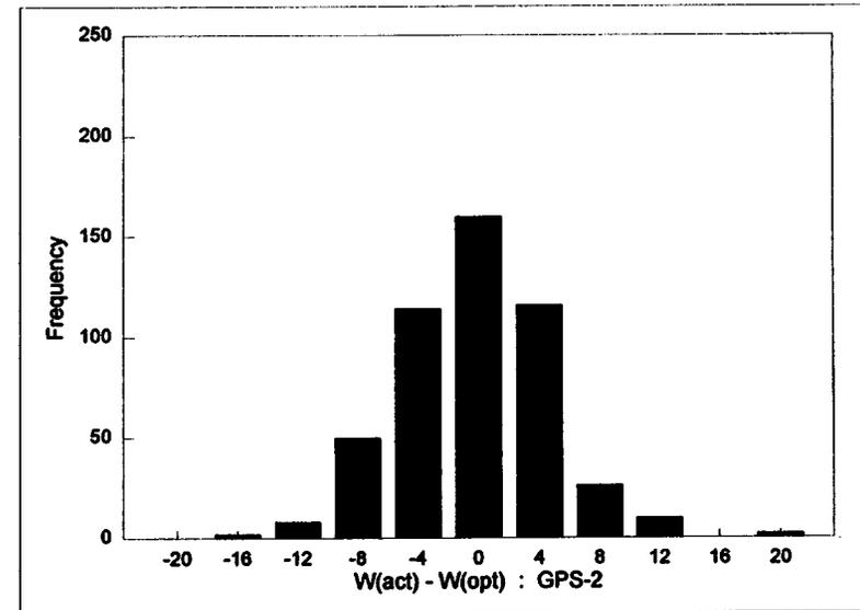
**Figure 37. Comparison of difference between optimum and actual moisture contents for subgrade soils in GPS-1 and GPS-2 sections with no positive drainage system.**
