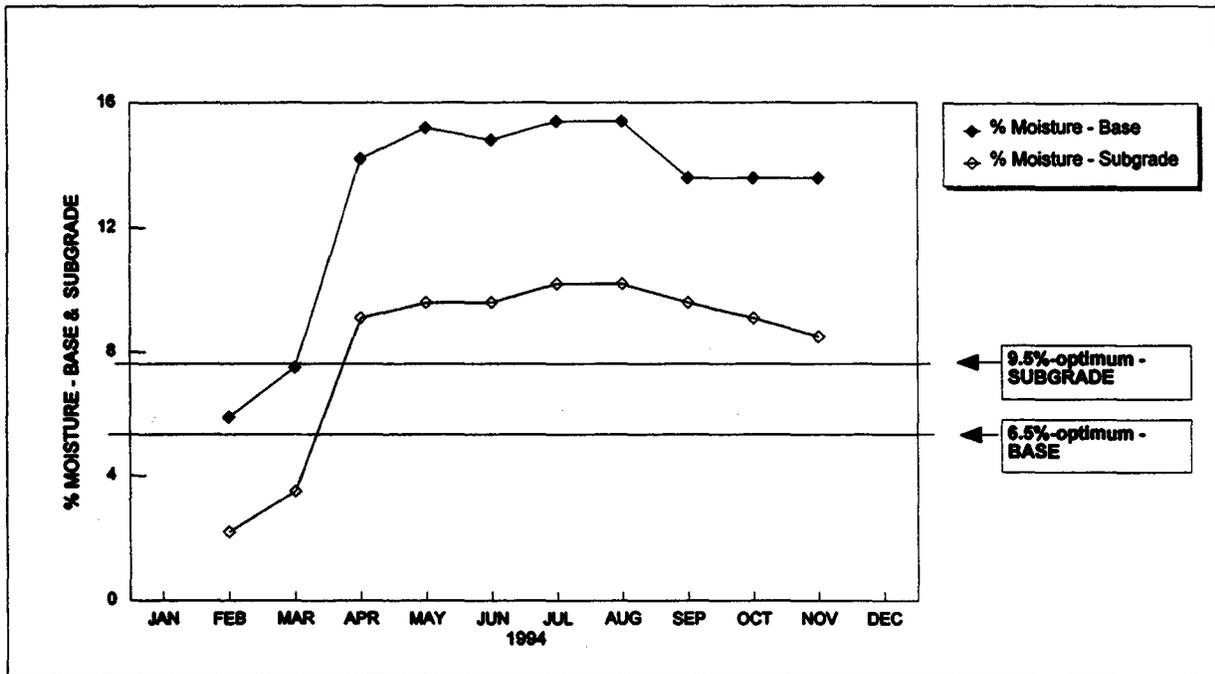
**Figure 40. Minnesota seasonal site measurements for base and subgrade moisture contents from 1994.**
