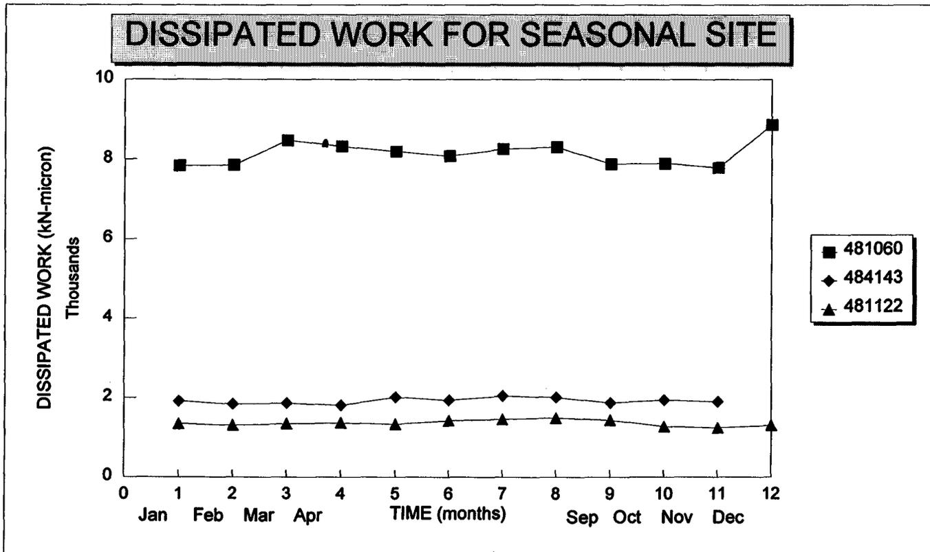
**Figure 72. Dissipated work by month, as measured during FWD deflection testing at three seasonal sites in the southern region.**
