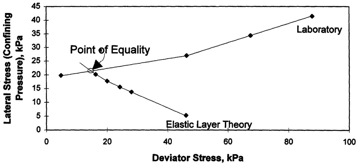
**Figure 28. Graphical illustration for procedure used to determine the stress states to be used in the laboratory so that the measured and backcalculated moduli are equal.**
