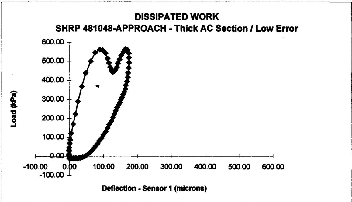
**Figure 53. Examples of the dissipated work determined from the deflection-time histories recorded during deflection testing on a pavement without a stabilized subgrade layer as compared to a pavement with a stabilized subgrade.**
