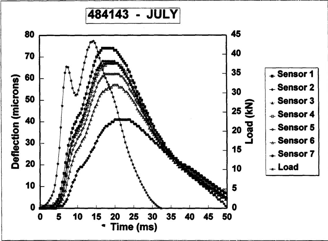
**Figure 68. Typical FWD deflection-time data from testing performed on a PCC pavement with viscoelastic behavior, GPS site 484143.**
