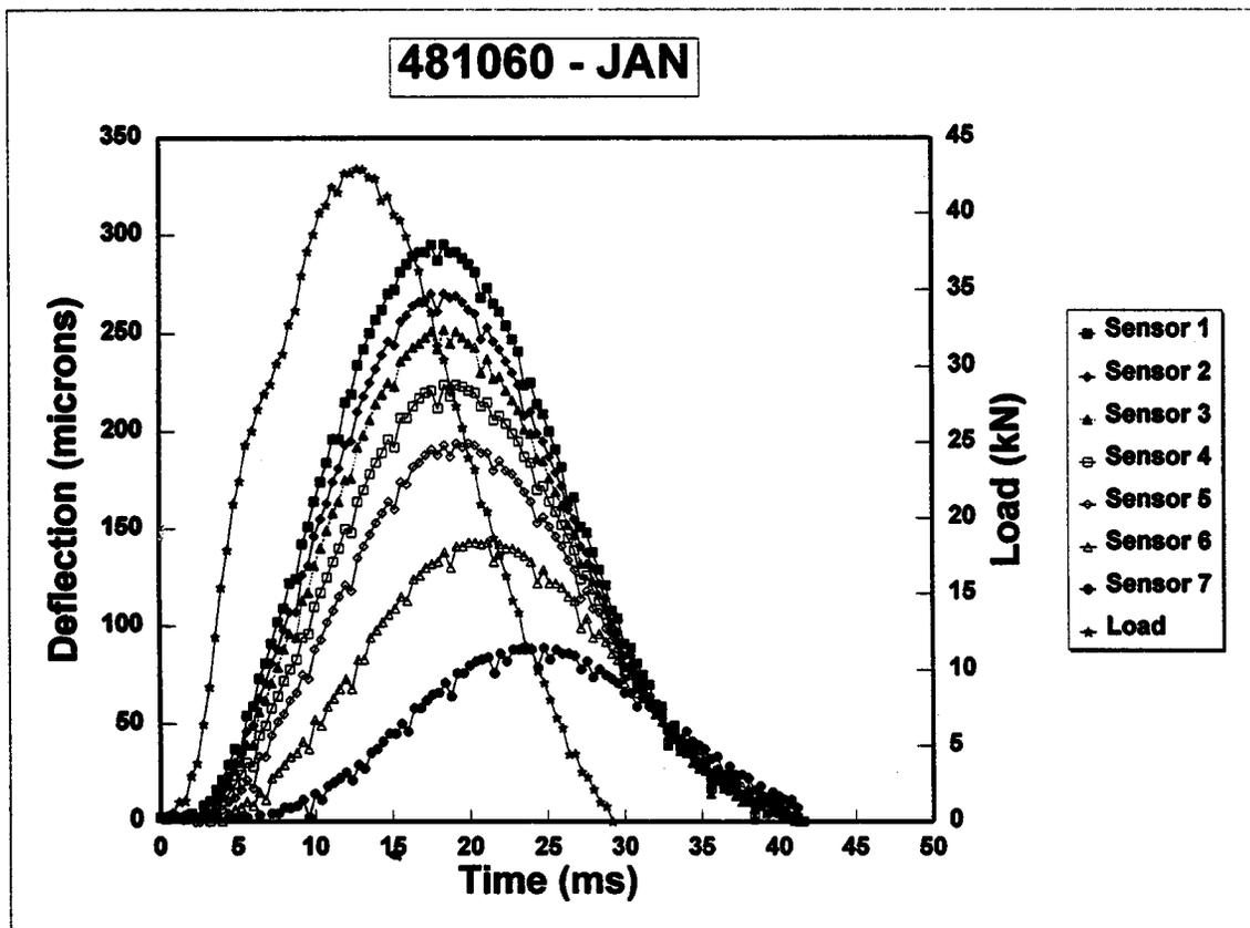
**Figure 67. Typical FWD deflection-time data from testing performed on an asphalt concrete pavement with some viscoelastic behavior, GPS site 481060.**
