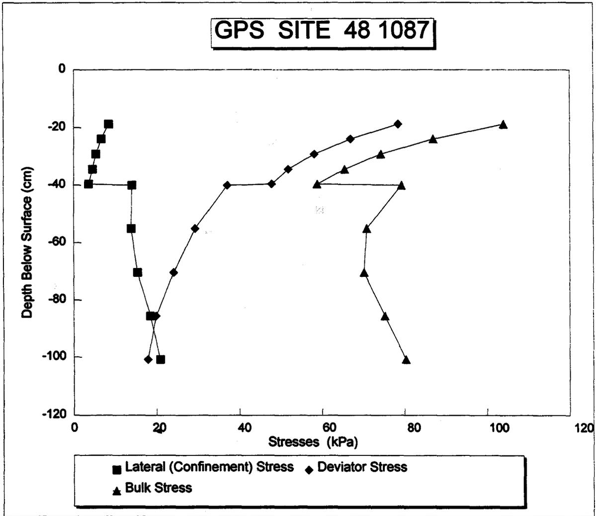
**Figure 29. Graphical illustration of the vertical profile of stresses in a layer for equating laboratory measured to backcalculated moduli.**
