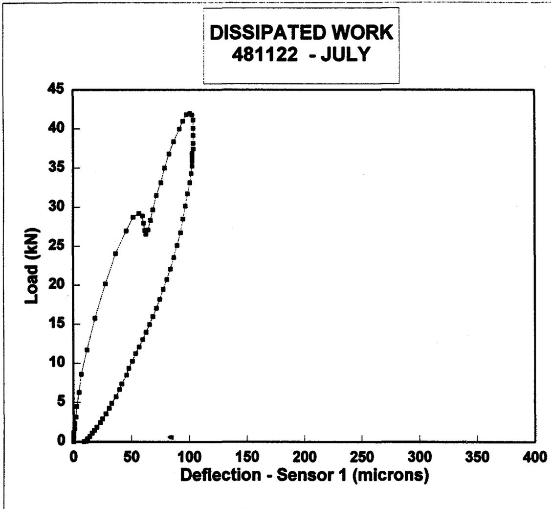
**Figure 69. Hysteresis loop as measured by the FWD at GPS site 481122 (asphalt concrete-surfaced pavement) in July.**
