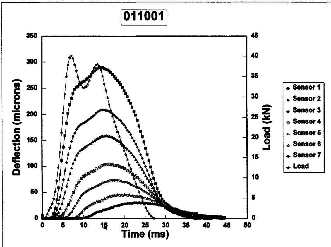
**Figure 64. FWD load pulse type "D" and the deflections measured by each sensor at GPS site 011001.**
