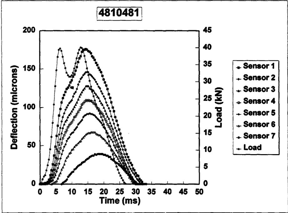
Figure 63. FWD load pulse type "C" and the deflections measured by each sensor at GPS site 4810481.
