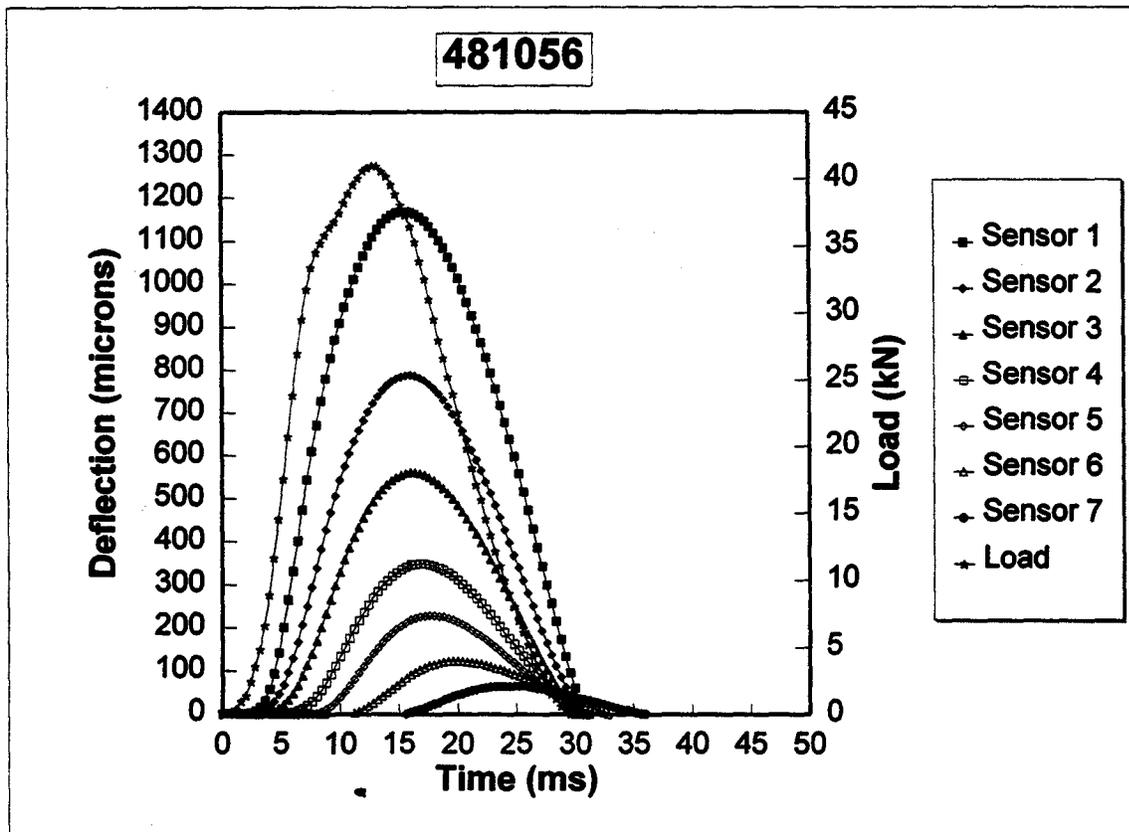
**Figure 66. Typical FWD deflection-time data from testing performed on an asphalt concrete pavement with elastic behavior, GPS site 481056.**
