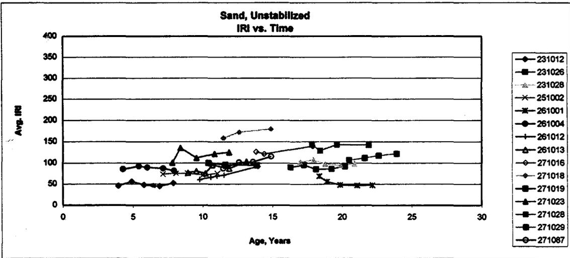
**Figure 48. Example of IRI versus time for GPS sites with sand subgrades.**
