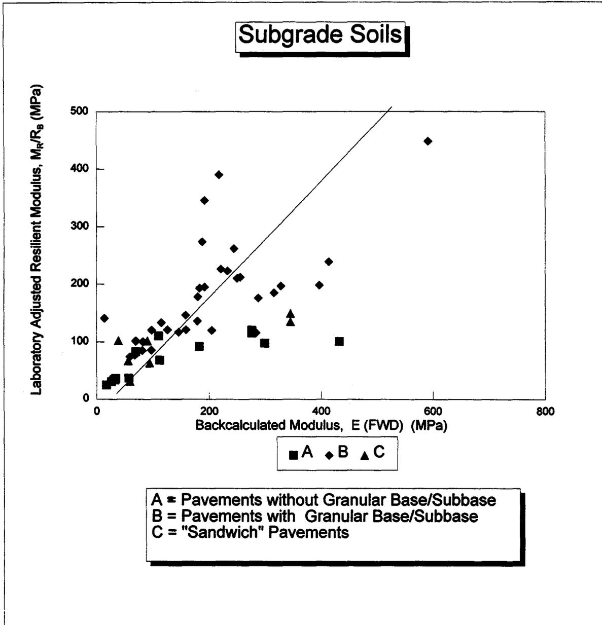
**Figure 31. Graphical comparison of backcalculated and laboratory measured moduli for subgrade soils.**
