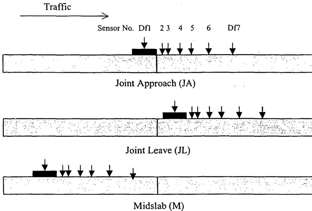
Sensor spacing from center of load plate: 0, 8, 12, 18, 24, 36 and 60 inches
