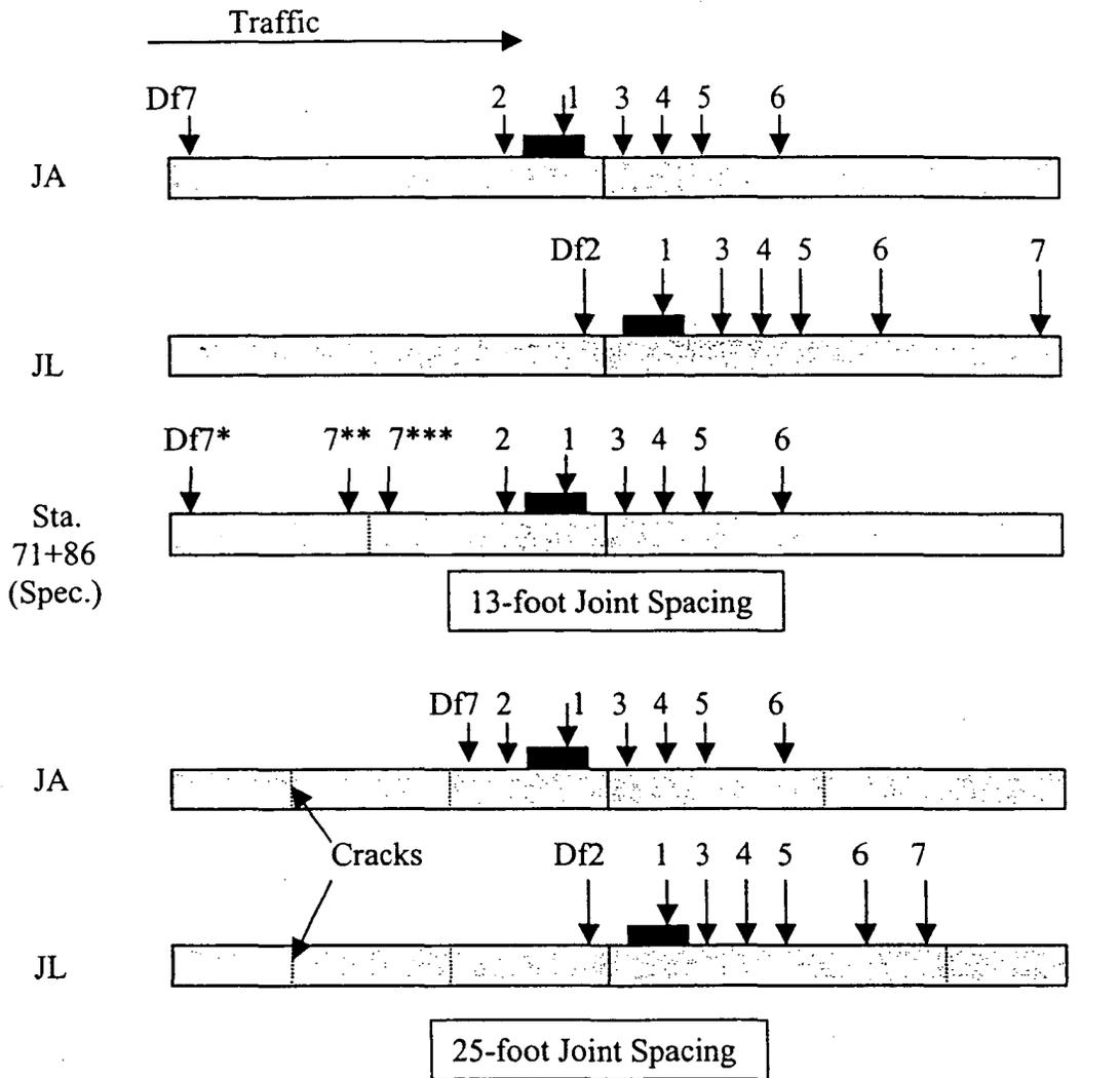
Sensor spacing from center of load plate: -12, 0, 12, 18, 24 and 36 inches, with Df7 being placed just inside the nearest crack or joint on the loaded slab
